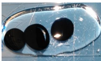
Figure 18. Cross-linked PEDOT:HAS 4 -PBA 0.3 -PEGene 0.22 ink film, swollen in water.
