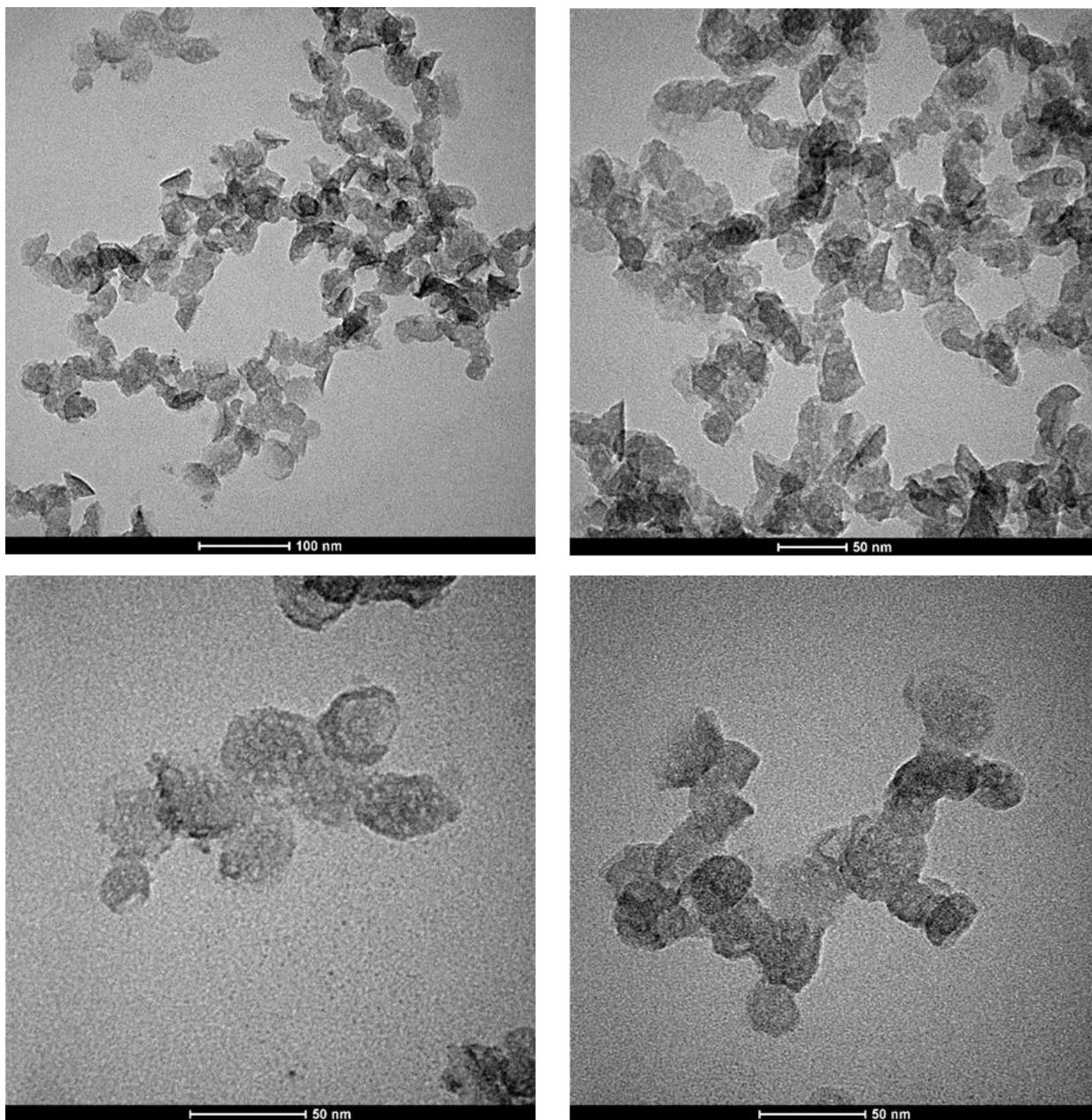
**Figure 3.24.** TEM images of 10% silica-coated Dodecyl silane QS after 5 days (reaction stopped by dialysis). Scale bar 100 and 50 nm.
