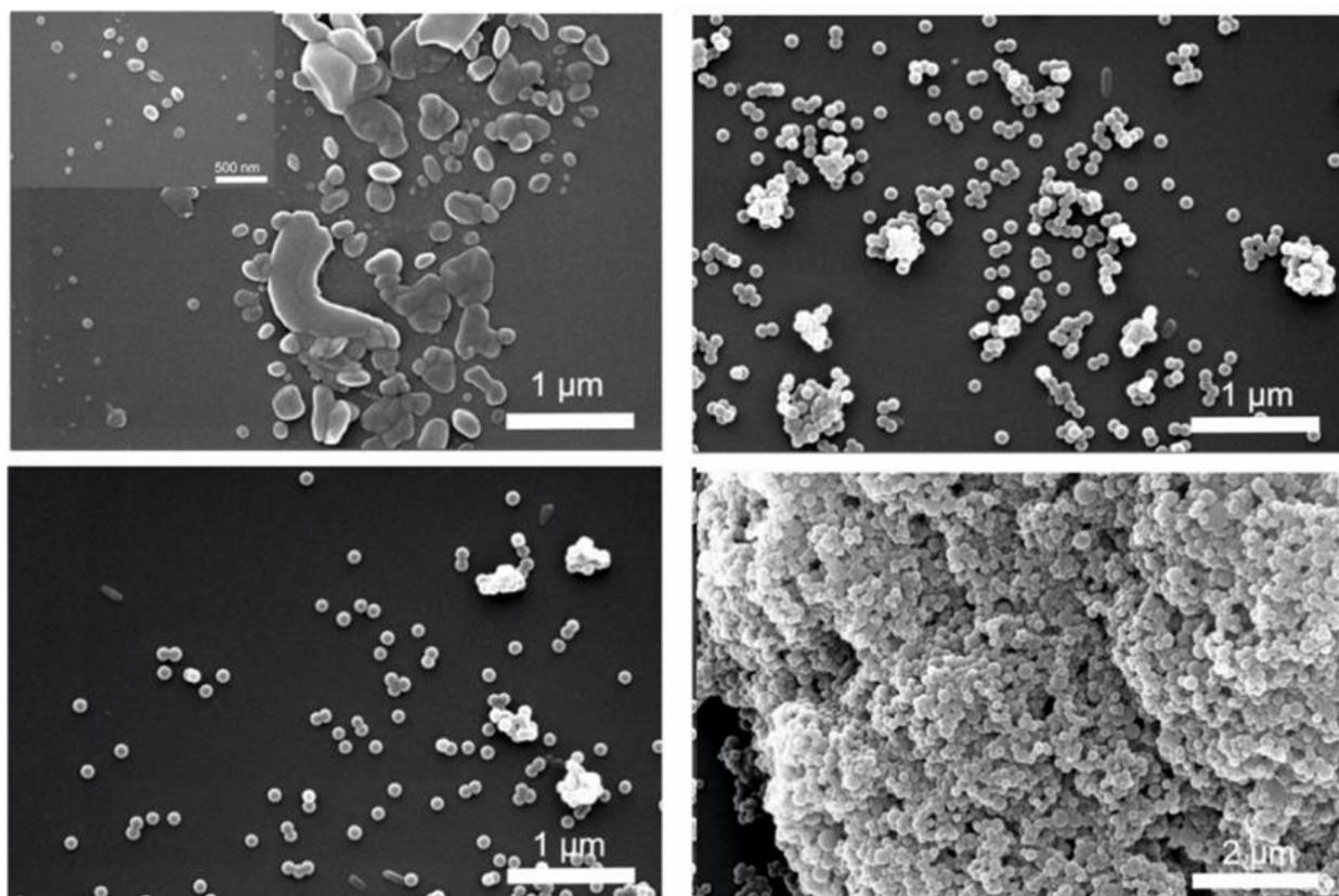
**Figure 3.8.** SEM pictures of the SQS after overnight of stirring (Scale bar of top left is  $1\ \mu\text{m}$  and inset is  $500\ \text{nm}$ , top right and down left are  $1\ \mu\text{m}$  and down right is  $2\ \mu\text{m}$ ).
