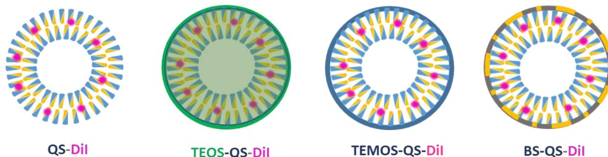
**Figure 4.19.** Labeled silica-coated QS used for the permeability test. From left to right: QS loaded with Dil, QS loaded with Dil and coated with TEOS (non-breakable shell), QS loaded with Dil and coated with TEMOS (non-breakable shell) and QS loaded with Dil and covered with BTSPD and APTES (breakable silica shell).
