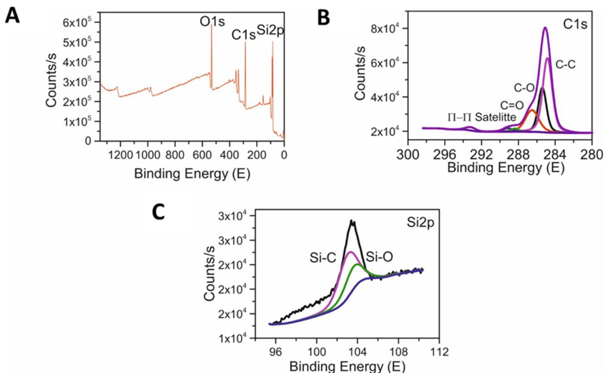
**Figure 3.26. A)** Representative X-Ray Photoelectron Spectroscopy (XPS) spectra analysis of the surfaces of 10% silica-coated Dodecyl silane QS after 5 days, **B)** Carbon analysis, deconvolution of the C<sub>1s</sub> core level spectra and **C)** Silicon analysis, deconvolution of the Si2p core level.
