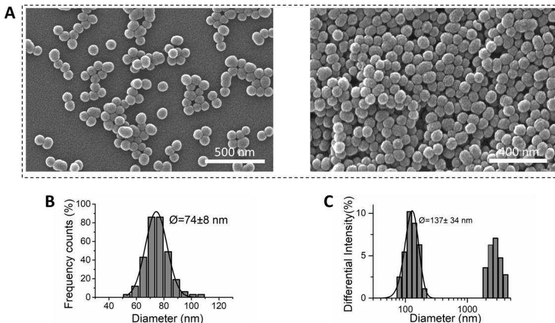
**Figure 5.24.** A) SEM pictures of Long Pore-Breakable NPs prepared with a non-toxic surfactant (MKC). B) SEM counting of 300 NPs (size distribution  $74 \pm 8$  nm) and C) DLS distribution  $137 \pm 34$  nm.
