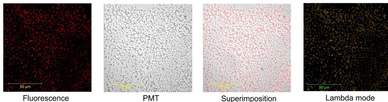
**Figure 2.26.** Confocal microscope images of the PLGA microspheres loaded with Nile Red using 63x objective.
