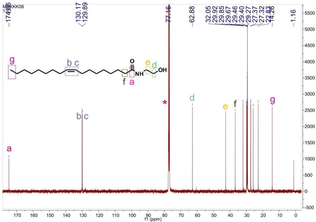
Figure 2.60. <sup>13</sup>C NMR spectrum of *N*-(2-hydroxy ethyl) oleamide.
