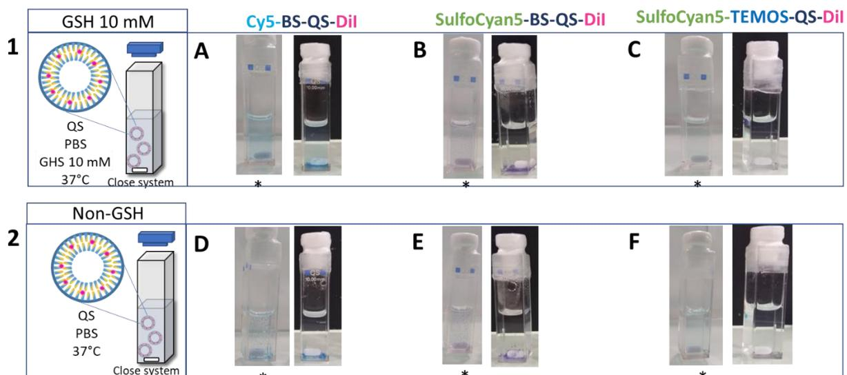
**Figure 4.32.** Pictures of the samples after 9 days for the Cy5-BS-QS-Dil, Sulfo-Cyan5-BS-QS-Dil, and Sulfo-Cyan5-TEMOS-QS-Dil in presence of GSH **A)**, **B)** and **C)**; and with non-GSH **D)**, **E)** and **F)**, respectively. \*Images were taken after shaking the samples.
