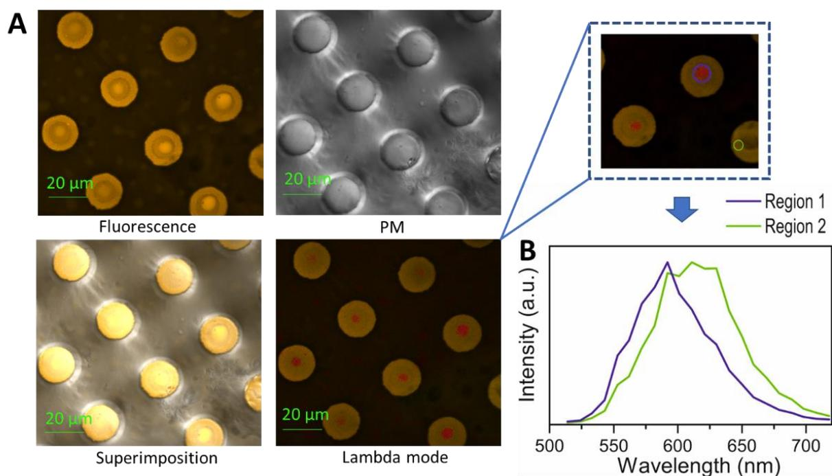
**Figure 2.37. A)** Confocal microscope images of 2HEO-PLGA@MBds loaded with Nile Red using 63x objective (scale bar 20 $\mu$ m). **B)** Emission spectra of the lambda mode of 2HEO taken from two different areas of the 2HEO-PLGA@MBds confocal images.
