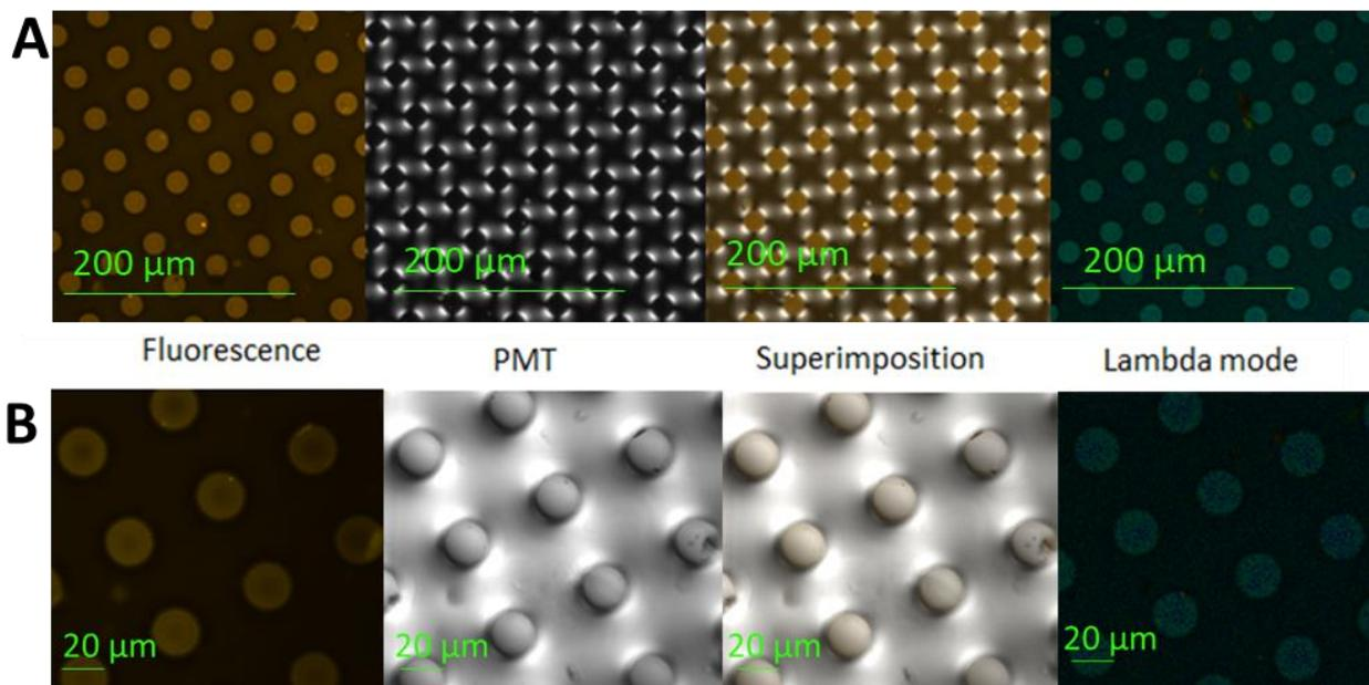
**Figure 2.45.** Confocal microscope images of the hydrogel filled by the polymer with NPs using **A)** 10x and **B)** 64x objective (scale bar 200 and 20 μm, respectively).
