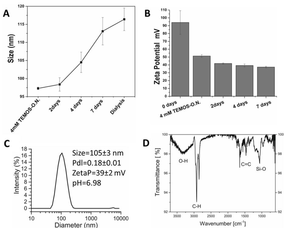
**Figure 3.28.** **A)** DLS size distribution measurement of the samples and **B)** Zeta Potential measurement of the reaction over time of TEMOS silica-coated QS at  $0^\circ \text{C}$  for 7 days. **C)** DLS-Size distribution measurement after 4 days of reaction the NB-QS-TEOS. **D)** IR spectra of silica-coated QS. The starting material has a size of  $84 \pm 1$  nm a Pdl of  $0.23 \pm 0.01$  and a Zeta Potential of  $84 \pm 2$  mV.
