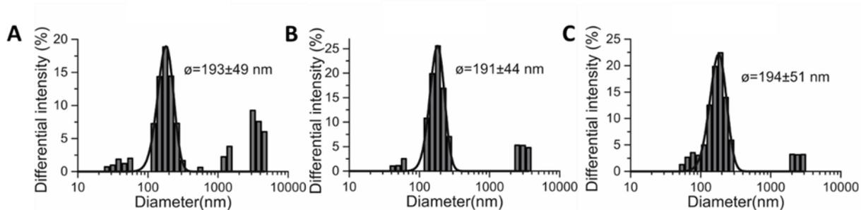
**Figure 3.7.** The DLS measurement of the SQS using APTES after **A)** 2h, **B)** overnight and **C)** 2 days of stirring.
