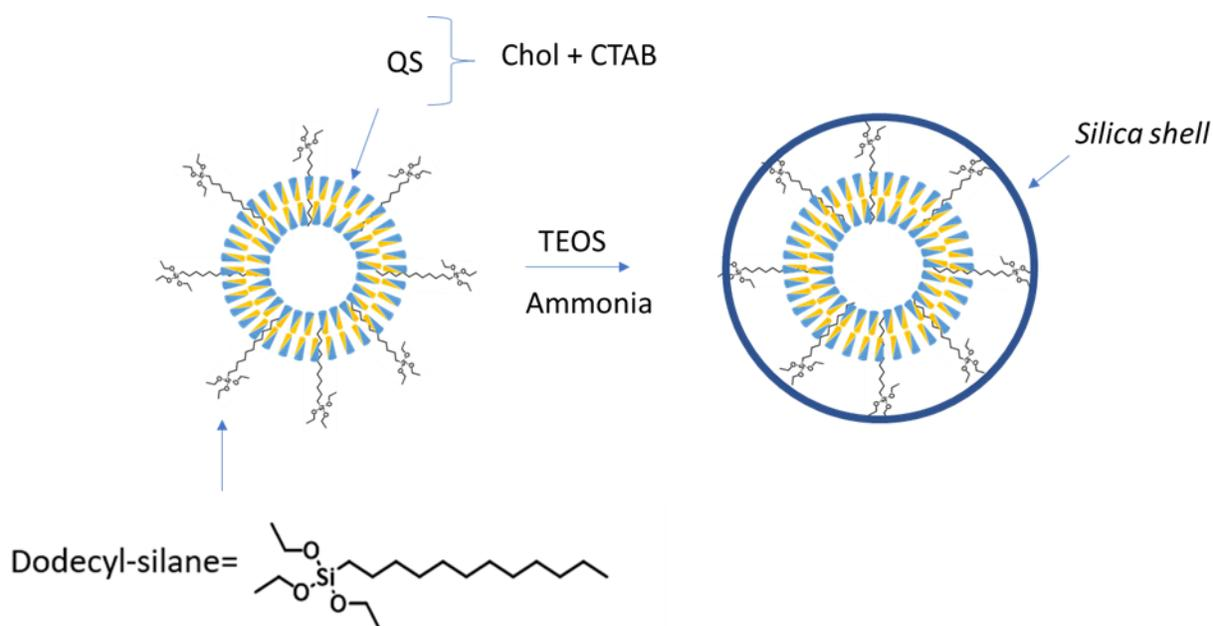
**Figure 3.20.** Representation of the Dodecyl-silane QS covered with a shell of silica form.
