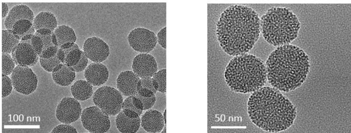
Figure 5.19. TEM images of the Breakable NPs done with MKC (Scale bar 100 and 50 nm).
