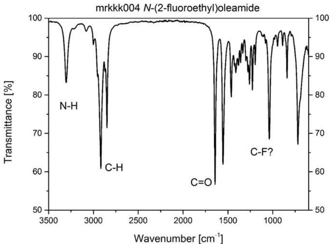
Figure 2.55. IR spectrum of *N*-(2-fluoroethyl)oleamide.
