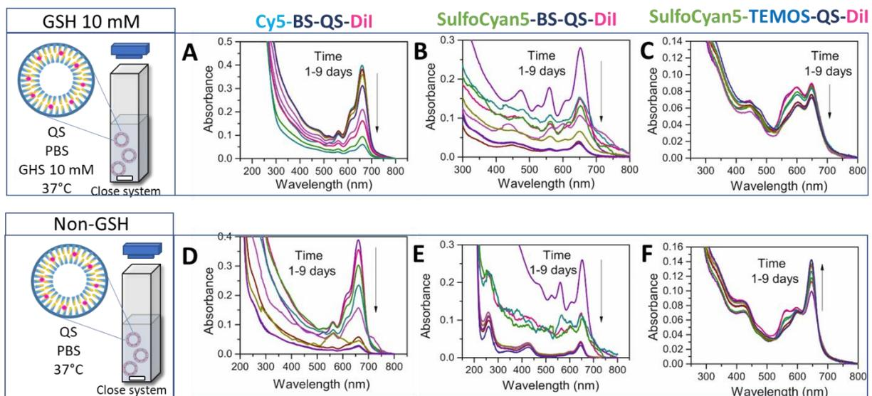
**Figure 4.30.** Absorbance of the sample during 9 days for the Cy5-BS-QS-Dil, Sulfo-Cyan5-BS-QS-Dil, and Sulfo-Cyan5-TEMOS-QS-Dil in presence of GSH **A)**, **B)** and **C)**; and with non-GSH **D)**, **E)** and **F)**, respectively.
