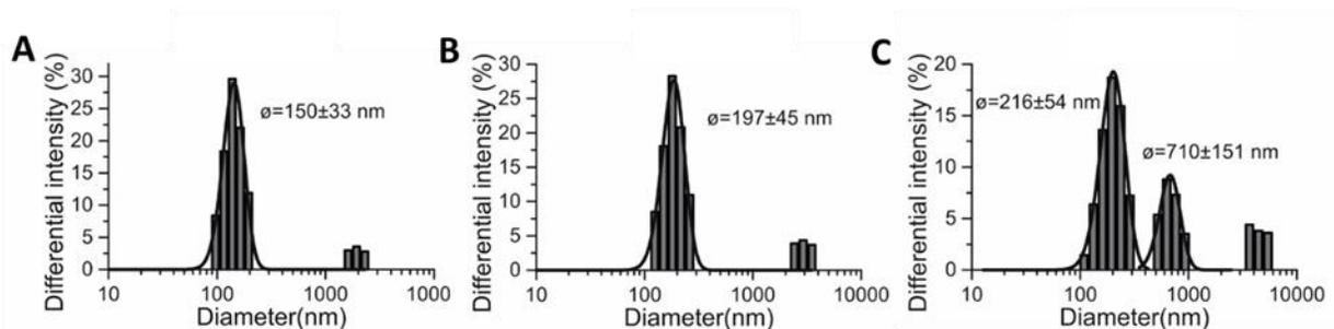
**Figure 3.3.** Size of the QS was measured by DLS at three different % of EtOH **A)** 20, **B)** 30 and **C)** 40 %.
