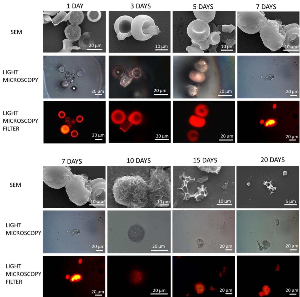
**Figure 2.51.** SEM, Light microscopy, and light microscopy using a filter of the degradation of the PLGA@MBds loaded with Nile Red in Acetates buffer media (pH 5.2) and 37 °C, followed during the time for 20 days.
