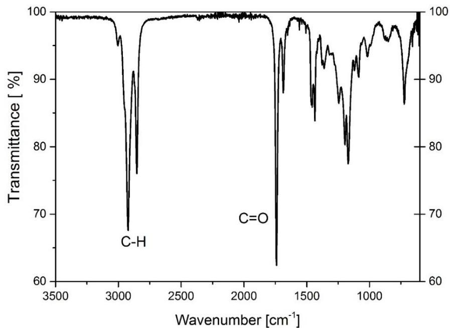
Figure 2.58. IR spectrum of methyl oleate.
