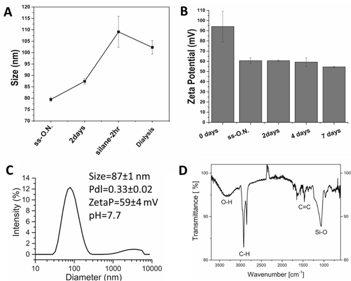
**Figure 3.38.** A) DLS-Size and B) Zeta Potential measurement of the reaction over time of for the breakable silica-coated QS at 0 °C for 2 days. C) DLS-Size distribution measurement after 2 days of reaction. D) IR spectra of silica-coated QS. The starting material has a size of  $84 \pm 1$  nm a Pdl of  $0.23 \pm 0.01$  and a Zeta Potential of  $84 \pm 2$  mV.
