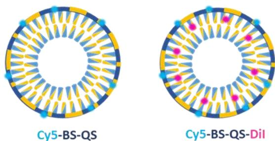
Figure 4.11. Schema of the labeled silica-coated QS used for the breakability test.
