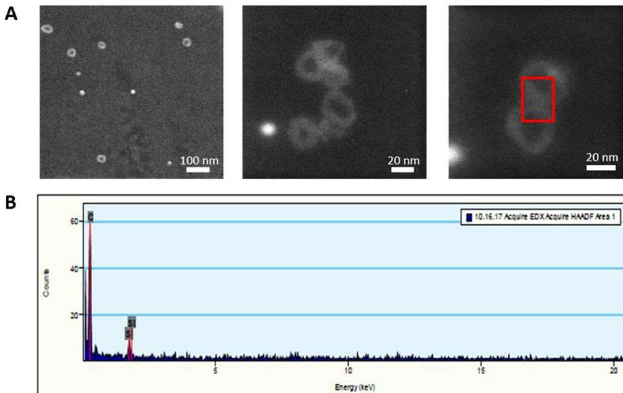
**Figure 3.36.** A) SEM image of breakable silica-coated QS. Scale bar 100, and 20 nm and B) EDX of the B-SQS sample.
