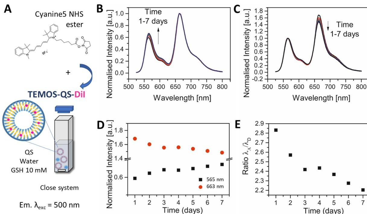
**Figure 4.23.** **A)** Experiment diagram for the permeability test using TEMOS-QS-Dil (non-breakable). **B)** and **C)** Normalised Intensity of the Emission of the TEMOS-QS-Dil; normalised by the Cyanine5 and the Dil band, respectively. **D)** Normalised intensity of the emission at 565 and 663 nm representing the Dil and the Cyanine5. **E)** Ratio Acceptor/Donor of the sample after 7 days.
