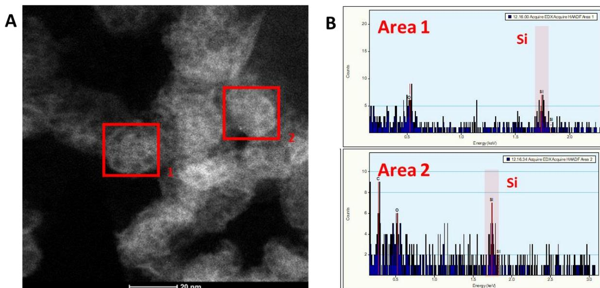
**Figure 3.25. A)** Cryo-STEM image of 10% silica-coated Dodecyl silane QS after 5 days (reaction stopped by dialysis). Scale bar 20 nm and **B)** EDX of the sample in two different areas (zone 1 and 2 of the Cryo-STEM image).
