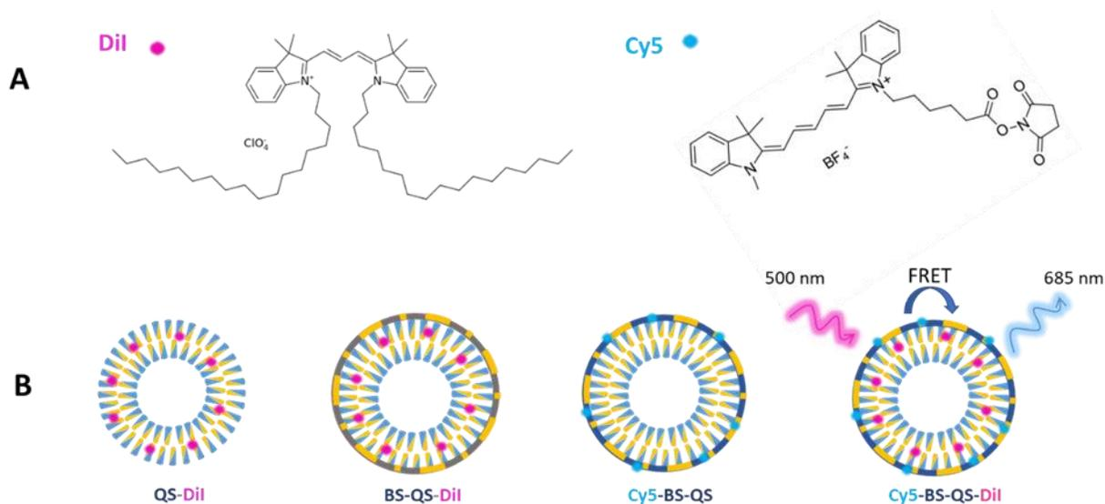
**Figure 4.3.** A) Dyes using for the labeled silica QS to produce the FRET system. B) Different systems for the labeled silica-coated QS to produce the Breakable labeled silica-coated QS with FRET.
