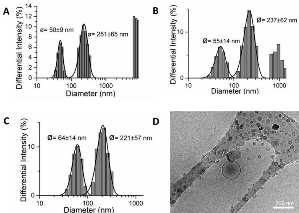
**Figure 5.6.** DLS measurements for the Breakable silica-coated MKC-QS. Using TEMOS and BTSPD-first change in methodology. Initial MKC-QS has a size of  $26\pm 19$  nm and  $81\pm 19$  nm. **A)** After the first addition of the mixture of silanes and 4 h of reaction, **B)** after the first addition and 1 day of reaction **C)** after the second addition and 1 h of reaction before dialysis stopped the reaction and **D)** Cryo-TEM images of the final sample.
