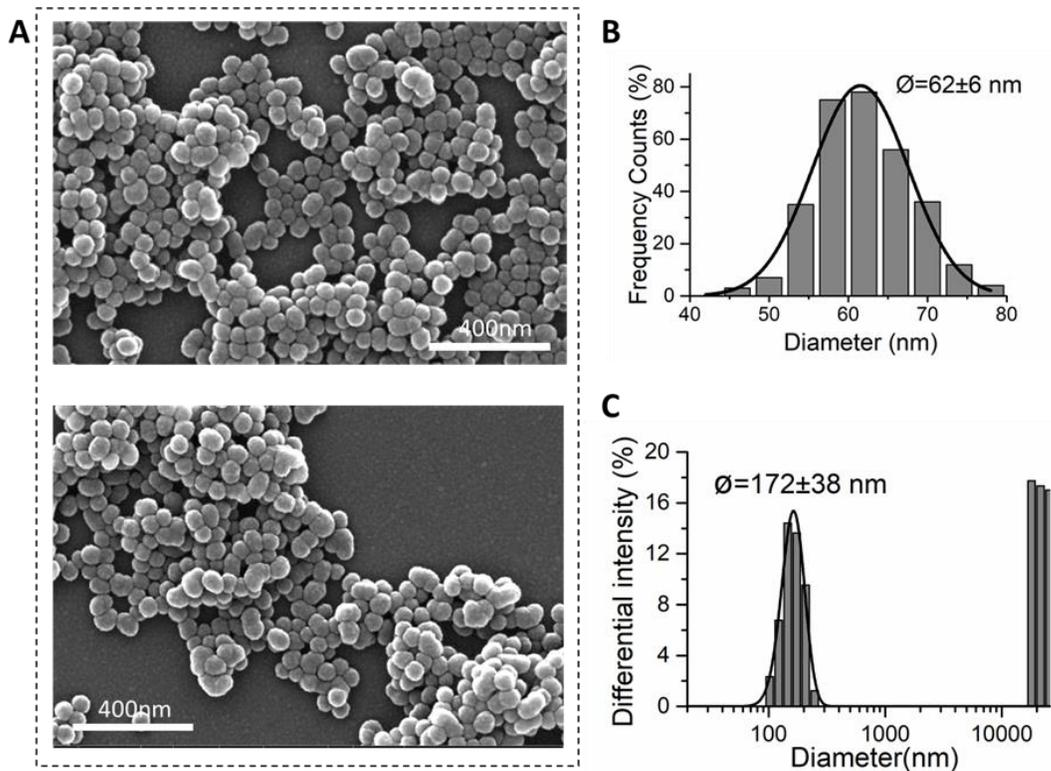
**Figure 5.11.** A) SEM pictures of non-breakable NPs prepared with a non-toxic surfactant (MKC). B) SEM counting of 300 NPs (size distribution  $62 \pm 6$  nm) C) DLS distribution  $172 \pm 38$  nm.
