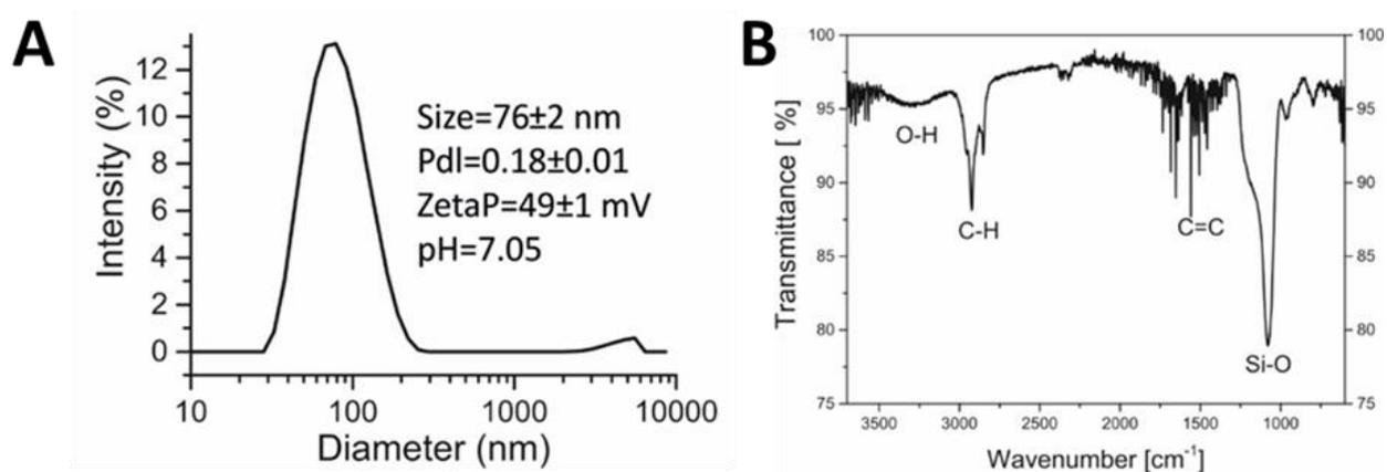
**Figure 3.21.** A) Size distribution of the 10% Dodecyl silane QS covered with TEOS after 2 days of reaction and B) IR spectra of silica dodecyl silane QS.
