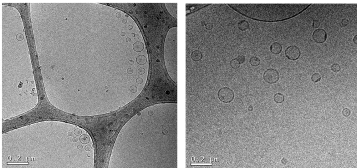
**Figure 3.39.** Cryo-TEM images of the responsible redox (BTSPD) silica-coated QS after 4 days of reaction. Scale bar 0.2  $\mu\text{m}$ .
