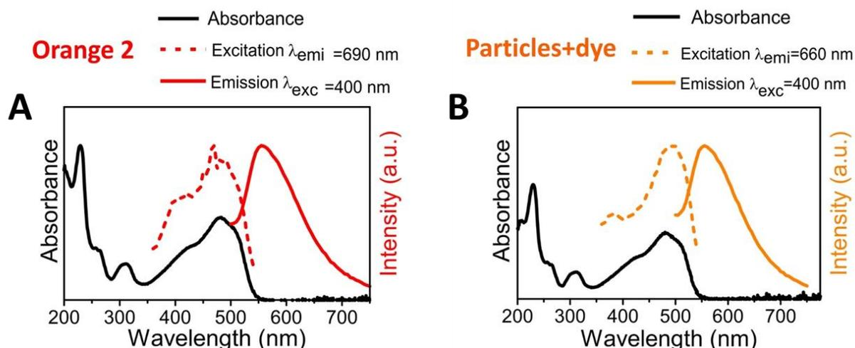
**Figure 2.44.** A) Absorption, Excitation and Emission spectra of A) Orange 2 and B) MSNPs loaded with Orange 2.
