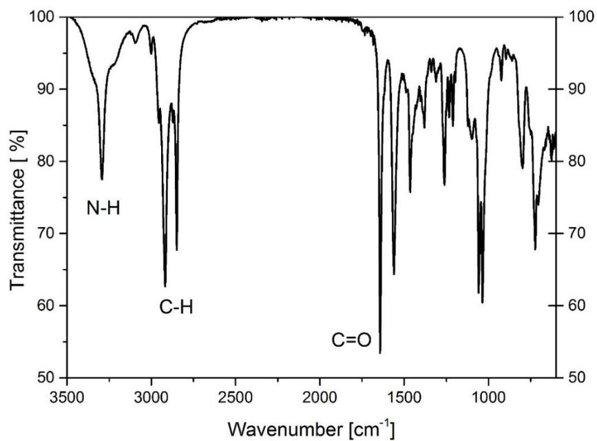
Figure 2.61. IR spectrum of *N*-(2-hydroxy ethyl) oleamide.
