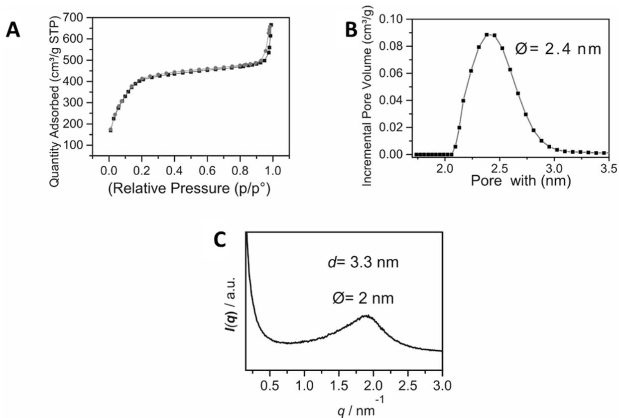
Figure 5.23. A)  $N_2$  adsorption-desorption isotherm of the Breakable NPs done with MKC, B) mesopore-size distribution and C) Small-angle X-ray scattering (SAXS) profile of the obtained mesoporous silica bulk.
