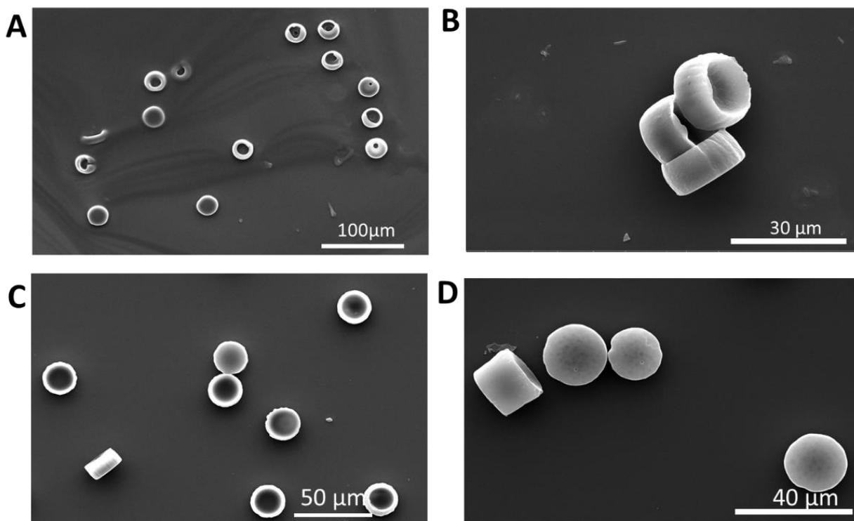
**Figure 2.34.** SEM pictures of the optimization of the production of PLGA-MBds using the hydrogel template technique. **A)** 20% PLGA MBds formed with the deposition of the solution using a razor, **B)** 30% PLGA MBds formed with the deposition of the solution using a razor putting 3 times layers of material. **C)** and **D)** 20% and 30% PLGA MBds formed with the deposition of the solution using a glass slide.
