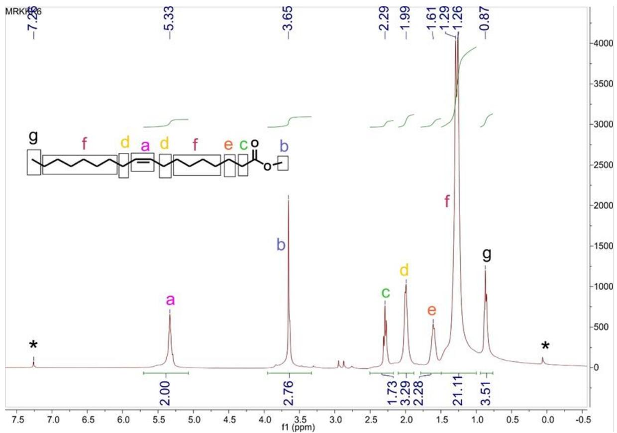
Figure 2.57.  $^1\text{H}$  NMR spectrum of methyl oleate.
