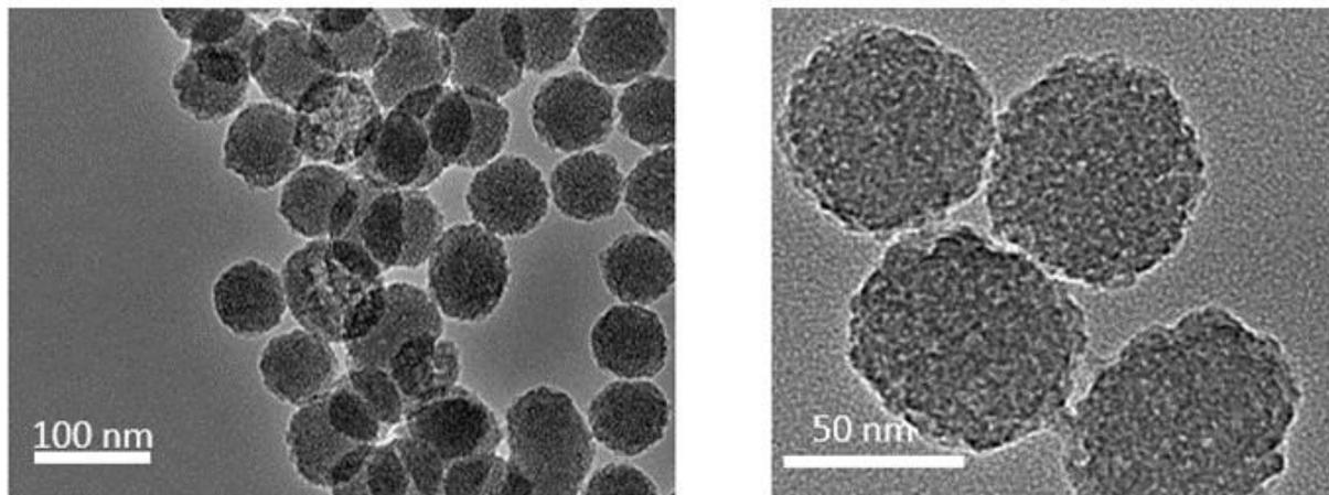
**Figure 5.27.** TEM images of the Breakable NPs done with MKC (Scale bar 100 and 50 nm).
