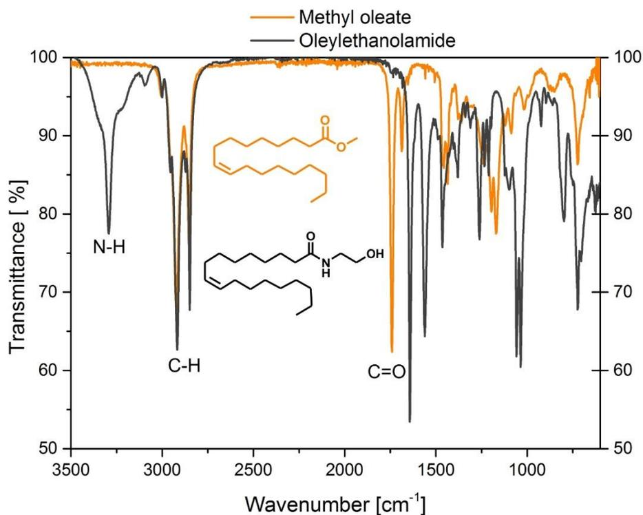
**Figure 2.63.** IR comparison between methyl oleate and *N*-(2-hydroxyethyl)oleamide (oleylethanolamide).
