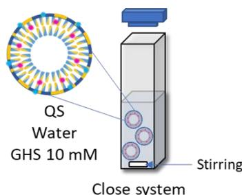
Figure 4.15. Experiment diagram for the breakability test (close system).
