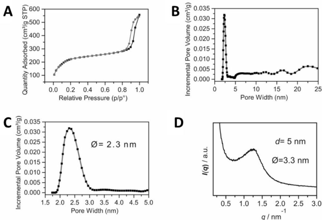
**Figure 5.17.** A)  $N_2$  adsorption-desorption isotherm of the Breakable NPs done with MKC, B) and C) mesopore-size distribution, D) Small-angle X-ray scattering (SAXS) profile of the obtained mesoporous silica bulk.
