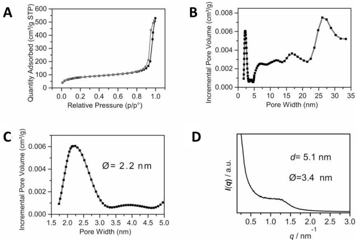
**Figure 5.26.** A)  $N_2$  adsorption-desorption isotherm of the Long Pore- Breakable NPs done with MKC, B) and C) mesopore-size distribution, D) Small-angle X-ray scattering (SAXS) profile of the obtained mesoporous silica bulk and.
