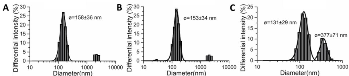
**Figure 3.4.** Size distribution of QS under stirring at 375 rpm and 20% of EtOH at different time of stirring **A)** 0h, **B)** 1h and **C)** 3h.
