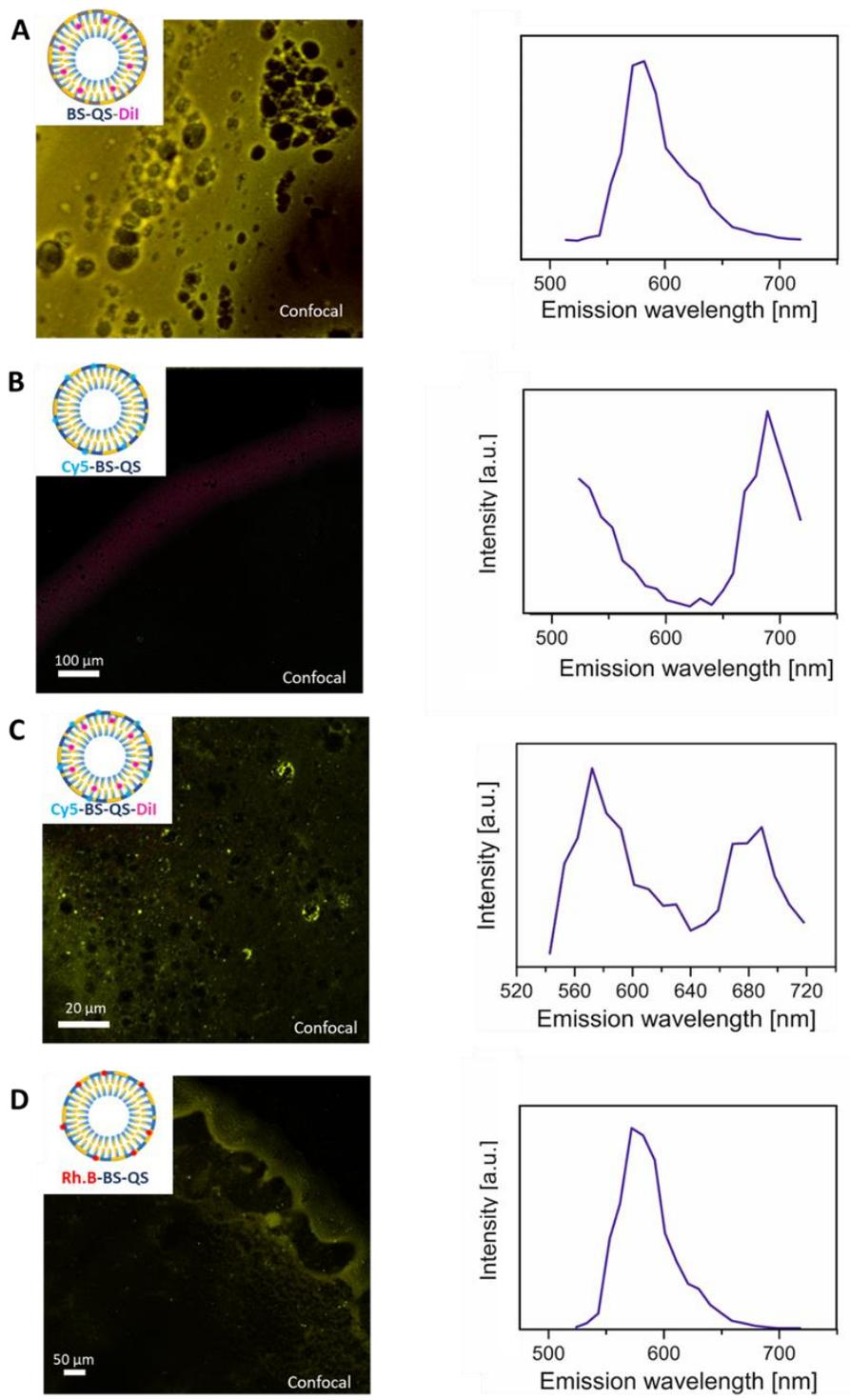
**Figure 4.8.** Image of the lambda mode and the emission spectra of the **A) BS-QS-Dil**, **B) Cy5-BS-QS**, **C) Cy5-BS-QS-Dil** and **D) Rh.B-BS-QS**. Using the Confocal microscope with a 64x Object. Excitation wavelength: 488 nm.
