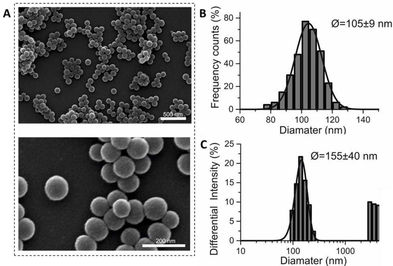
**Figure 5.7.** A) SEM pictures of non-breakable NPs prepared with a non-toxic surfactant (MKC). B) SEM counting of 300 NPs (size distribution  $105 \pm 9 \text{ nm}$ ) and C) DLS distribution ( $155 \pm 40 \text{ nm}$ ) of the particles.
