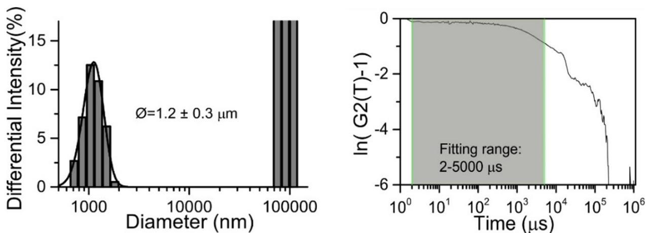
**Figure 2.31.** DLS result of size distribution of PLGA nanospheres produced from the SOAP methodology experiment with an average diameter of  $1.2 \pm 0.3 \mu\text{m}$ , data obtained from the fitting range of 2-5000 of the autocorrelation function of the sample.
