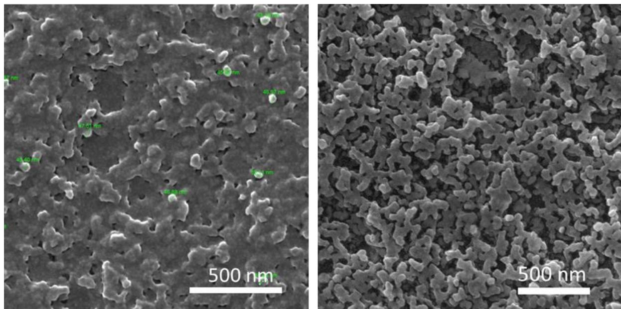
**Figure 3.23.** SEM images of 10% silica-coated Dodecyl silane QS after 5 days (reaction stopped by dialysis) and after 13 days (reaction still continue). Scale bar 500 nm.
