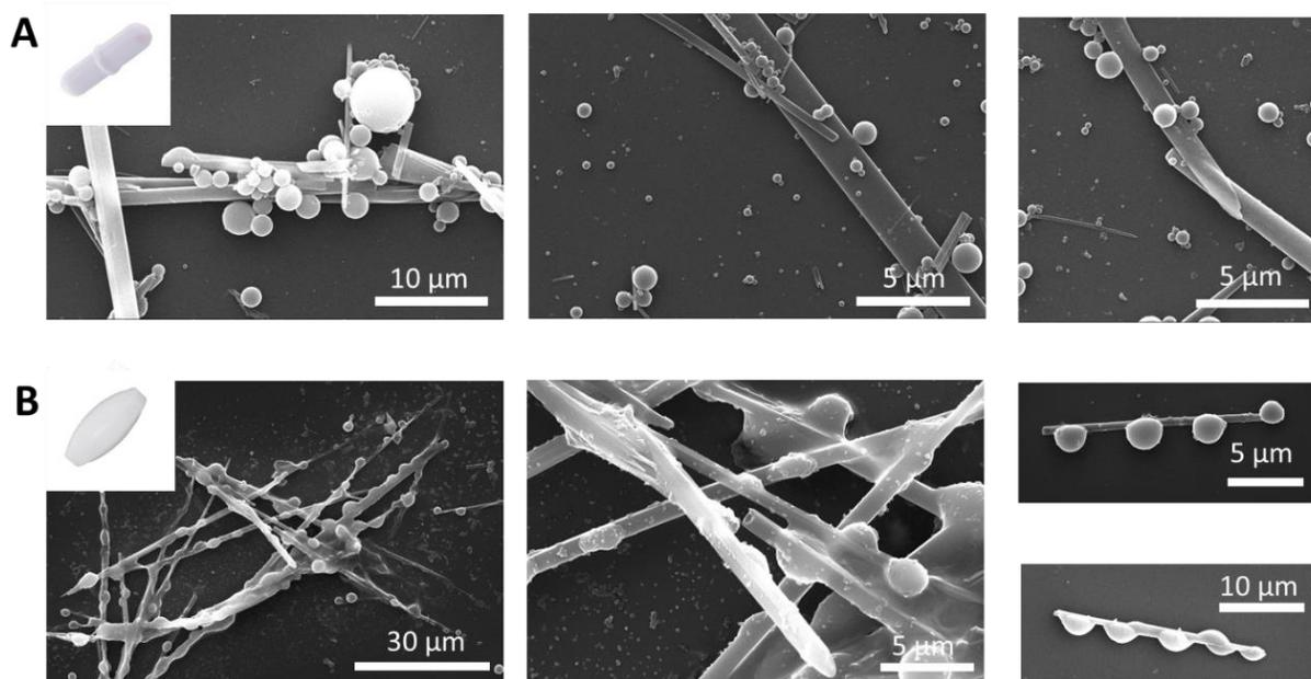
**Figure 2.29.** A) SEM image of the PLGA microspheres using the SOAP methodology and high speed of stirring (scale bare 10 and 5 µm). B) SEM image of the PLGA rods-nanospheres using the SOAP methodology big-scale 10x (scale bare 30, 10 and 5 µm).
