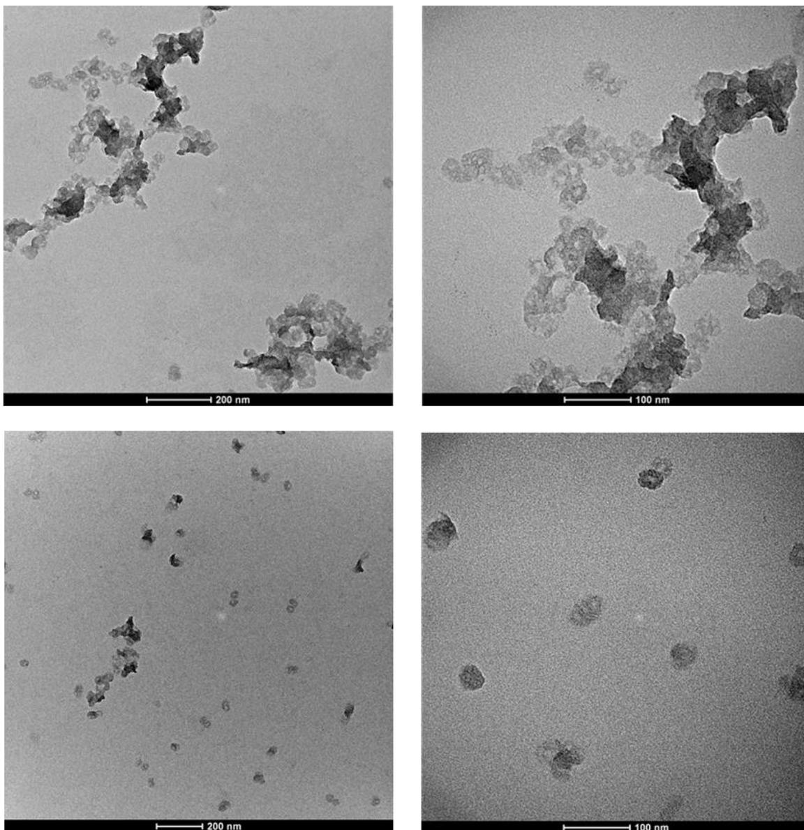
Figure 3.41. TEM images of breakable silica-coated QS (TEMOS+BTSPD). Scale bar 200 and 100 nm.
