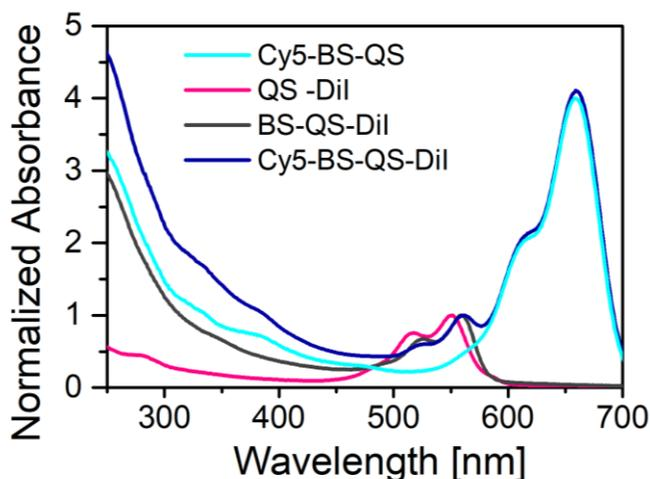
**Figure 4.4.** Absorbance of the different labeled silica-coated QS systems in the range of 200 to 700 nm.
