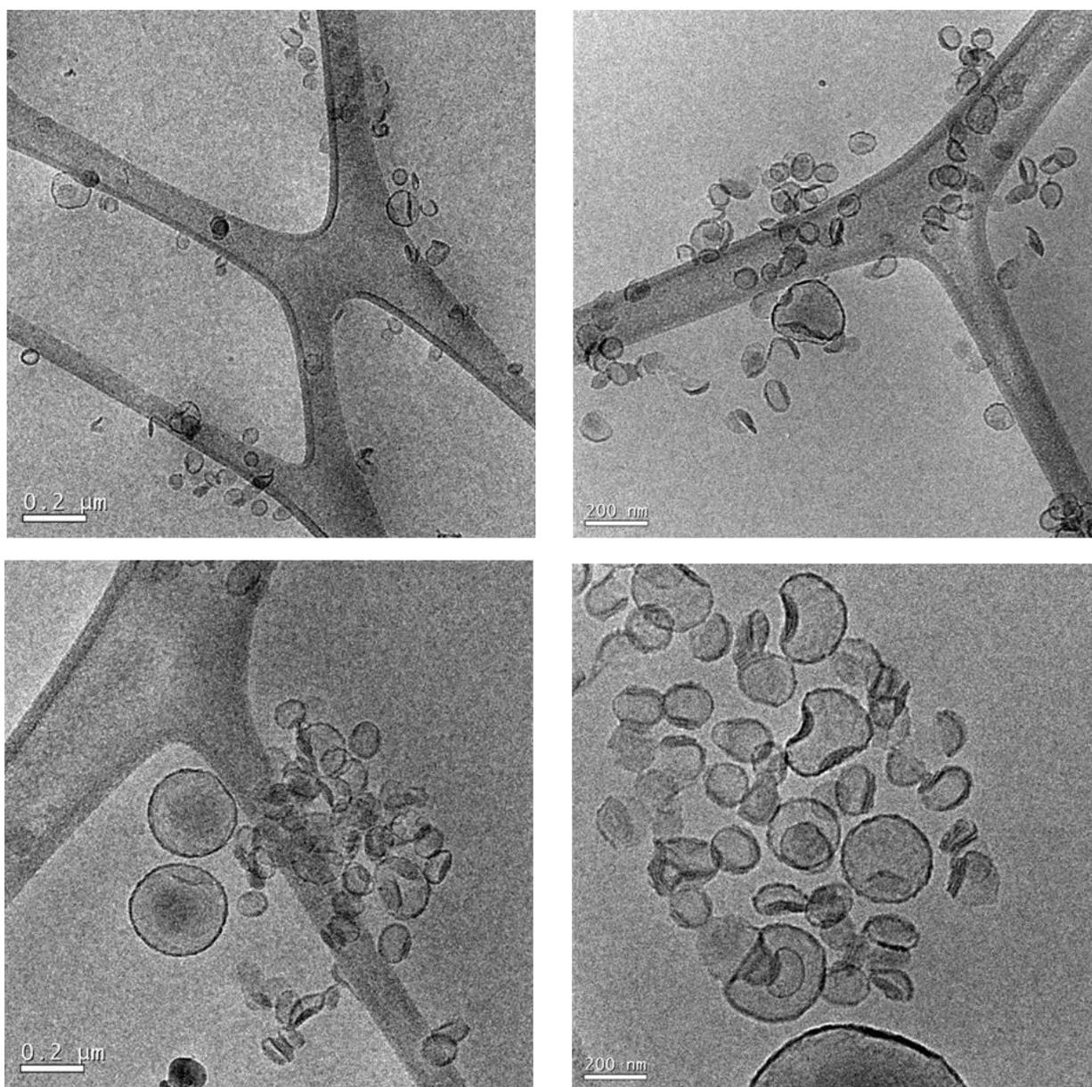
**Figure 3.29.** Cryo-TEM images of the 4.4 mM TEMOS silica-coated QS after 4 days of reaction. Scale bars, 200 nm.
