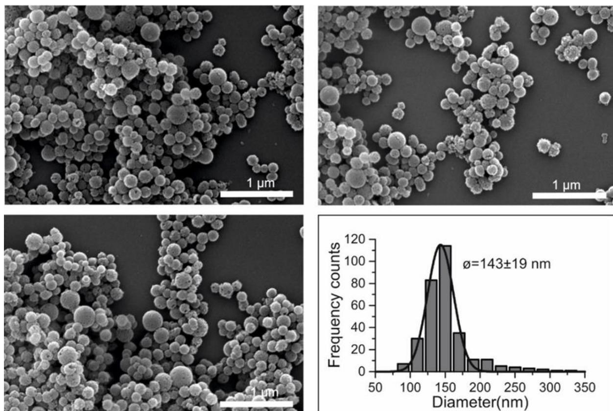
**Figure 3.31.** SEM pictures of the Breakable Silica covered Quatsomes (B-SQS) after overnight of stirring (scale bar 1  $\mu\text{m}$ ). Down right: SEM size distribution (count performed on 300 nanoparticles; average diameter 143 $\pm$ 19nm).
