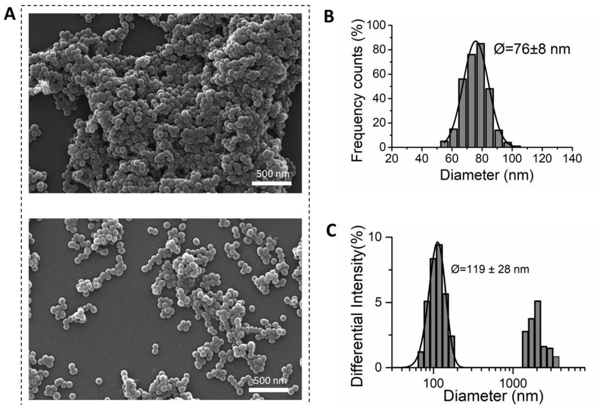
Figure 5.15. a) SEM pictures of breakable NPs prepared with a non-toxic surfactant (MKC). b) SEM counting of 300 NPs (size distribution  $76 \pm 8$  nm) c) DLS distribution  $119 \pm 26$  nm.
