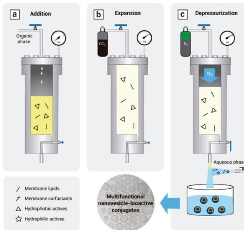
**Figure 3.43.** A) Schematic representation of the DELOS-SUSP method for the efficient preparation of multifunctional nanovesicle–bio-active hybrids. Extracted from ref. <sup>12</sup> Copyright 2013, with permission from American Chemical Society.
