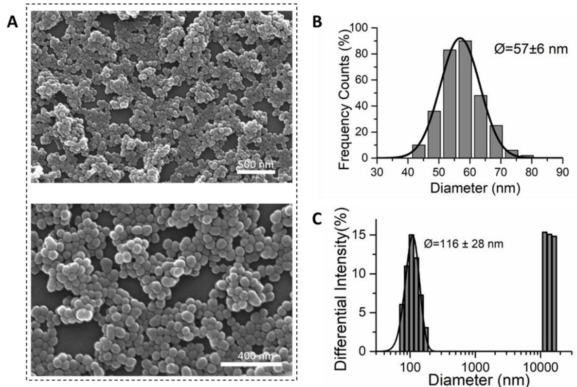
**Figure 5.14.** A) SEM pictures of Breakable NPs prepared with a non-toxic surfactant (MKC). B) SEM counting of 300 NPs (size distribution  $57 \pm 6 \text{ nm}$ ) C) DLS distribution  $116 \pm 28 \text{ nm}$ .
