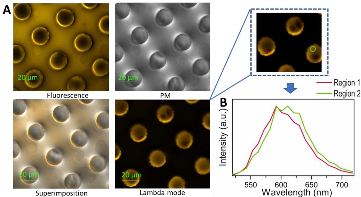
**Figure 2.40. A)** Confocal microscope images of AEA-PLGA@MBds loaded with Nile Red using 63x objective (scale bar 20μm). **B)** Emission spectra of the lambda mode of AEA taken from two different areas of the AEA-PLGA@MBds confocal images.
