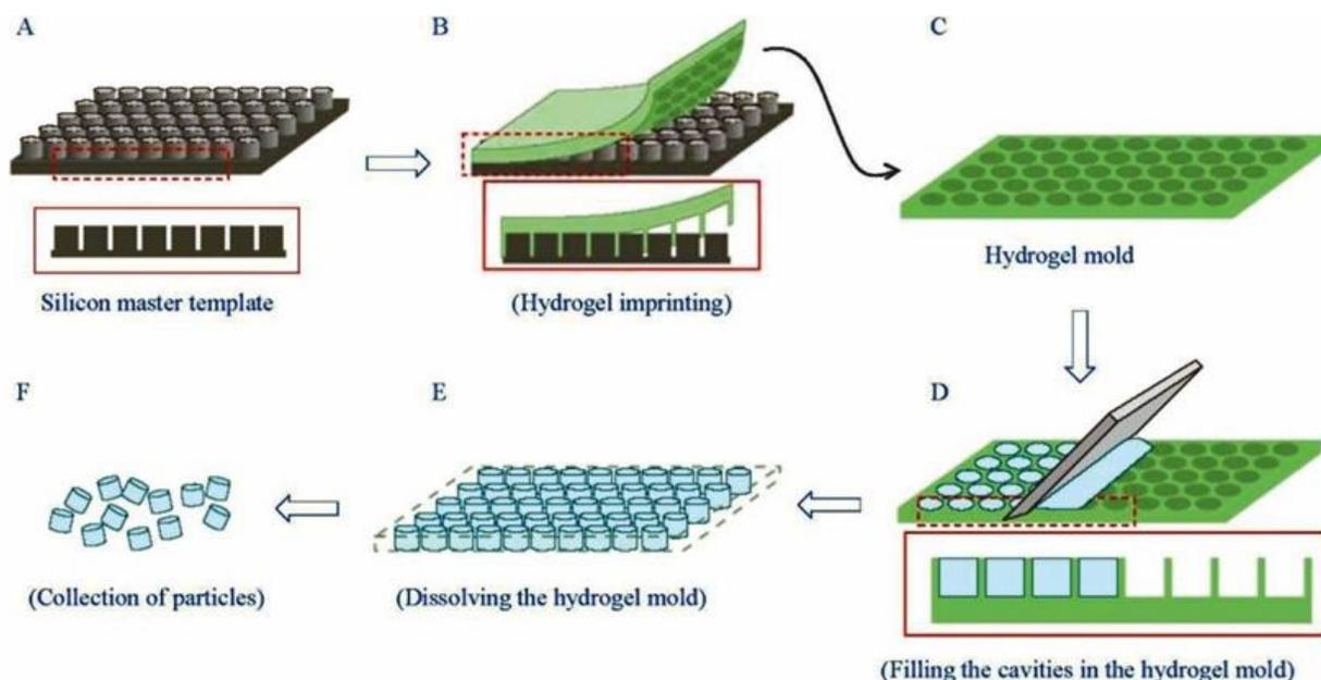
**Scheme 2.10.** Mold method of microparticle fabrication through the hydrogel template method. Reprinted with permission from AKINA, INC (Copyright 2015).
