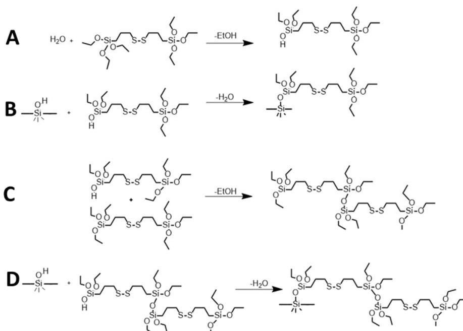
**Figure 5.18.** A) Hydrolysis of One Ethoxy group of BTSPD B) Grafting through condensation of hydrolyzed silane and silica silanols, C) Oligomerization trough reaction between a nonhydrolyzed and a hydrolyzed species, D) Grafting of the oligomerized BTSPD to the silica framework. Adapted with permission from ref 38. (Copyright 2014, American Society for Microbiology)
