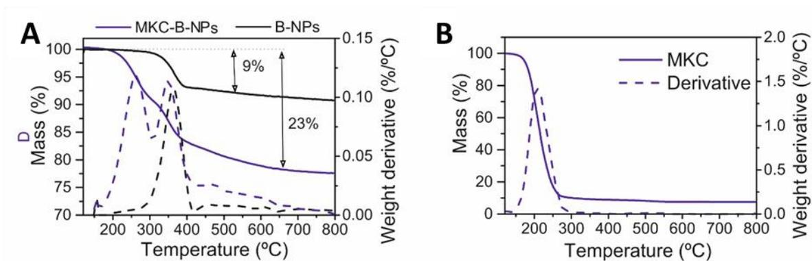
Figure 5.16. A) TGA of the Breakable MKC NPs before and after the extraction of the MKC and B) MKC surfactant (Micellar templating method).
