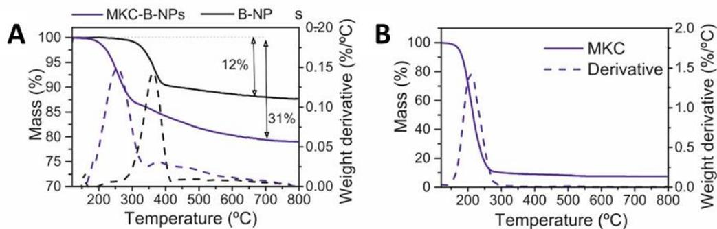
**Figure 5.12.** A) TGA of the Breakable MKC NPs before and after the extraction of the MKC and B) MKC surfactant.
