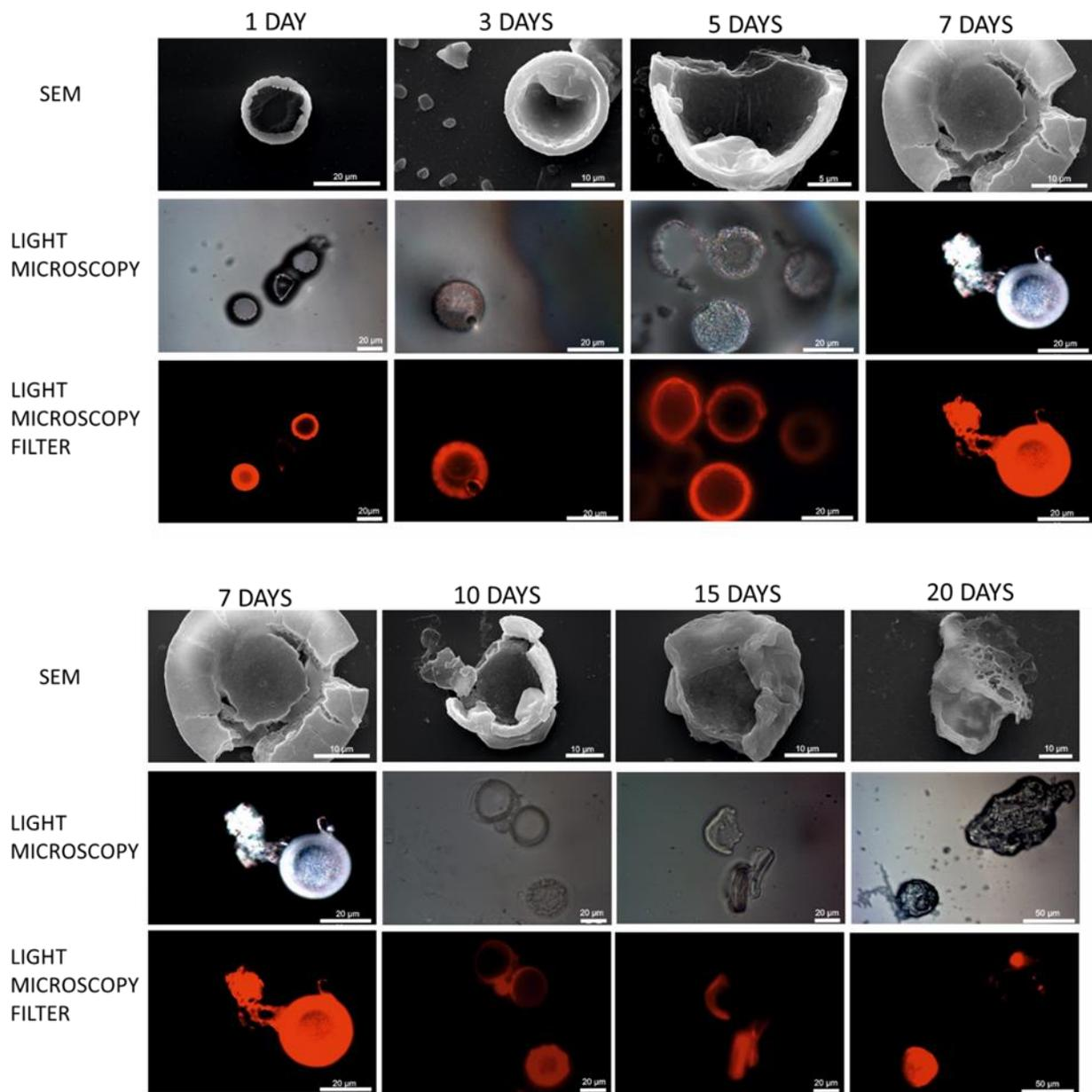
**Figure 2.50.** SEM, Light microscopy, and light microscopy using a filter of the degradation of the PLGA@MBDs loaded with Nile Red in PBS pH 7 media and 37 °C, followed during the time for 20 days.
