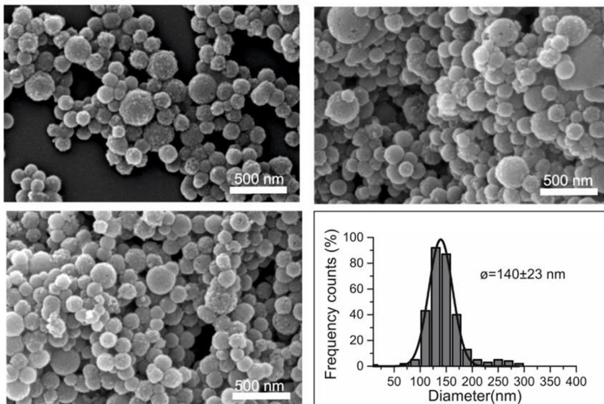
**Figure 3.9.** SEM pictures of the SQS after overnight stirring (scale bar 500 nm). Down right: SEM size distribution (count performed on 300 nanoparticles; average diameter  $140\pm 23$  nm).
