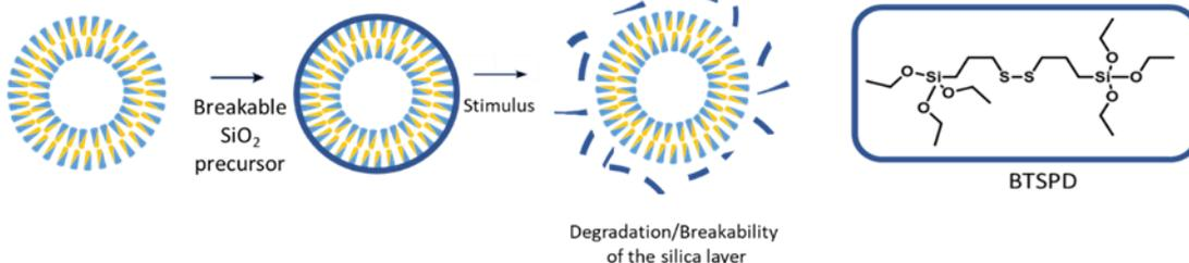
**Figure 3.2.** Synthesis of non-breakable silica and breakable coated QS and the silane precursors employed in each case.
