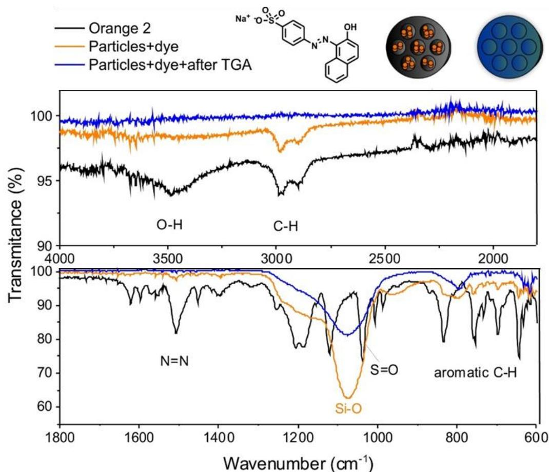
**Figure 2.43.** IR spectra of Orange 2 dye, particles loaded with Orange 2 and particles loaded after TGA; line black, orange and blue, respectively.
