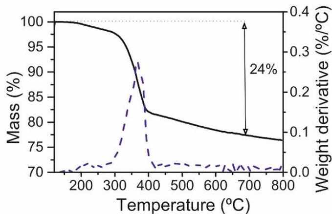
Figure 5.22. A) TGA of the Breakable MKC NPs after the extraction of the MKC (Stöber process).
