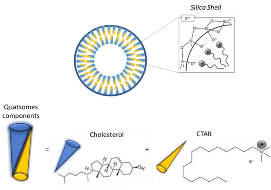
**Figure 3.1.** Representation of a silica-coated QS. The bilayer of the QS is formed by CTAB and cholesterol. In basic conditions electrostatic interactions make possible the interaction between the silica (negatively charged) and the QS (positive charge).
