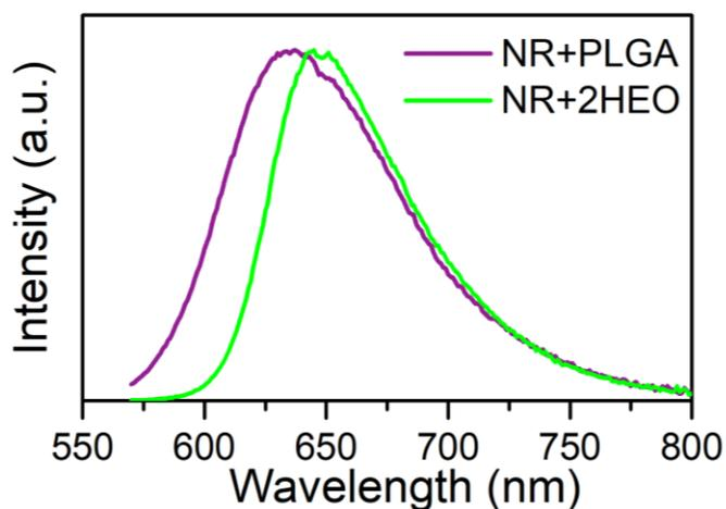
**Figure 2.38.** Emission spectra of NR in PLGA and NR with 2HEO using a fluorimeter.
