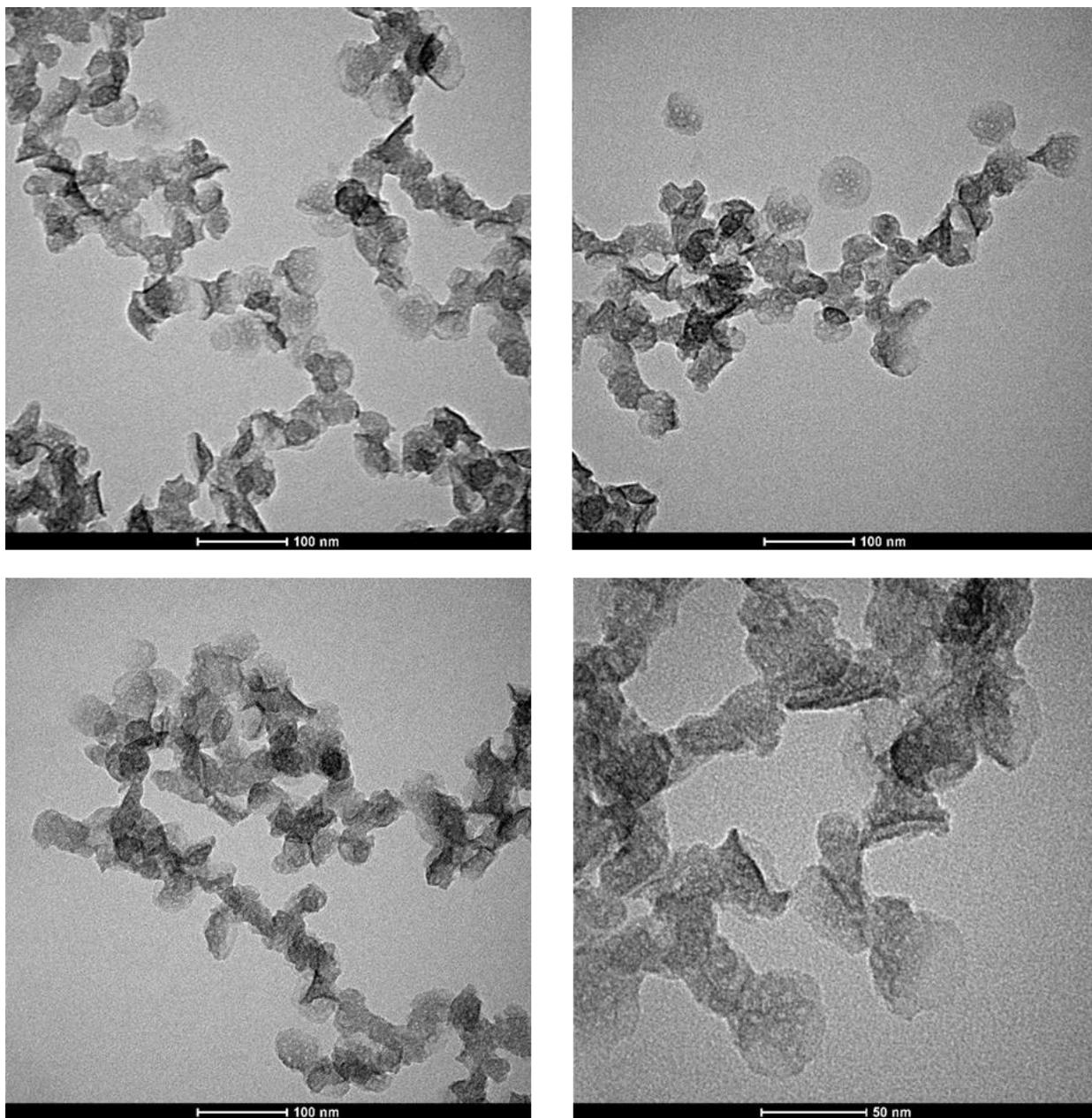
**Figure 3.27.** TEM images of 10% silica-coated Dodecyl silane QS with not pos-treatment to the reaction. Scale bar 100 and 50 nm.
