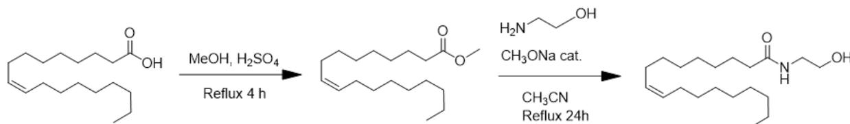
Scheme 2.15. Synthesis route of 2HEO from oleic acid.
