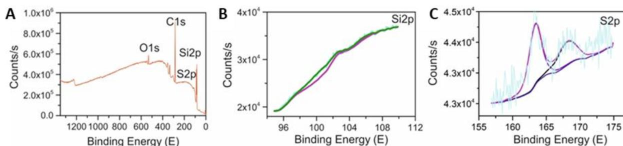
**Figure 3.34. A)** Representative X-Ray Photoelectron Spectroscopy (XPS) spectra analysis of the surfaces of B-SQS **B)** Silicon analysis, deconvolution of the Si2p core level spectra and **C)** Sulfur analysis, deconvolution of the S2p core level.
