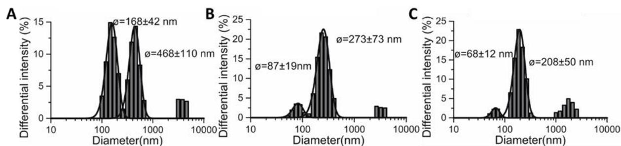
**Figure 3.30.** DLS experiments of the silica covered Quatsomes (SQS) **A)** after the addition of silanes, **B)** 1 h, **C)** overnight.
