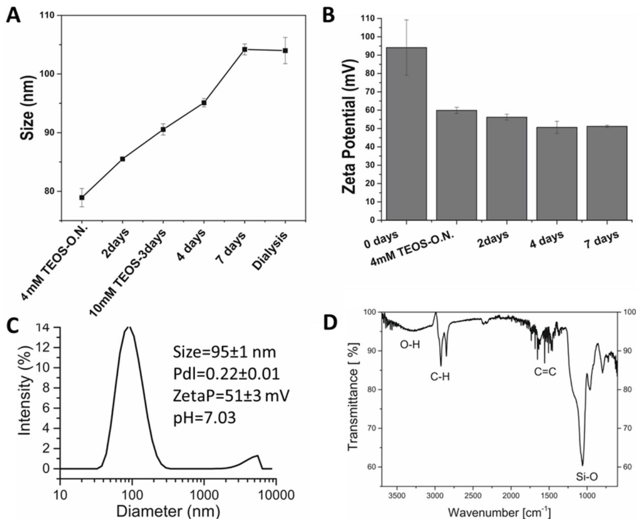
**Figure 18.** **A)** DLS-Size and **B)** Zeta Potential measurement of the reaction over time of TEOS silica-coated QS at 0 °C for 7 days. **C)** DLS-Size distribution measurement after 4 days of reaction the NB-QS-TEOS. **D)** IR spectra of silica-coated QS. The starting material has a size of 84±1 nm a Pdl of 0.23±0.01 and a Zeta Potential of 84±2 mV.
