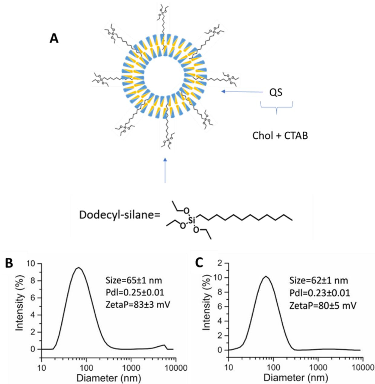
Figure 3.19. A) Representation of the Dodecyl-silane-QS and their DLS-Size distribution measurement of B) 5% C) 10% wt Dodecyl silica QS.
