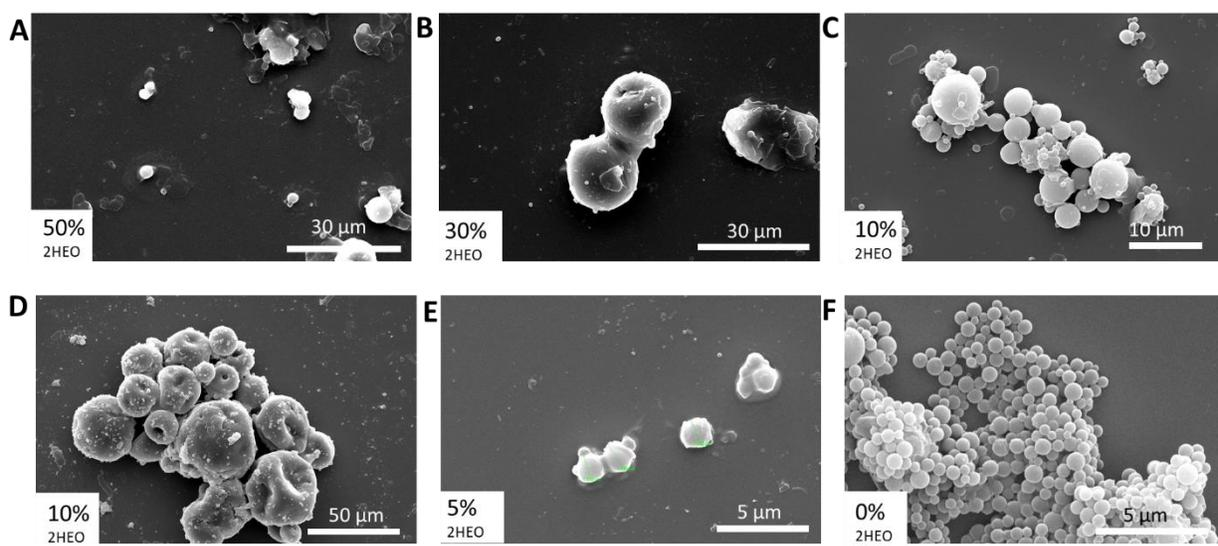
**Figure 2.33.** SEM images of the incorporation of **A)** 50%, **B)** 30%, **C)** and **D)** 10%, **E)** 5% and **F)** 0% w/w of 2HEO in the PLGA nanospheres using the SOAP methodology.
