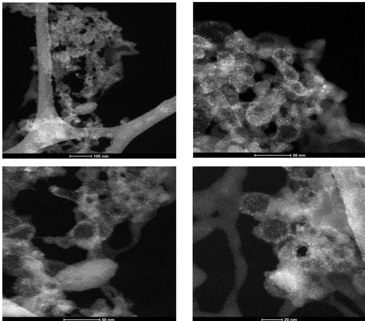
**Figure 3.35.** Cryo-STEM image of breakable silica-coated QS (APTES+BTSPD). Scale bar 100, 50 and 20 nm.
