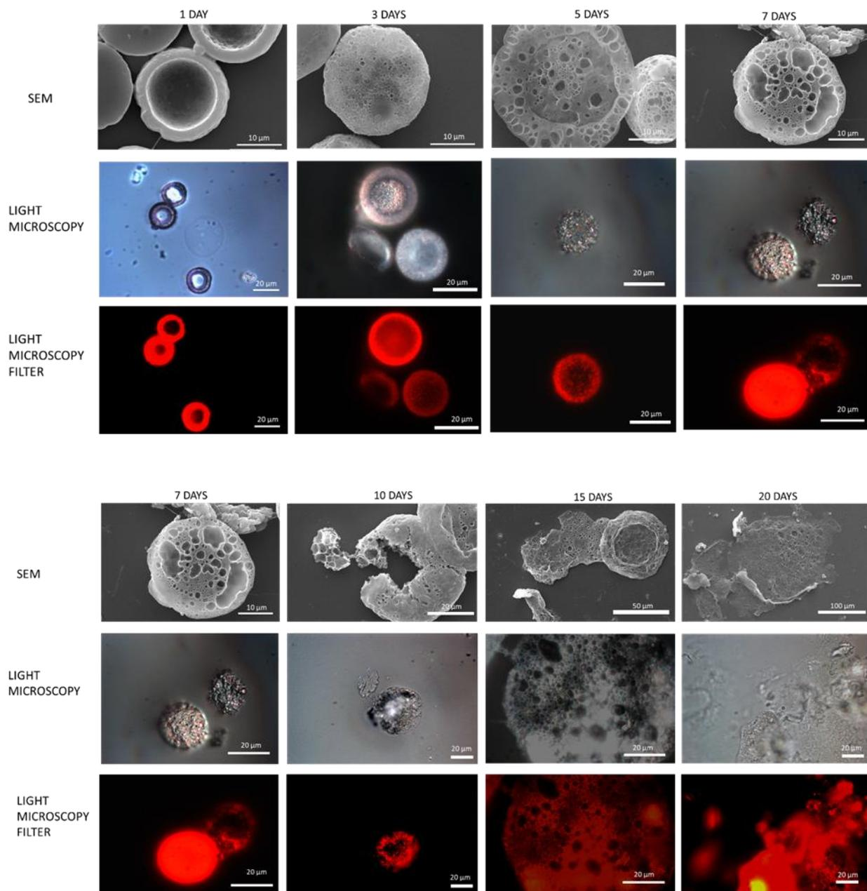
**Figure 2.49.** SEM, Light microscopy, and light microscopy using a filter of the degradation of the PLGA@MBDs loaded with Nile Red in water media (pH 5.2) and 37 °C, followed during the time for 20 days.
