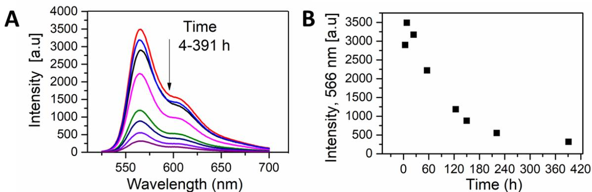
**Figure 4.25.** A) Emission of the QS loaded with Dil and put them in PBS and stirring up 391 h. B) Intensity at 566 nm of the QS-Dil during the time.
