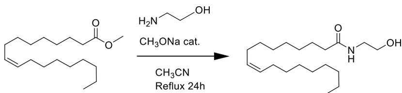
Scheme 2.17. Synthesis of *N*-(2-hydroxy ethyl) oleamide from methyl oleate.
