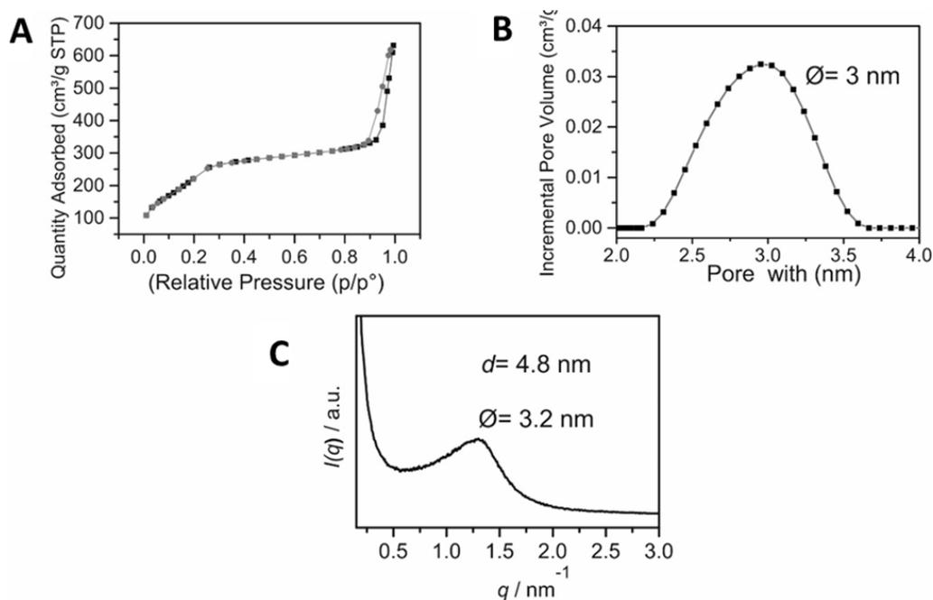
**Figure 5.9.** A) N<sub>2</sub> adsorption-desorption isotherm of the prepared bulk, B) mesopore-size distribution and C) Small-angle X-ray scattering (SAXS) profile of the obtained mesoporous silica bulk.
