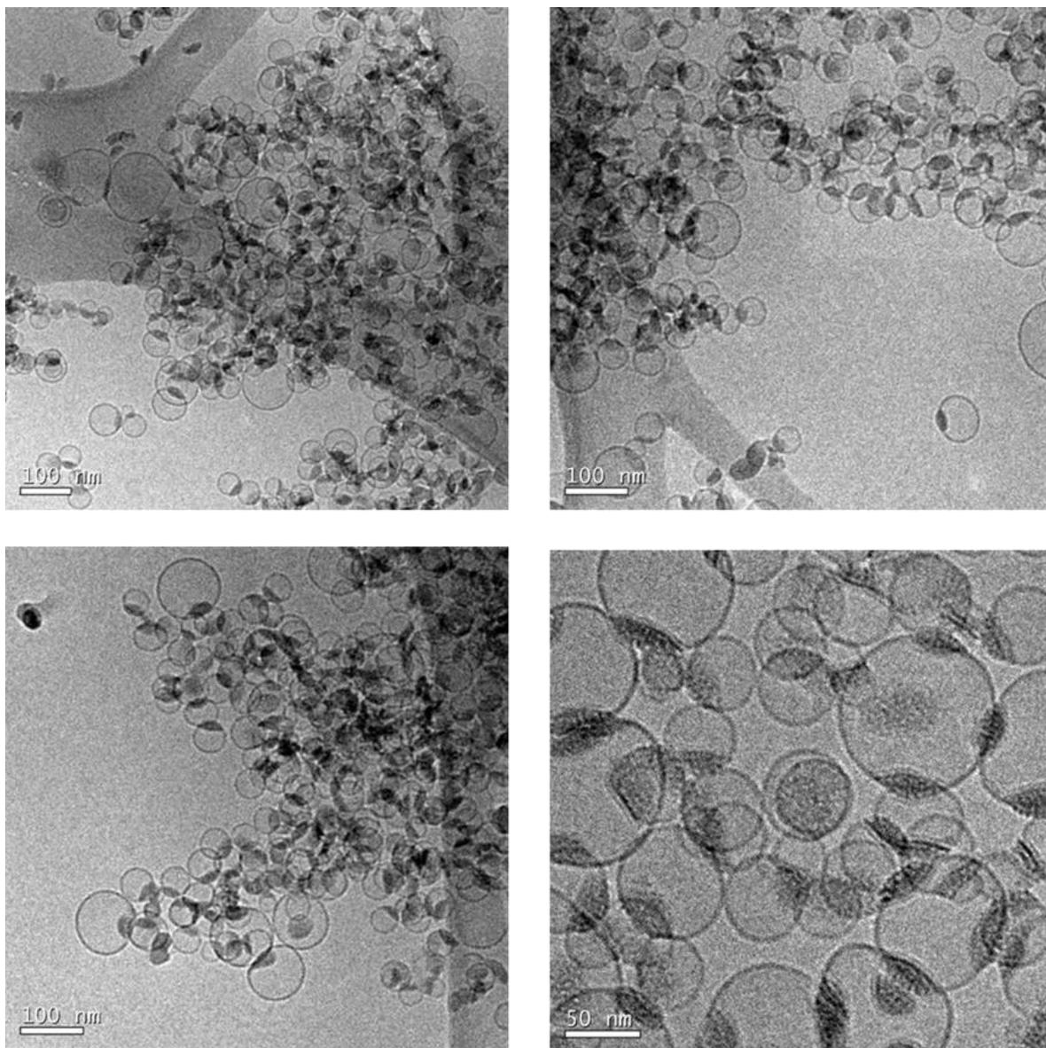
**Figure 3.16.** Cryo-TEM images of the 10 mM TEOS silica-coated QS at 20 °C after dialysis. Scale bars, 100 and 50 nm.
