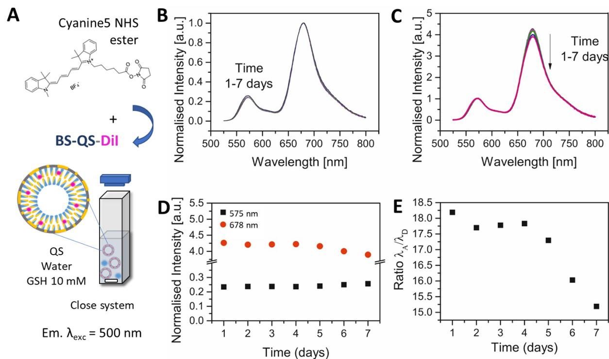
**Figure 4.24.** **A**) Experiment diagram for the permeability test using BTSPD-QS-Dil (breakable shell). **B**) and **C**) Normalised Intensity of the Emission of the BTSPD-QS-Dil; normalised by the Cyanine5 and the Dil band, respectively. **D**) Normalised intensity of the emission at 575 and 678 nm representing the Dil and the Cyanine5. **E**) Ratio Acceptor/Donor of the sample after 7 days.
