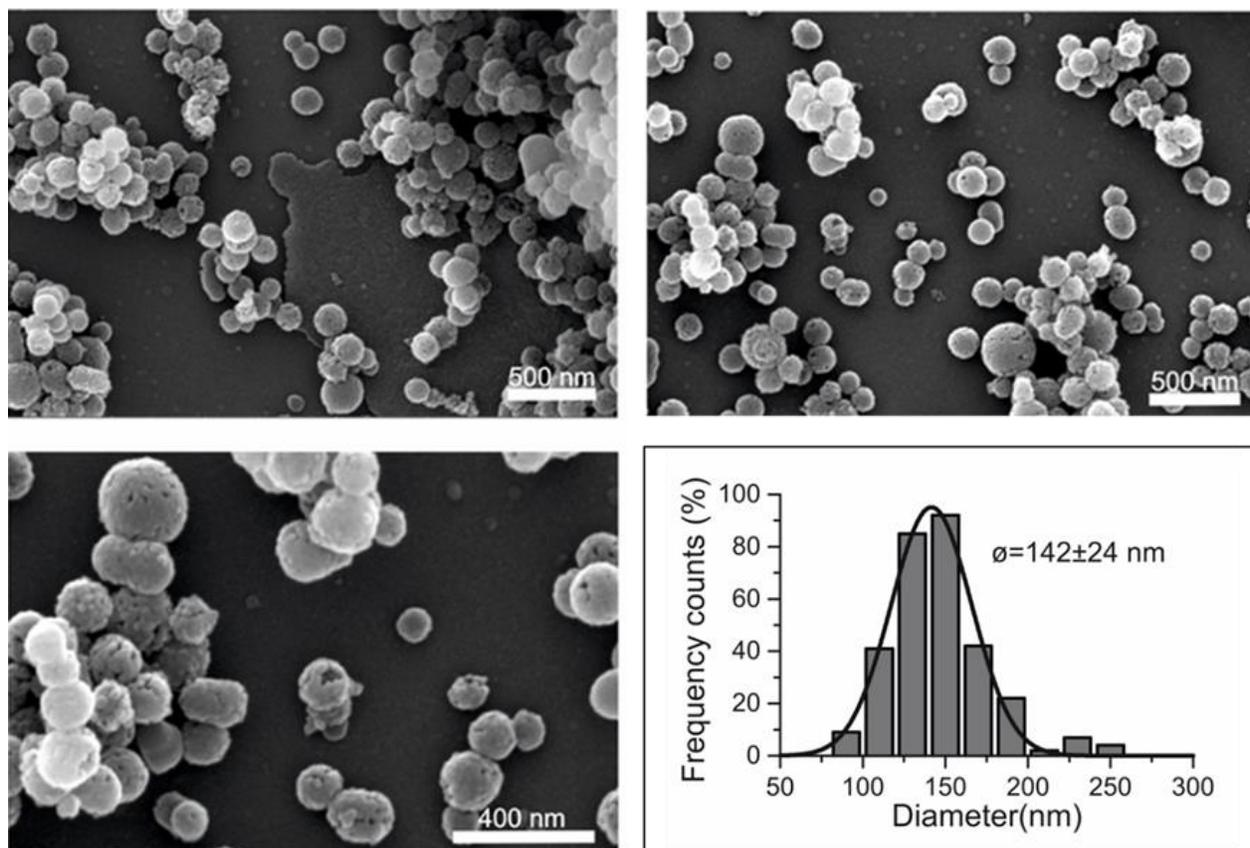
**Figure 3.11.** SEM pictures of the silica covered Quatsomes (SQS) after overnight of stirring (scale bar 500 nm and 400 nm) using a concentrated methodology to produce them. Down right: SEM size distribution (count performed on 300 nanoparticles; average diameter  $142 \pm 24$  nm).
