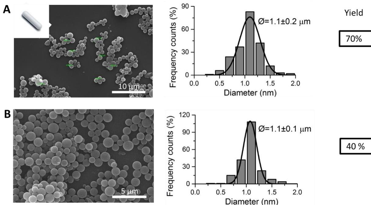
**Figure 2.30.** 5x Upscale reaction of the PLGA- spheres by the SORP methodology using a flat stirring bar and do it twice. SEM and their frequency counts reveal of 300 particles. First synthesis **A**) size diameter of  $1.1 \pm 0.2 \mu\text{m}$  and 70% of yield. Second synthesis **B**) size diameter of  $1.1 \pm 0.1 \mu\text{m}$  with 40% of yield.
