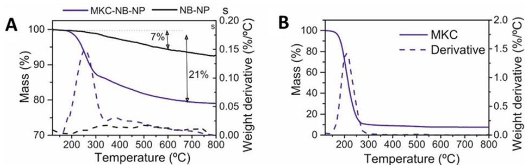
**Figure 5.8.** A) TGA of the Non-breakable MKC NPs before and after the extraction of the MKC and B) MKC surfactant.
