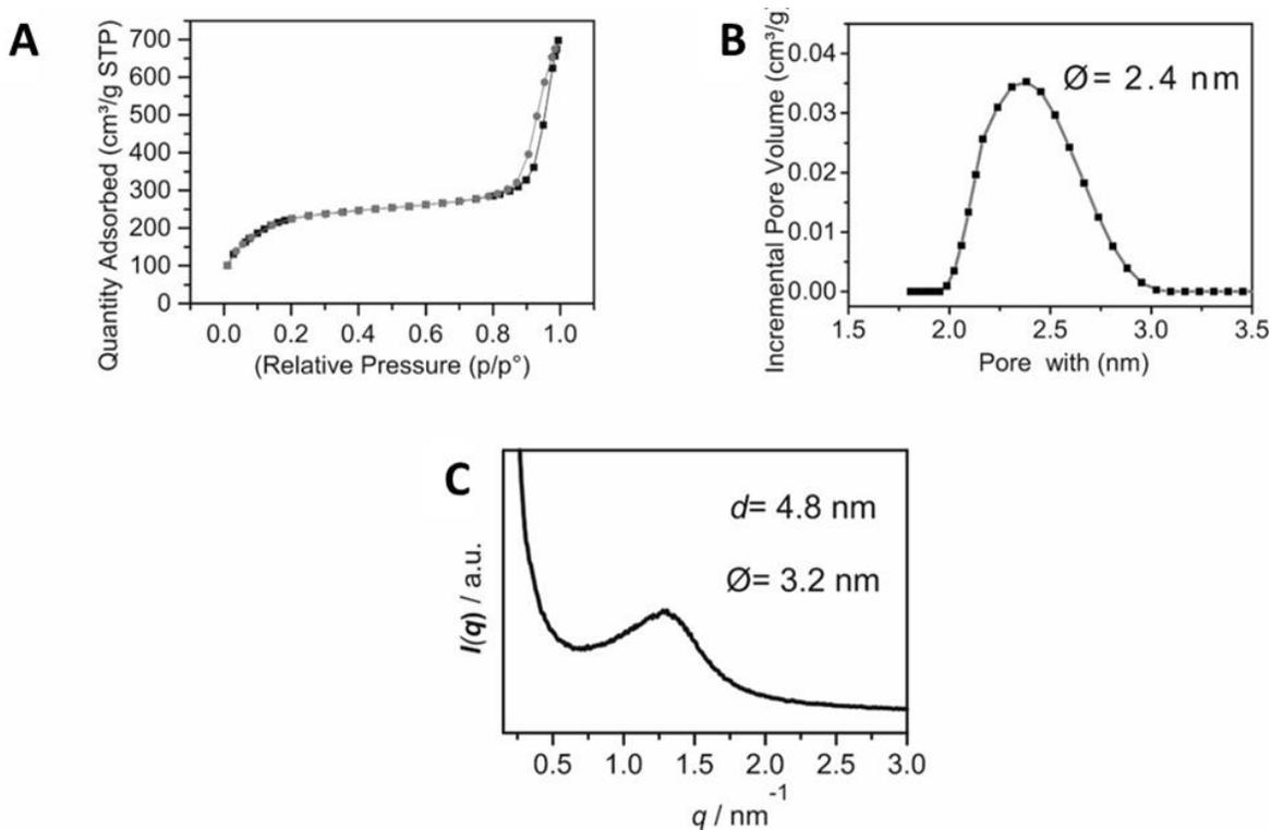
**Figure 5.13.** A) N<sub>2</sub> adsorption-desorption isotherm of the Breakable NPs done with MKC, B) mesopore-size distribution and C) Small-angle X-ray scattering (SAXS) profile of the obtained mesoporous silica bulk.
