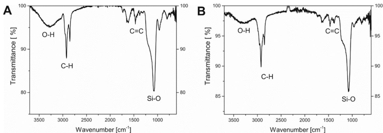
**Figure 3.17.** IR spectra of TEOS silica-coated QS at **A)** 0 °C and **B)** 20 °C.
