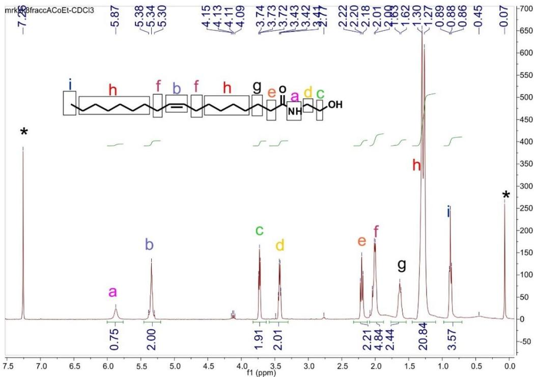
Figure 2.59. <sup>1</sup>H NMR spectrum of *N*-(2-hydroxy ethyl) oleamide.
