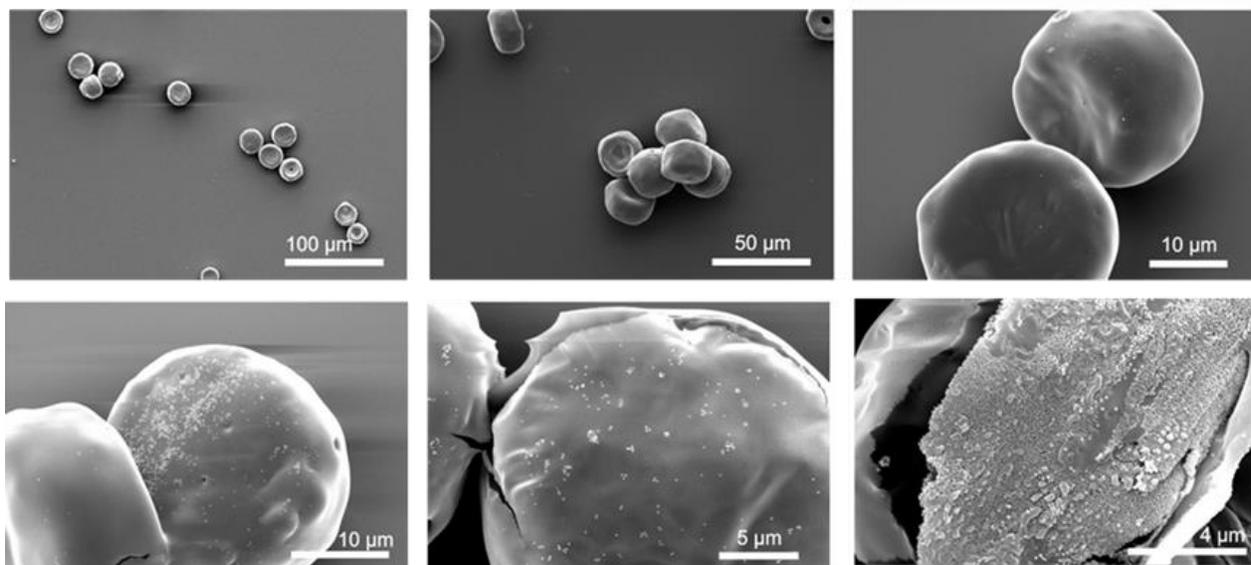
**Figure 2.47.** SEM images of the NPs-PLGA@MBds microparticles containing NPs and loaded with orange 2 (Scale bars 100, 50, 10, 5 and 4 μm).
