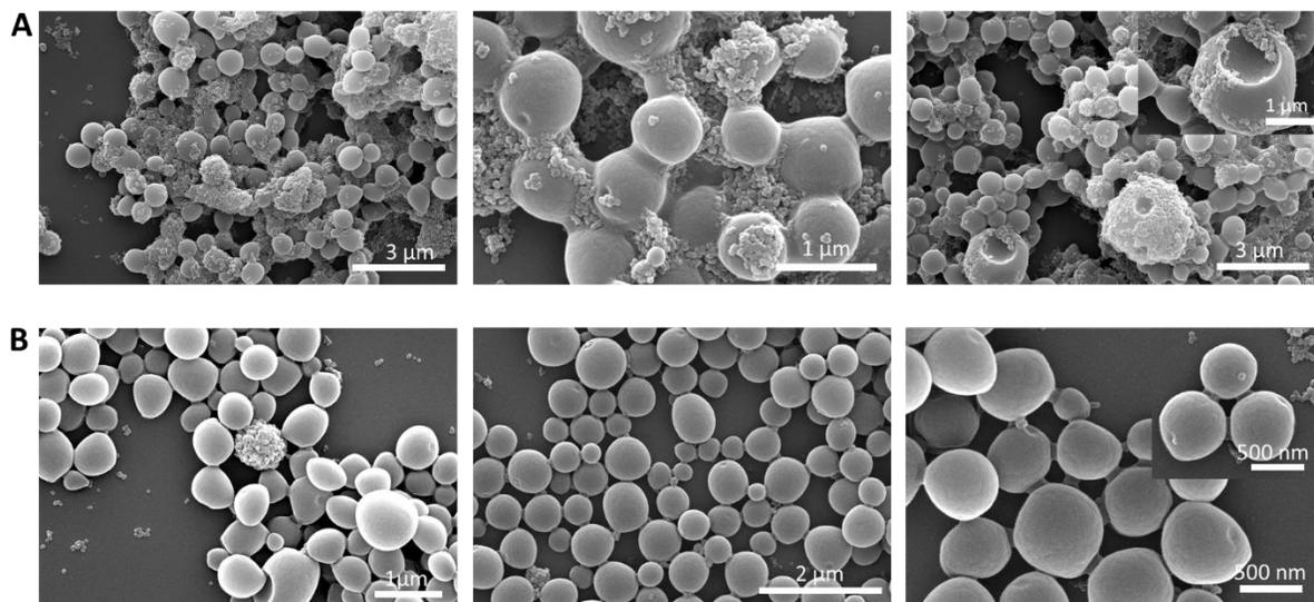
**Figure 2.32.** SEM image of the incorporation of **A)** 20% w/w and **B)** 5% MSNPs in the PLGA nanospheres using the SOAP methodology (scale bare 3, 2, 1 μm and 500 nm).
