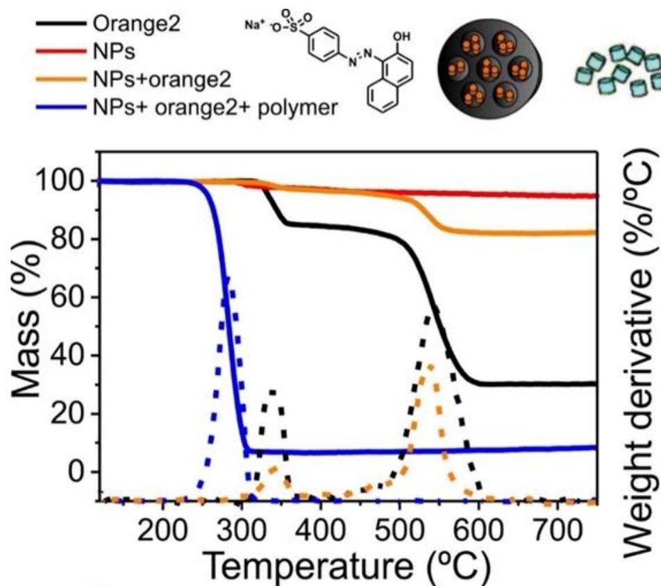
**Figure 2.48.** TGA analysis of the microparticles containing NB-NPs loaded with orange dye (line blue), and the comparison with NB-NPs (line red), NPs loaded with orange 2 (line orange) and the dye (line black).
