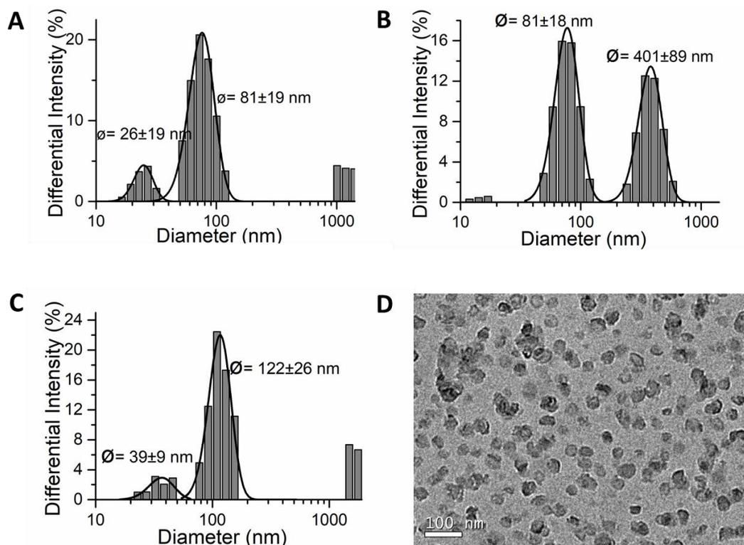
**Figure 5.5.** DLS measurements for the Breakable silica-coated MKC-QS. Using TEMOS and BTSPD-first change in methodology. **A)** Initial MKC-QS, **B)** After the first addition of the mixture of silanes and 1 day of reaction, **C)** after the second addition and 20 mins of reaction before dialysis stopped the reaction and **D)** Cryo-TEM images of the final sample.
