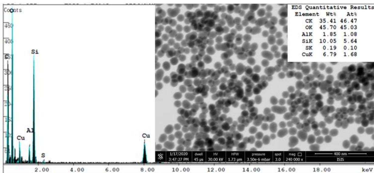
Figure 5.20. EDX of the Breakable MKC NPs.
