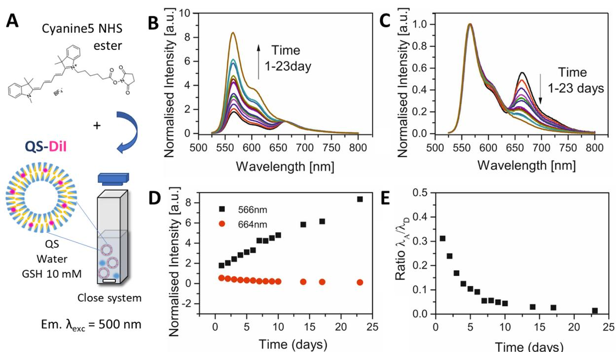
**Figure 4.21.** **A)** Experiment diagram for the permeability test using QS-Dil (without silica coating). **B)** and **C)** Normalised Intensity of the Emission of the QS-Dil; normalised by the Cyanine5 and the Dil, respectively. **D)** Normalised intensity of the emission at 566 and 664 nm representing the Dil and the Cyanine5. **E)** Ratio Acceptor/Donor of the sample after 24 days.
