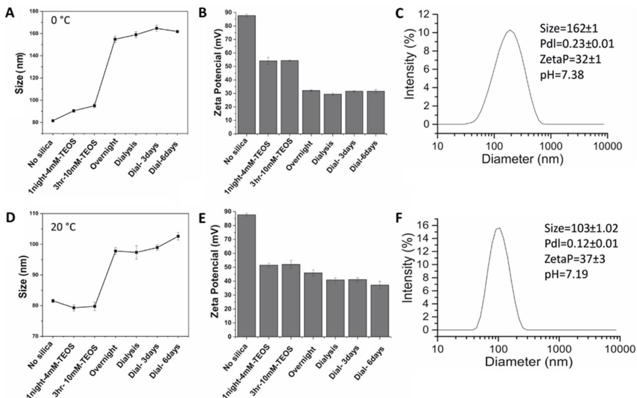
**Figure 3.14.** DLS-Size distribution of the reaction over time of TEOS silica-coated QS at **A)** 0 °C and **D)** 20 °C that was carried out by DLS. Zeta Potential of the reaction over time of TEOS silica-coated QS at **B)** 0 °C and **E)** 20 °C. DLS- measurement after dialysis of the NB-QS-TEOS at **C)** 0 °C and **F)** 20 °C. The starting material has a size of 82±1 nm a Pdl of 0.22±0.01 and a Zeta Potential of 88±1 mV.
