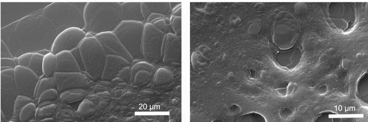
**Figure 3.12.** SEM pictures of the drop casting silica covered Quatsomes (SQS) after overnight of stirring (scale bar: 20 and 10  $\mu\text{m}$ ); in the interior of the drop; all the sample is broken due to the vacuum of the SEM equipment.
