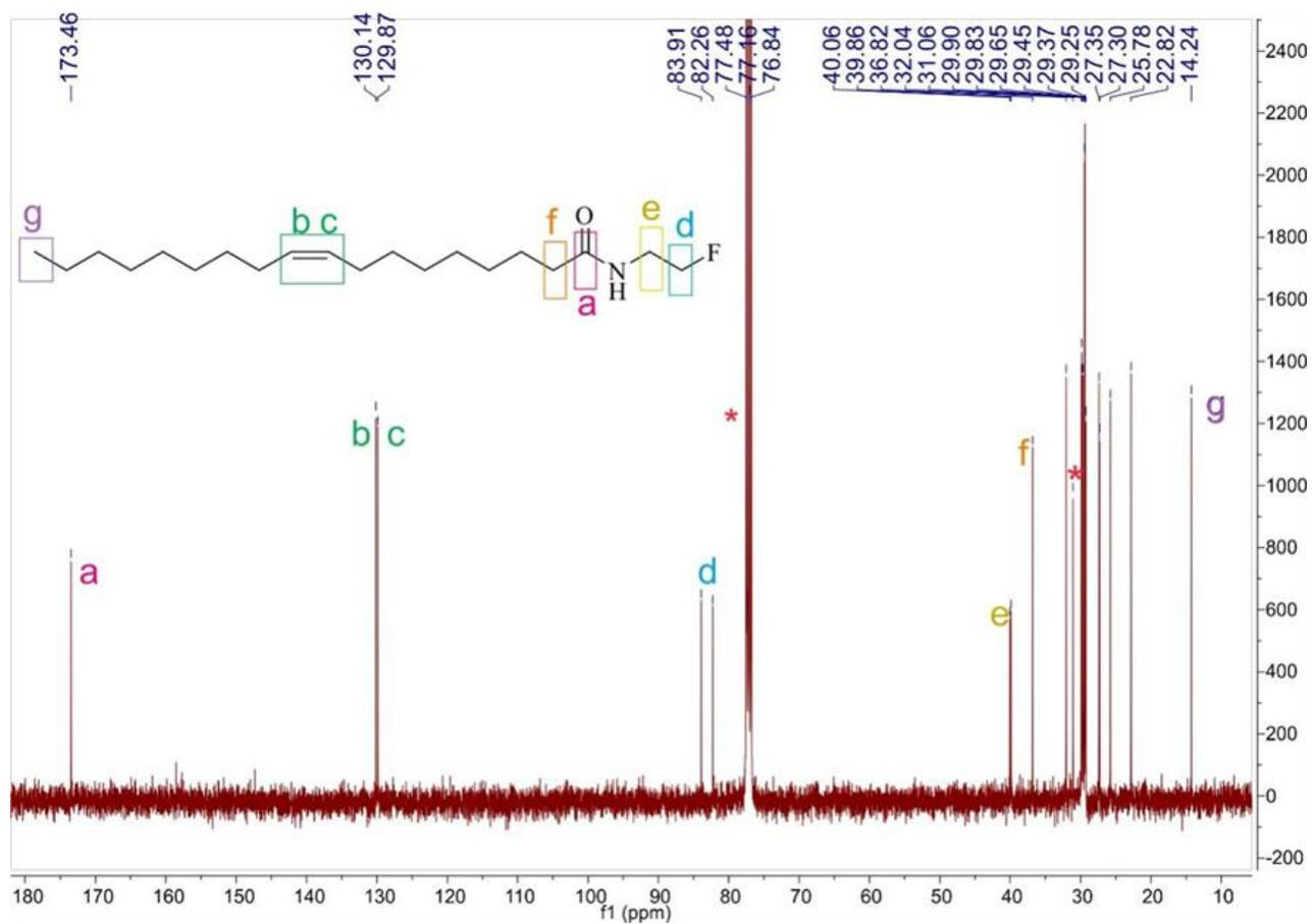
Figure 2.53. <sup>13</sup>C NMR spectrum of N-(2-fluoroethyl)oleamide.
