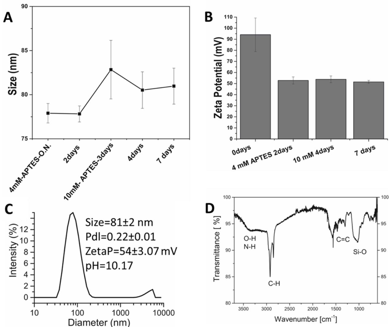
**Figure 3.13.** **A)** DLS measurements and **B)** Zeta Potential measurement of the reaction over time of TEOS silica-coated QS at 0 °C for 7 days. **C)** DLS measurements after 4 days of reaction the NB-QS-TEOS. **D)** IR spectra of silica-coated QS. The starting material has a size of  $84 \pm 1$  nm a Pdl of  $0.23 \pm 0.01$  and a Zeta Potential of  $84 \pm 2$  mV.
