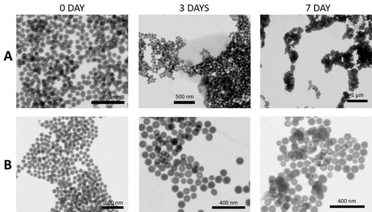
Figure 5.28. STEM pictures of the breakability test of A) Breakable NPs done with BTSPD 24% w/w with respect of TEOS and B) Non-breakable NPs.
