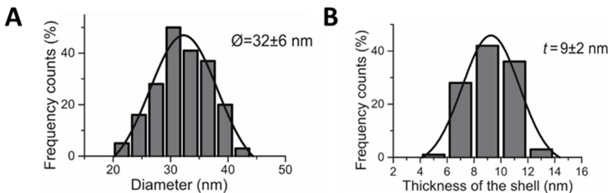
**Figure 3.33. A)** TEM size diameter distribution (count performed 200 silica-QS particles; average diameter  $32 \pm 6$  nm) and **B)** TEM size Thickness of the shell distribution (count performed in 100 silica-QS particles; average thickness of the shell  $9 \pm 2$  nm).
