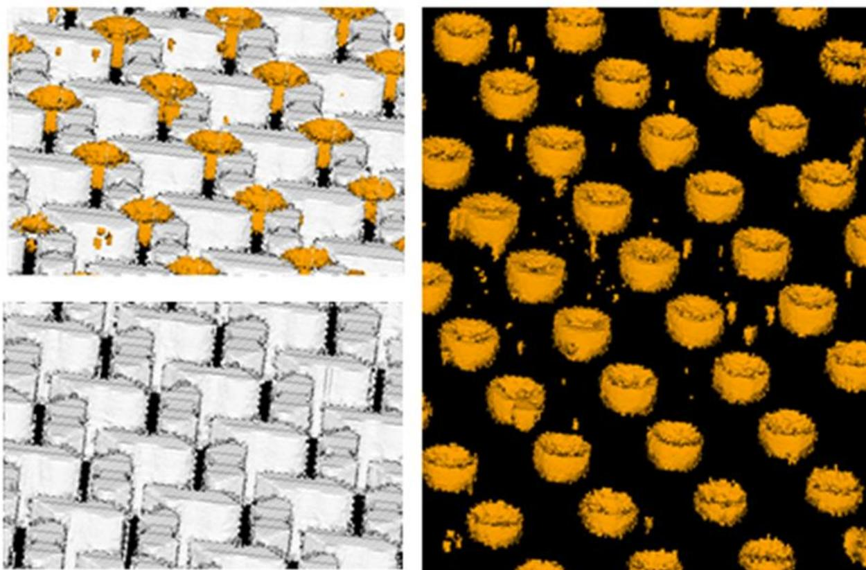
**Figure 2.46.** Z-stack analysis of the hydrogel filled by the polymer with NPs using 63x objective.
