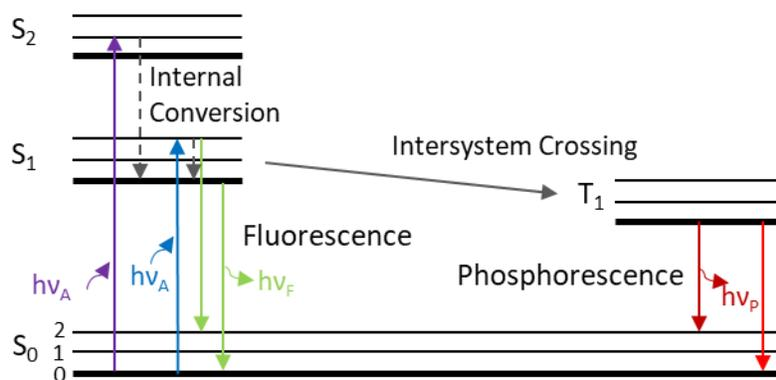
**Figure 4.1.** Jablonski diagram, fluorescence and phosphorescence phenomena.
