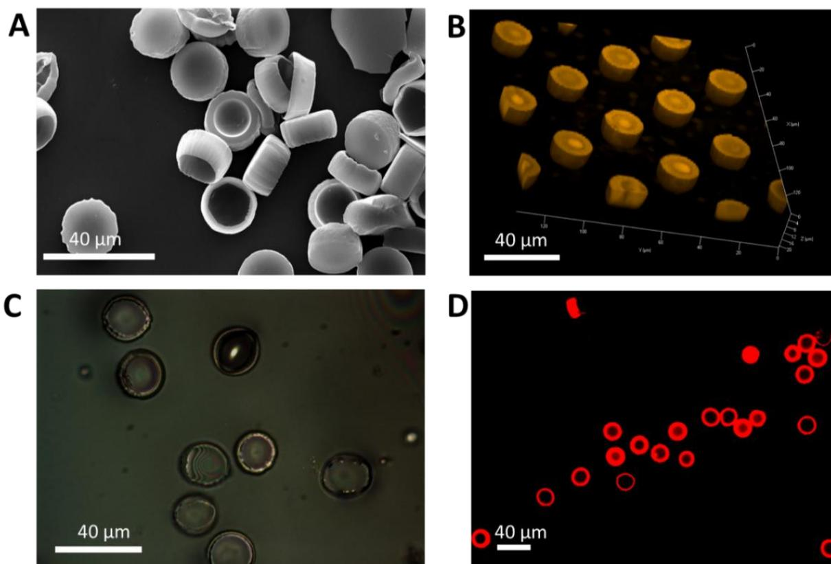
**Figure 2.35.** A) SEM image, B) Z-Stack confocal microscope image of the PLGA microspheres loaded with Nile Red using 63x objective C) and D) Light microscopy images.
