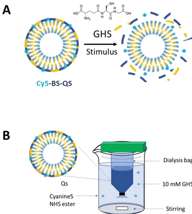
**Figure 4.12.** A) Schematic of the silica shell of the QS under the reducing agent glutathione (GSH) B) Experiment diagram for the breakability test (open system).
