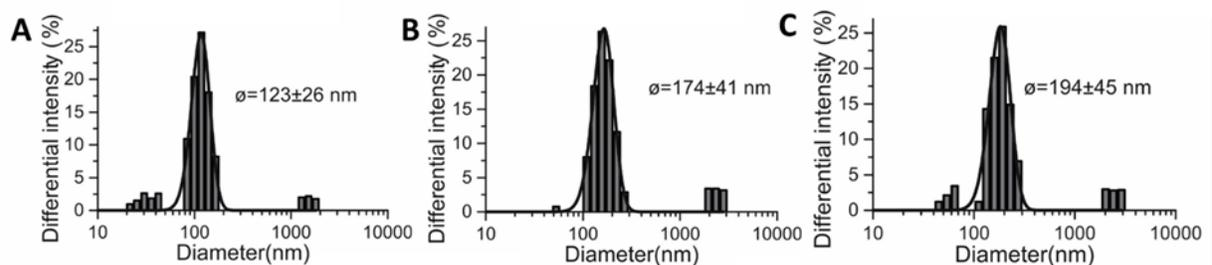
**Figure 3.10.** DLS measurements of the silica covered Quatsomes (SQS) **A)** after putting base (6 mM ammonia) and stirring during **B)** 1 h and **C)** overnight.
