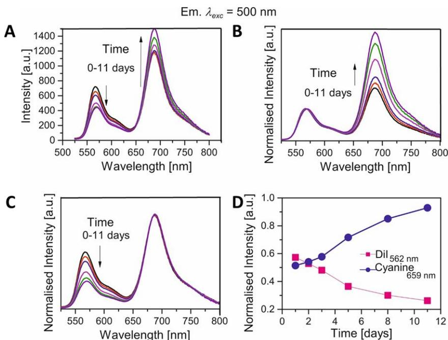
Figure 4.16. **A)** Emission spectra of Cy5-Breakable QS loaded with Dil after the time in the presence of 10 mM Glutathione. **B)** and **C)** Normalised Intensity of the Emission of Cy5-Breakable QS loaded with Dil normalised by the Dil and the Cy5, respectively. **D)** Normalised intensity of the emission at 562 and 659 nm representing the Dil and the Cyanine5.
