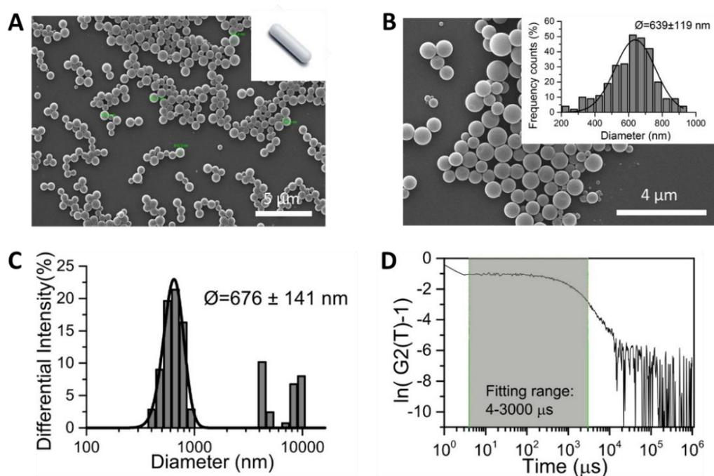
**Figure 2.25.** **A)** SEM image of the PLGA nanospheres using the SOAP methodology (scale bare 5  $\mu$ m). **B)** SEM size distribution (count performed on 300 particles: average diameter  $639 \pm 119$  nm). **C)** DLS result average diameter of  $676 \pm 141$  nm. Data obtained from the fitting range of 4-3000 of the **D)** autocorrelation function of the sample.
