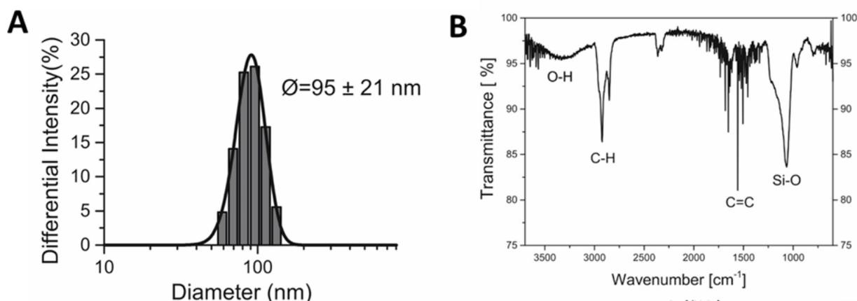
Figure 3.40. A) DLS measurement and B) IR spectra of the B-SQS.
