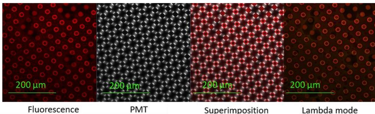
**Figure 2.39.** Confocal microscope images of the hydrogel filled by AEA-PLGA@MBds using 10x objective (scale bar 200μm).
