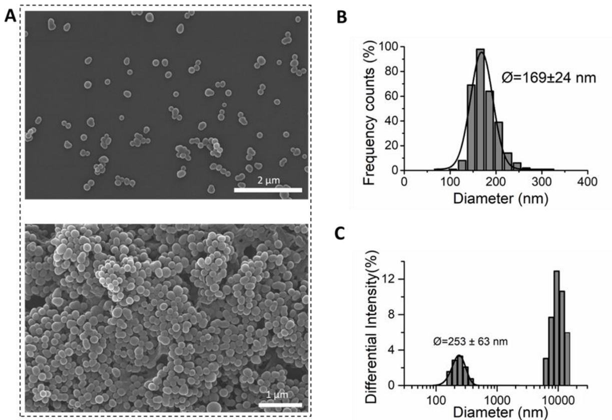
**Figure 5.21.** A) SEM pictures of Breakable NPs prepared with a non-toxic surfactant (MKC) and Stöber methodology. B) SEM counting of 300 NPs (size distribution  $169 \pm 24$  nm) C) DLS distribution  $253 \pm 63$  nm.
