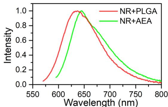
**Figure 2.41.** Emission spectra of NR in PLGA and NR with AEA using a fluorimeter.
