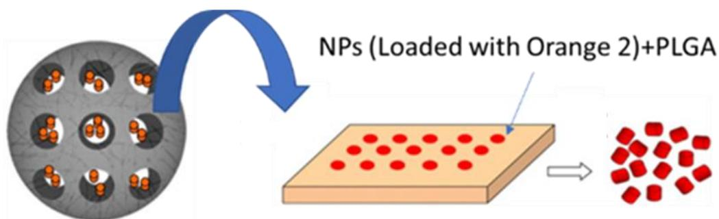
**Scheme 2.13.** Representation of the loading of NPs in the PLGA@MBds by the hydrogel template method.
