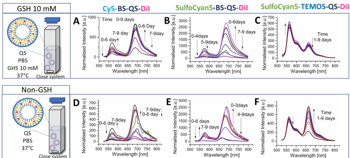
**Figure 4.27.** Emission (excitation wavelength 500 nm) for the Cy5-BS-QS-Dil, Sulfo-Cyan5-BS-QS-Dil, and Sulfo-Cyan5-TEMOS-QS-Dil in presence of GSH **A**), **B**) and **C**); and with non-GSH **D**), **E**) and **F**), respectively.
