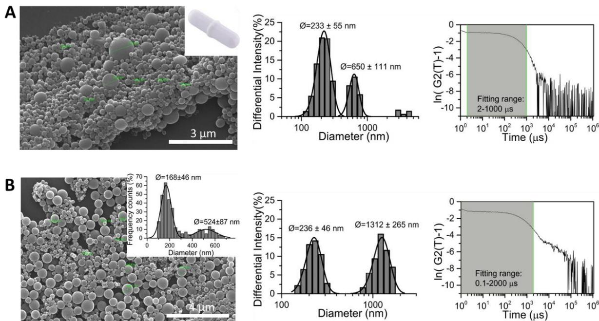
**Figure 2.28.** Experiments to produce the PLGA- spheres by the SORP methodology changing the stirring bar for one with a pivot ring . SEM and DLS results average diameter show two different populations: first synthesis **A)** size diameter of  $233 \pm 55$  nm and  $650 \pm 111$  nm; second synthesis **B)** size diameter of  $236 \pm 46$  nm and  $1312 \pm 265$  nm.
