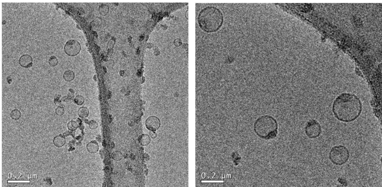
**Figure 3.22.** Cryo-TEM images of 10% silica-coated Dodecyl silane QS. Scale bar 0.2  $\mu\text{m}$ .
