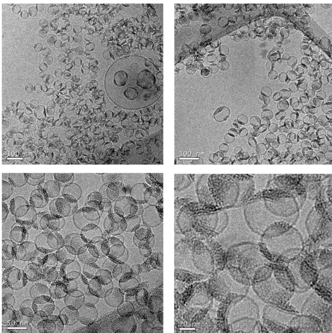
**Figure 3.15.** Cryo-TEM images of the 10 mM TEOS silica-coated QS at 0 °C after dialysis. Scale bars, 100, 50 and 20 nm.
