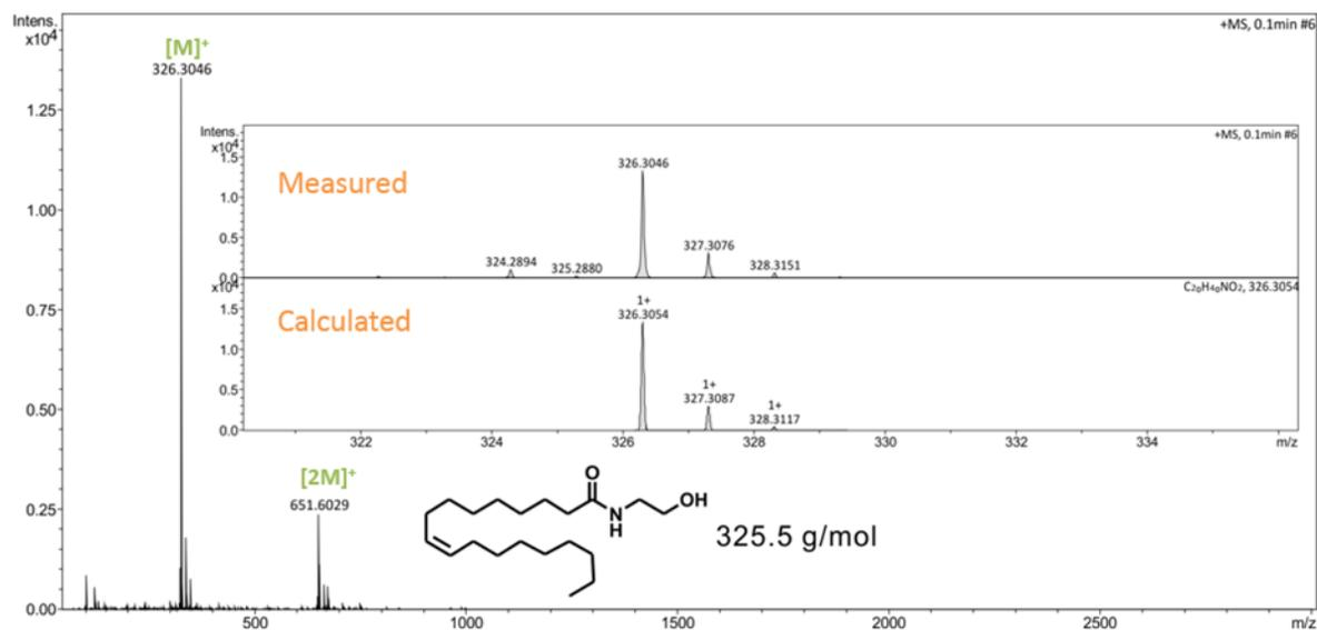
Figure 2.62. HR ESI-TOF-MS spectra of *N*-(2-hydroxy ethyl) oleamide.
