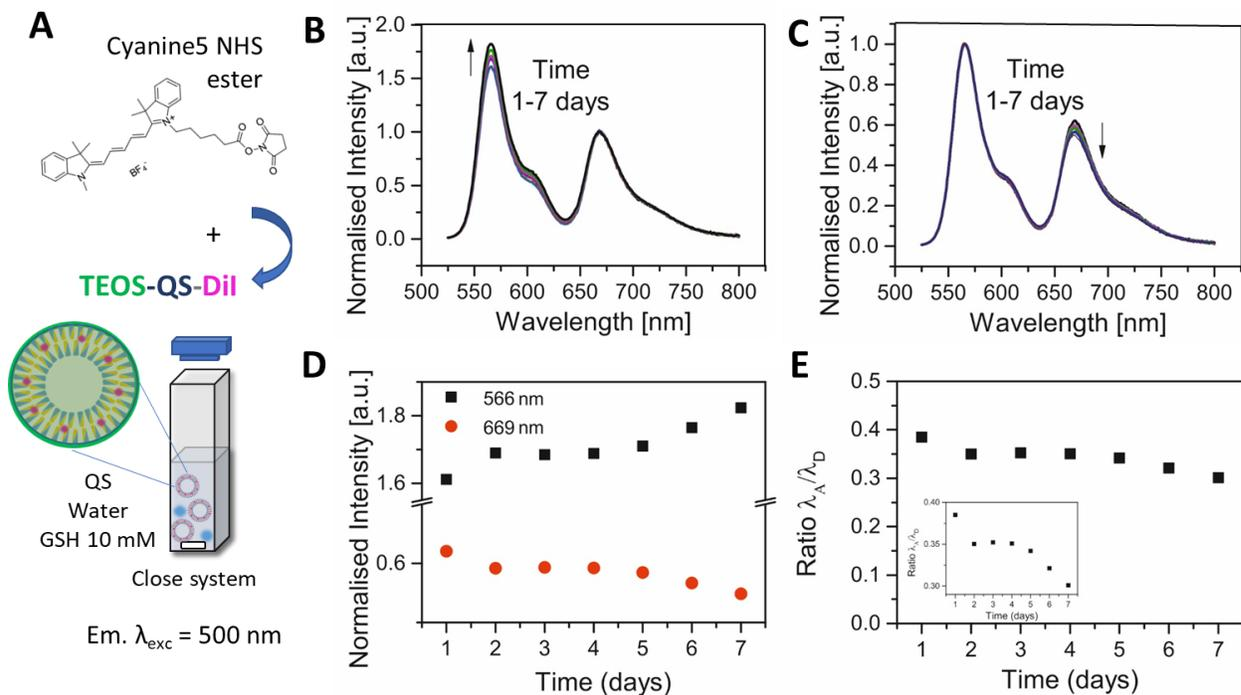
**Figure 4.22.** **A**) Experiment diagram for the permeability test using TEOS-QS-Dil (non-breakable). **B**) and **C**) Normalised Intensity of the Emission of the TEOS-QS-Dil; normalised by the Cyanine5 and the Dil band, respectively. **D**) Normalised intensity of the emission at 566 and 669 nm representing the Dil and the Cyanine5. **E**) Ratio Acceptor/Donor of the sample after 7 days.
