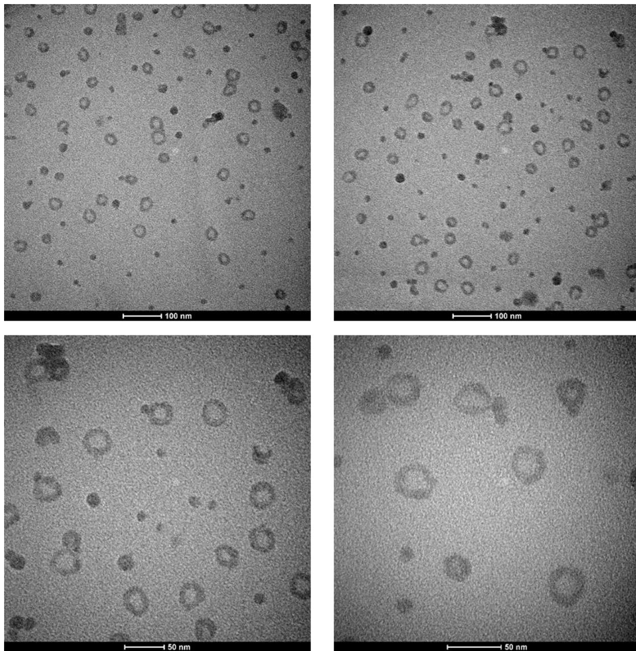
Figure 3.32. TEM images of breakable silica-coated QS (APTES+BTSPD). Scale bar 100 and 50 nm.
