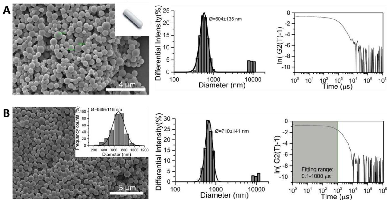
**Figure 2.27.** A) Second and B) Third repetition of the PLGA- spheres done by the SORP methodology. SEM and DLS result average diameter of  $604 \pm 135$  nm and  $710 \pm 141$  nm, respectively.
