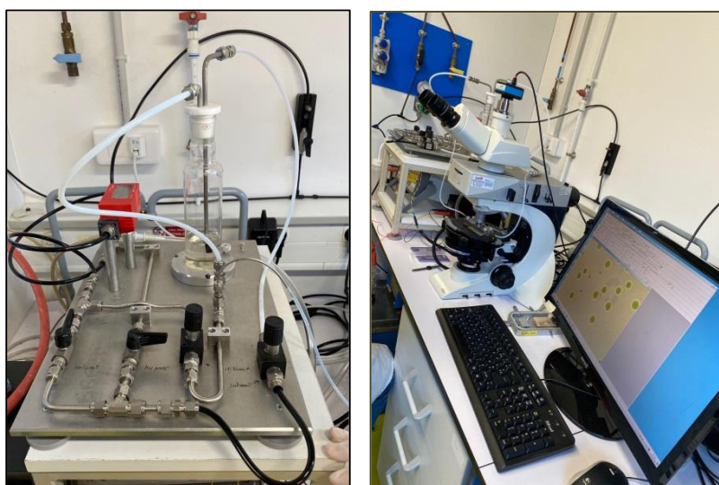
Figure V. 2 Solvent vapor annealing setup connected to an optical microscope and a Keithley machine.
