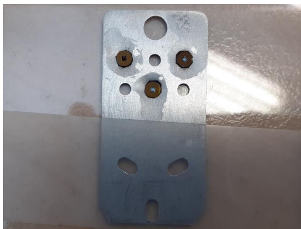
Figure 3.4: Sample holder with glued TEM grid.
