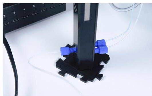
MUX-wire configuration for flow to waste. 3/2 valve "N.C." (closed)
