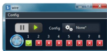
MUX-wire configuration for flow to waste. 3/2 valve "N.C." (closed)
