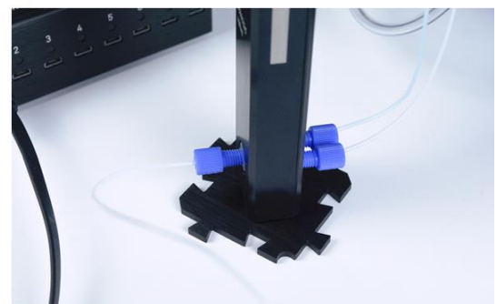
MUX-wire configuration for flow to waste. 3/2 valve "N.C." (closed)
