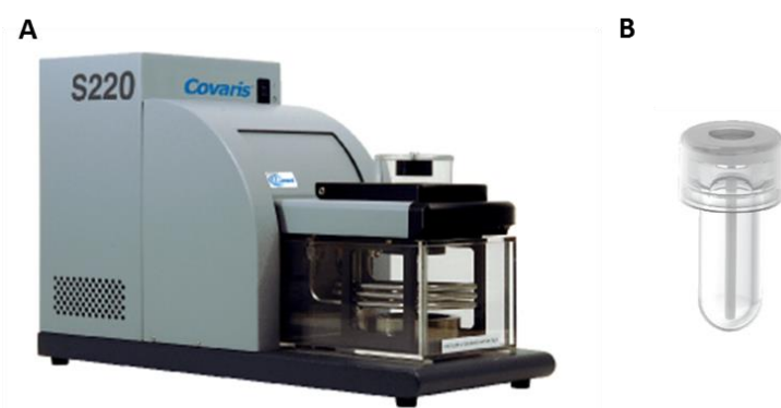
Figure 79: Presentation of the system used for the experiments. Covaris S220 Focused-ultrasonicator (A). MicroTUBE AFA Fiber Pre-Slit Snap-Cap 6x16mm (B).
