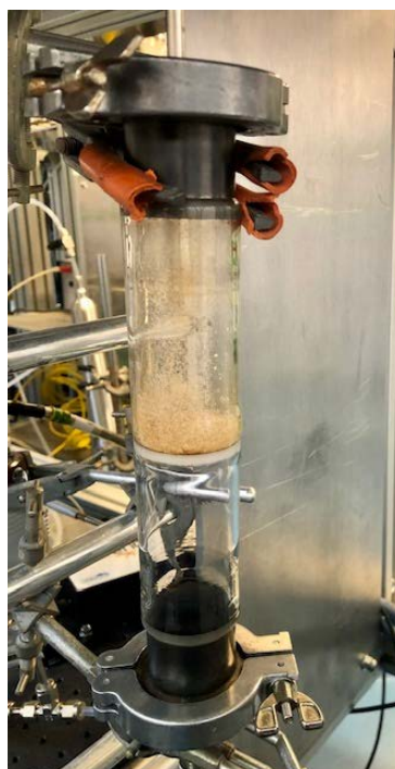
Figure 2.4.1: Precursor/ICN vessel, fitted with a glass frit, used to flow in the precursor with a buffer gas flowing in from the top.
