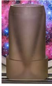
(a) Picture of a 3-D printed Laval nozzle which provides a temperature of 10 K with He as buffer gas.
