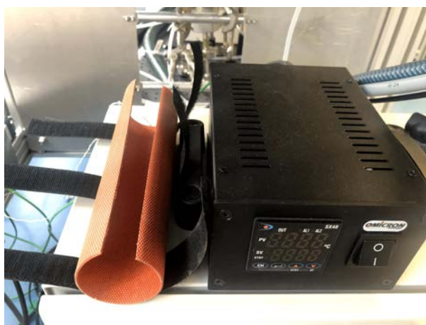
Figure 2.4.4: The heating pad apparatus used with the ICN vessel along with the controller.
