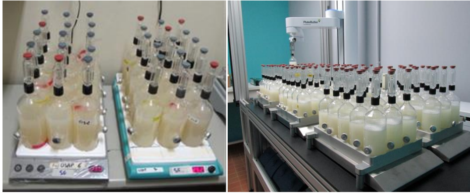
Figure 17: Experimental layout of small scale wine fermentations with tracking of fermentation kinetics by hand (left) and using a custom-built robot (right).
