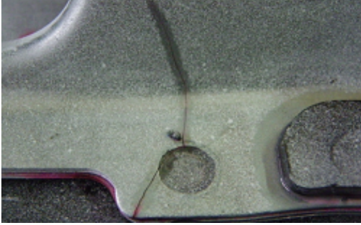
Figure 4.1: Example of critical zone on a cradle model under longitudinal solicitations. The picture on the left represents the zone on the sixth specimen tested. The figure on the right represents the severity (multiplicative coefficient of the client objective F_n ) of the seven tests performed. Only two (the red ones) resulted into a crack initiation.
