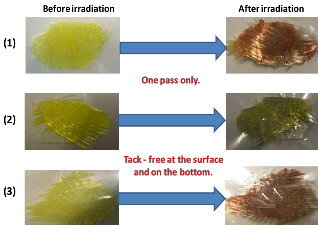
Figure 6. Photocomposites produced upon exposure to near-UV light (LED@395 nm), belt speed = 2 m/min, using free radical polymerization (FRP) in the presence of glass fibers/acrylate resin for different systems: (1) PT2/Iod/NPG (0.1%/1%/1% w/w/w); (2) PT4/Iod/NPG (0.1%/1%/1% w/w/w); and (3) PT2/Iod/NPG (0.1%/1%/1%) in TMPTA.
