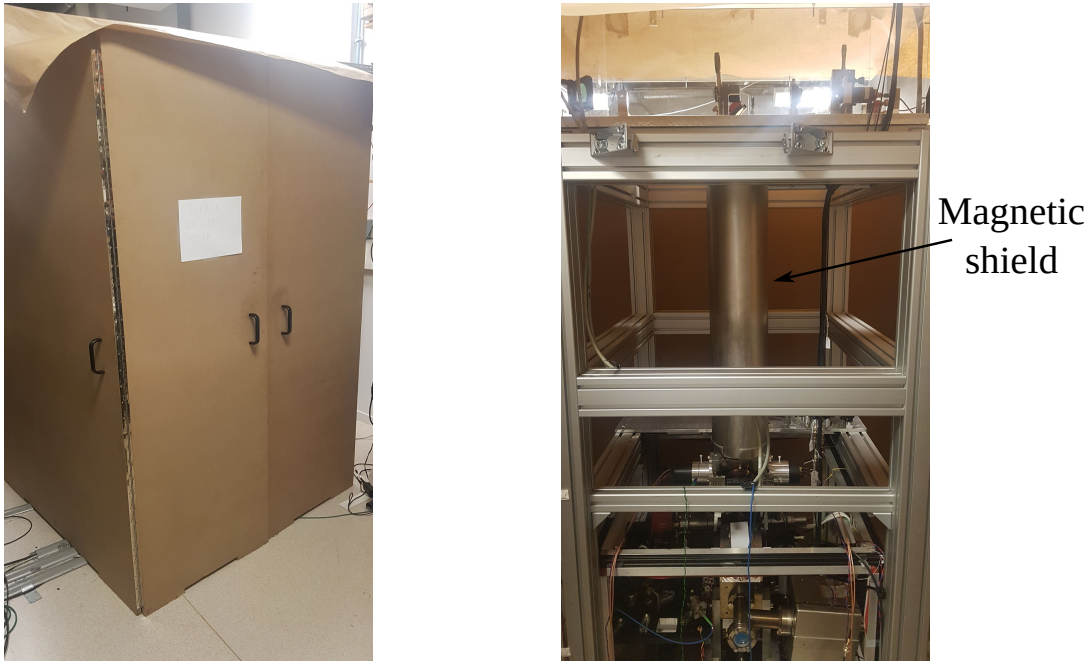
Figure 3.1: Left: Wood panel box protecting the experiment from the environment perturbation. Right: \mu – metal magnetic shield for the interferometer tube
