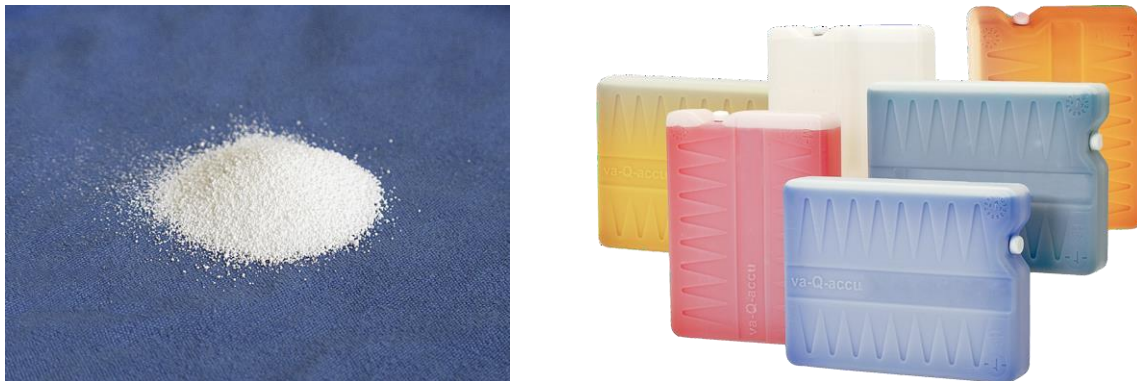
Figure 13: Micro [71] et macro [72] capsules de PCM.
