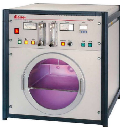
Figure 4.13: The O 2 plasma cleaner system by DIENER Nano is used in this thesis. The sample is placed on a large carrier into the box. Active oxygen plasma then fill the box and clean the surface of the sample.
