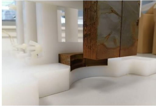
Figure III.13. View of the end-parts of the cut pieces no.1 and 2 obtained from the delivered closed magnetizing circuits for the 90° configuration of the demonstrator.
