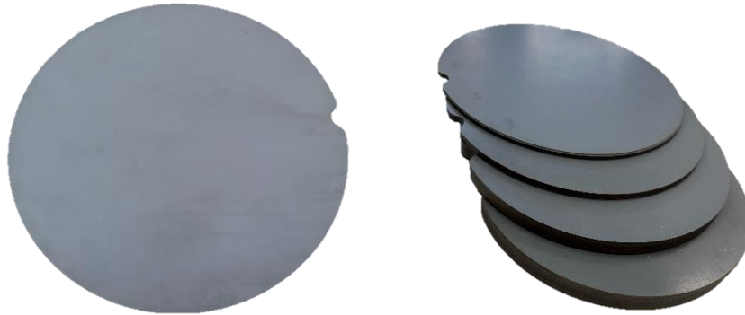
Figure III.8. Photos of the cut disks and the sets of laminations constituting the stack of interest.
