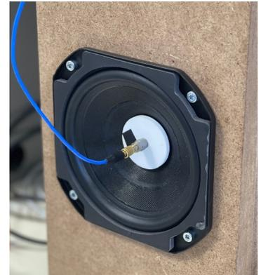
(b) Fatial Pro 5FE100 with accelerometer.
