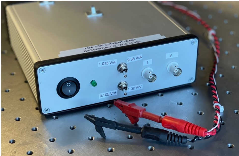
FIGURE E.3 – Voltage/Current sensing system
