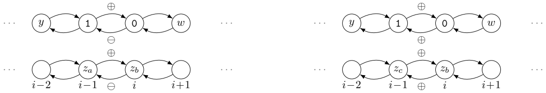
Figure A.19 – On the left, starting from a configuration (y, 1, 0, w) , the schedule \Delta updates the cell i before cell i - 1 . Therefore, the cell i becomes z_b = r_{44}(1, 0, w) , and the cell i - 1 is updated to z_a = r_{44}(y, 1, z_b) . On the right, according to \Delta' , the cells i and i - 1 are updated at the same time. Therefore, z_c is equal to r_{44}(y, 1, 0) and z_b is equal to r_{44}(1, 0, w) .
