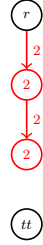
Figure 5.9 – The SB-MDD (before reduction) for C_2^1 \odot \overset{\circ}{X} = C_4^5 . The red part will be deleted by the pReduction algorithm.
