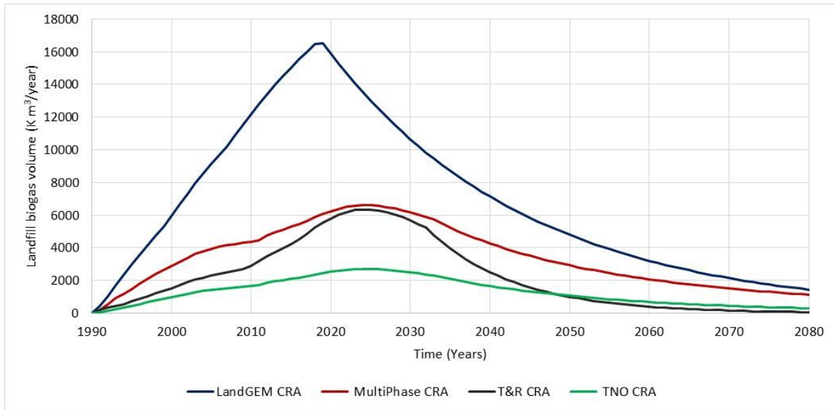
Figure 2-4: LFG generation obtained by CRA method with different models at L_0 = 115.7 and k = 0.04
