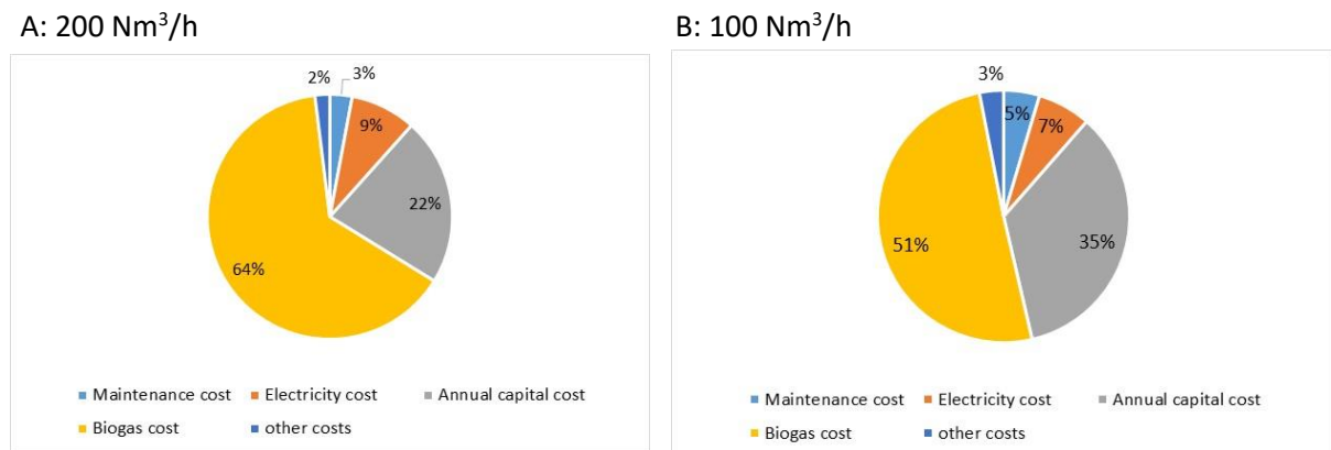
Figure 3-11: Share of cost items in the specific cost of biomethane production with water scrubbing at biogas flow rate A: 200 Nm 3 /h and B: 100 Nm 3 /h
