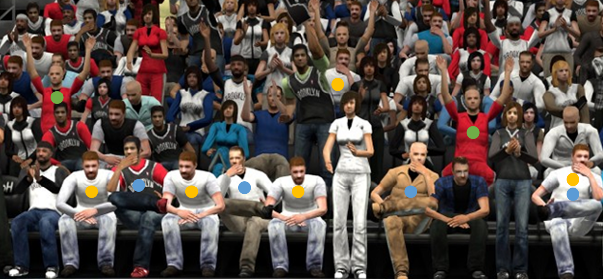
Figure 1.1: Typical crowd from the NBA 2k14 Video Game. Yellow dots correspond to Appearance Clones i.e. characters with similar clothes and character model. Blue dots correspond to Motion Clones, i.e. characters sharing the same animation. Green dots show clones that share both motion and appearance.
