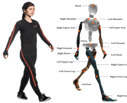
Figure 3.1: Xsens Motion Capture system used to record the motion of our actors. The system consists in 17 IMU based sensors (right) placed within a motion capture suit (left). Each sensor is composed of accelerometers and gyroscopes. Figure taken from http://www.xsens.com .
