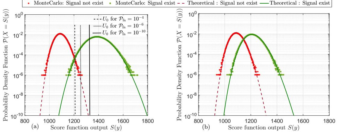
Figure 4.7 – MC and Theoretical PDFs in both hypothesis  $\mathcal{H}_0$  and  $\mathcal{H}_1$ , for a CCSK frame of  $N=20$  symbols in  $\text{GF}(64)$  for the first scenario (a)  $\text{SNR} = -10$  dB,  $\Delta = 0$ , no frequency offset and for the second scenario (b)  $\text{SNR} = -10$  dB,  $\Delta = 16$ ,  $\theta_\delta = \pi/2$ .
