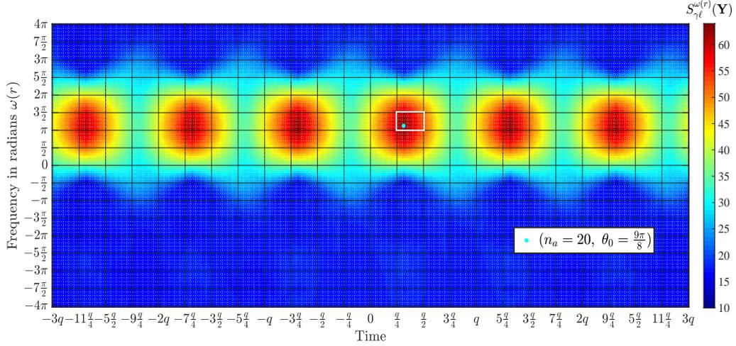
Figure 4.5 – Values of  $\mathbf{S}_{\gamma\ell}^{\omega(r)}(\mathbf{Y})$  for an arriving QCSP frame in a noiseless channel.
