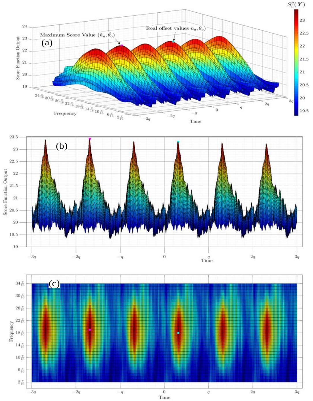
Figure 5.2 – Values of  $S_n^\theta(\mathbf{y})$  for an arriving QCSP frame in a very Low SNR channel, with  $n \in [n_a - 3q, n_a + 3q]$  and  $\theta \in [\theta_o - \frac{\pi}{4}, \theta_o + \frac{\pi}{4}]$ .
