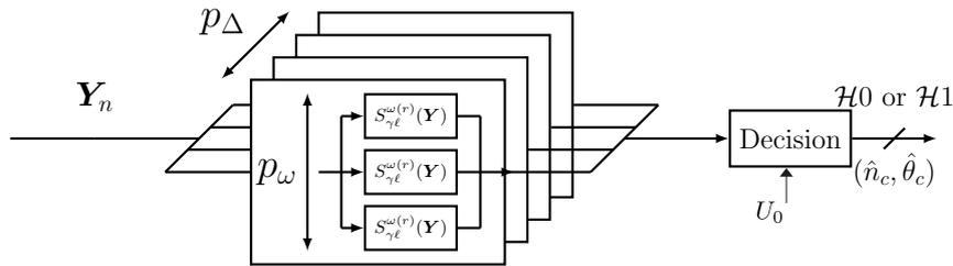
Figure 4.4 – Complete theoretical detection system.
