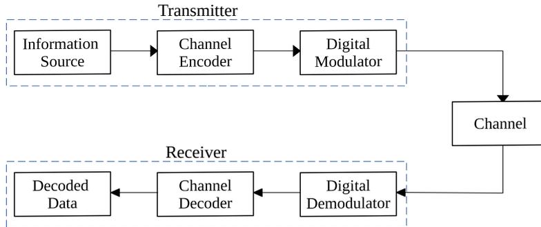
Figure 2.2 – The transmission system model.
