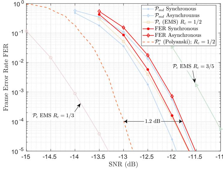
Figure 6.3 – Joint FER due to  $\mathcal{P}_\epsilon$ ,  $\mathcal{P}_{\text{md}}$  and to  $\mathcal{P}_{\text{fa}} = 10^{-6}$  for  $N = 120$  symbols, where  $R_c = 1/2$ , in synchronous and asynchronous CAWGN channel.
