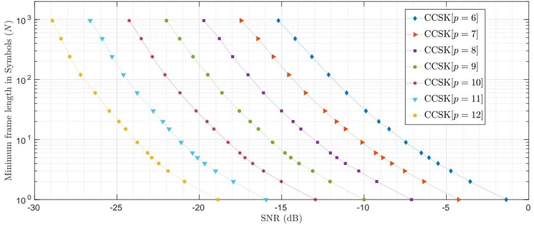
(a) CCSK frame length in Symbols  $N$ .
