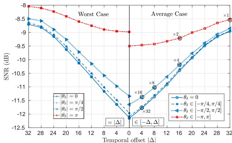
Figure 4.10 – Minimum SNR required as function of different  $\Delta$  and  $\theta_\delta$  values, for defined probabilities ( $\mathcal{P}_{fa} = 10^{-6}$  and  $\mathcal{P}_{md} = 10^{-4}$ ), in a CCSK frame of  $N = 120$  and order  $p = 6$ .
