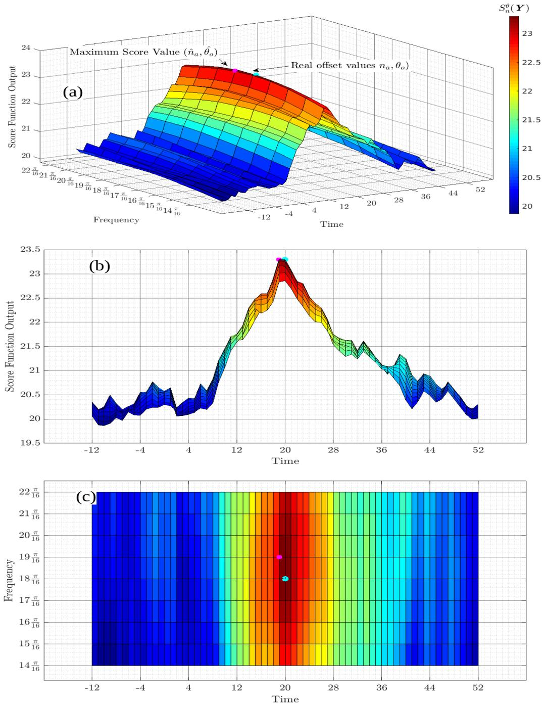
Figure 5.3 – Values of  $S_n^\theta(\mathbf{y})$  for an arriving QCSP frame in a very Low SNR channel, with  $n \in [n_a - q/2, n_a + q/2]$  and  $\theta \in [\theta_o - \frac{\pi}{4}, \theta_o + \frac{\pi}{4}]$ .
