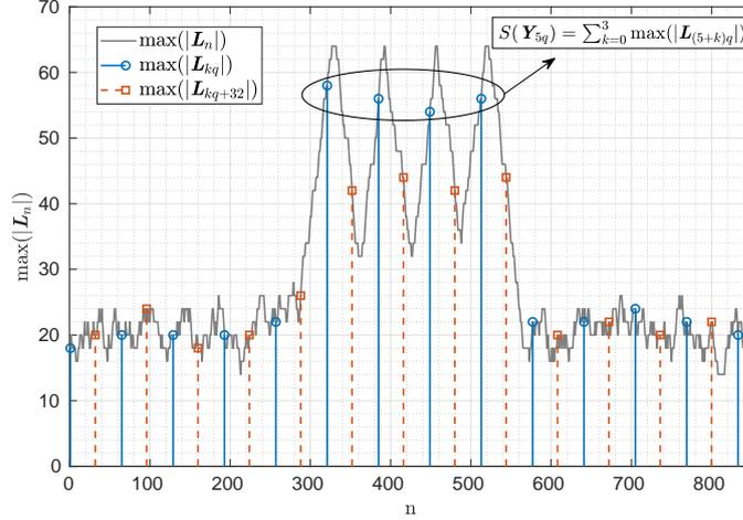
Figure 4.3 – Example of the score function calculation for a CCSK frame of size  $N = 4$ ,  $q = 64$  starting at time  $n_a = 327 = 5q + \Delta$ , where  $\Delta = 7$ . Random bits are assumed to be transmitted before and after the CCSK frame.
