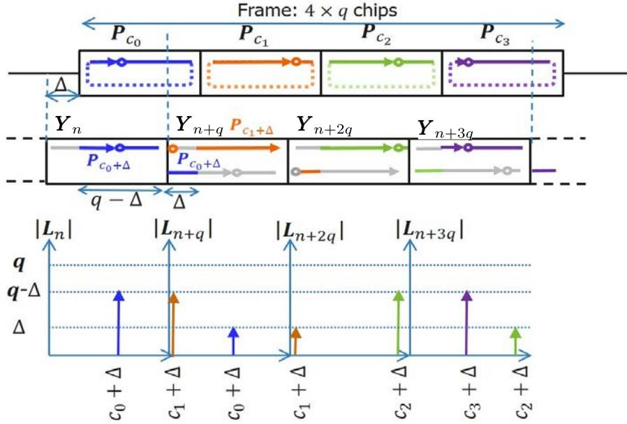
Figure 4.2 – Illustration of the frame detection principle.
