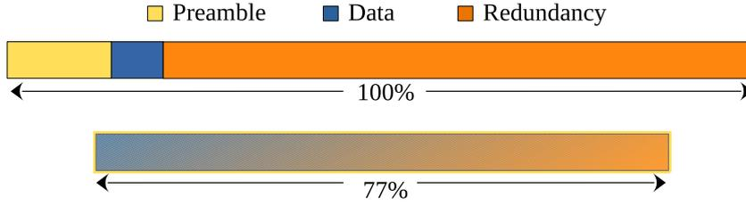
Figure 6.4 – Classical vs. preamble-less proposed approach (QCSP) for transmitting a frame.
