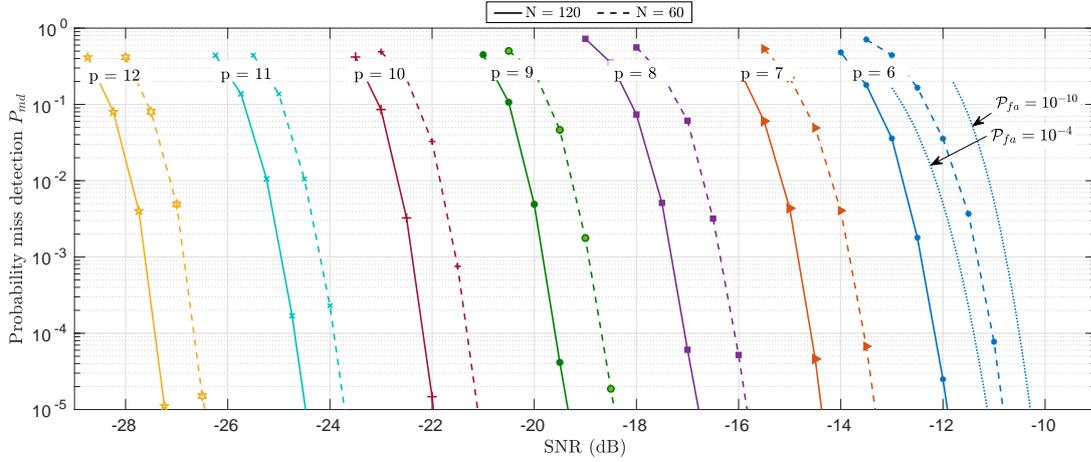
Figure 4.8 –  $\mathcal{P}_{\text{md}}$  and  $\mathcal{P}_{\text{fa}}$  as function of SNR for a CCSK frame of  $N = 60, 120$  symbols for different  $q = 2^p$  orders, in an ideally synchronized channel.
