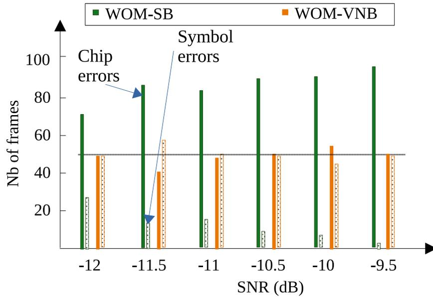
Figure 5.16 – Type of the time synchronization errors: at chip level or symbol level.
