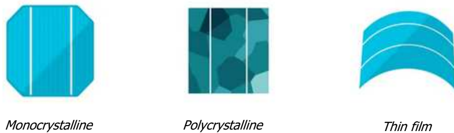
Figure 1.5.: The main types of the PV cell [1].
