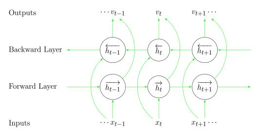
Figure 3.16: Bidirectional LSTM
