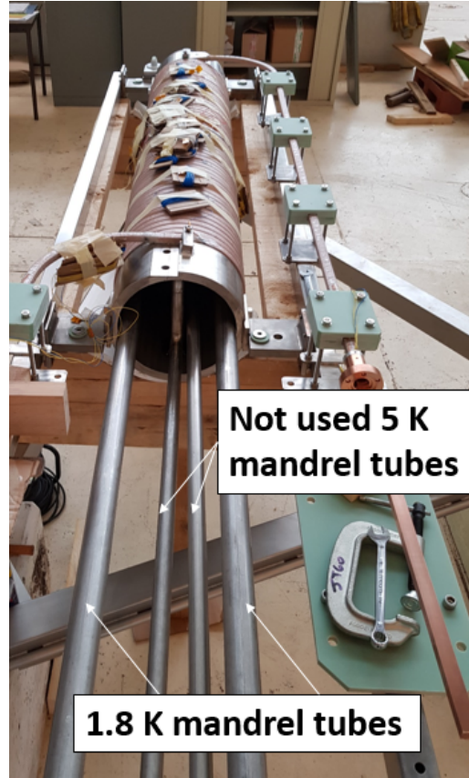
Figure 3.16: Picture of the mandrel tubes filled with the superfluid helium, on the left and right sides. The tubes are installed to help the center of the magnet to cool down. With the courtesy of Théophile Pontarollo for the picture.
