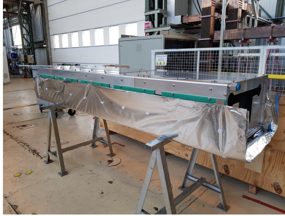
Figure 3.19: Picture of the thermal shield, at the beginning of the MLI laying. The front face of the shield allows to hydraulically and electrically supply the magnet. At the back, the back and forth cooling tubes can be seen.
