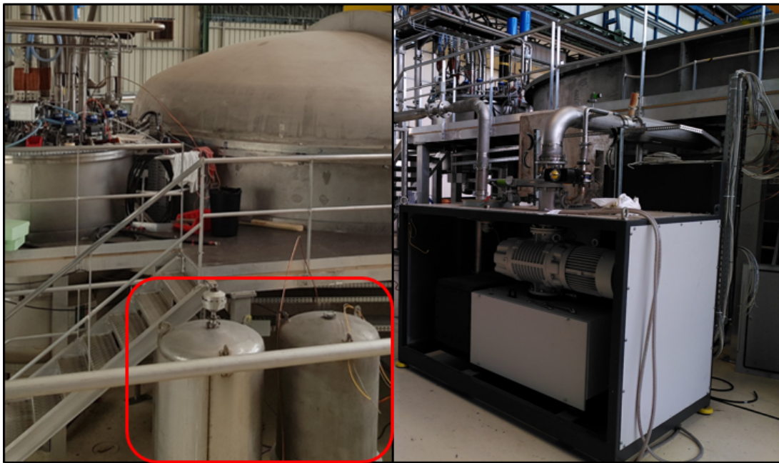
Figure 3.15: Picture of the pressurized and vacuum tank on the left and picture of the pumping group on the right.
