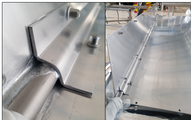
Figure 3.18: Picture of improved thermal contact between the tubes and the shield, all along the shield length.
