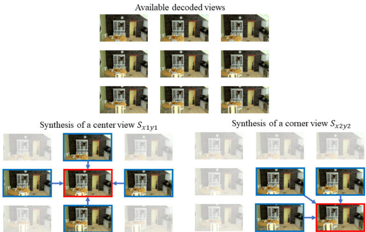
Figure 2.16 – Objective evaluation: allowed reference views (blue) to be used to synthesize a target view (red) at source position.
