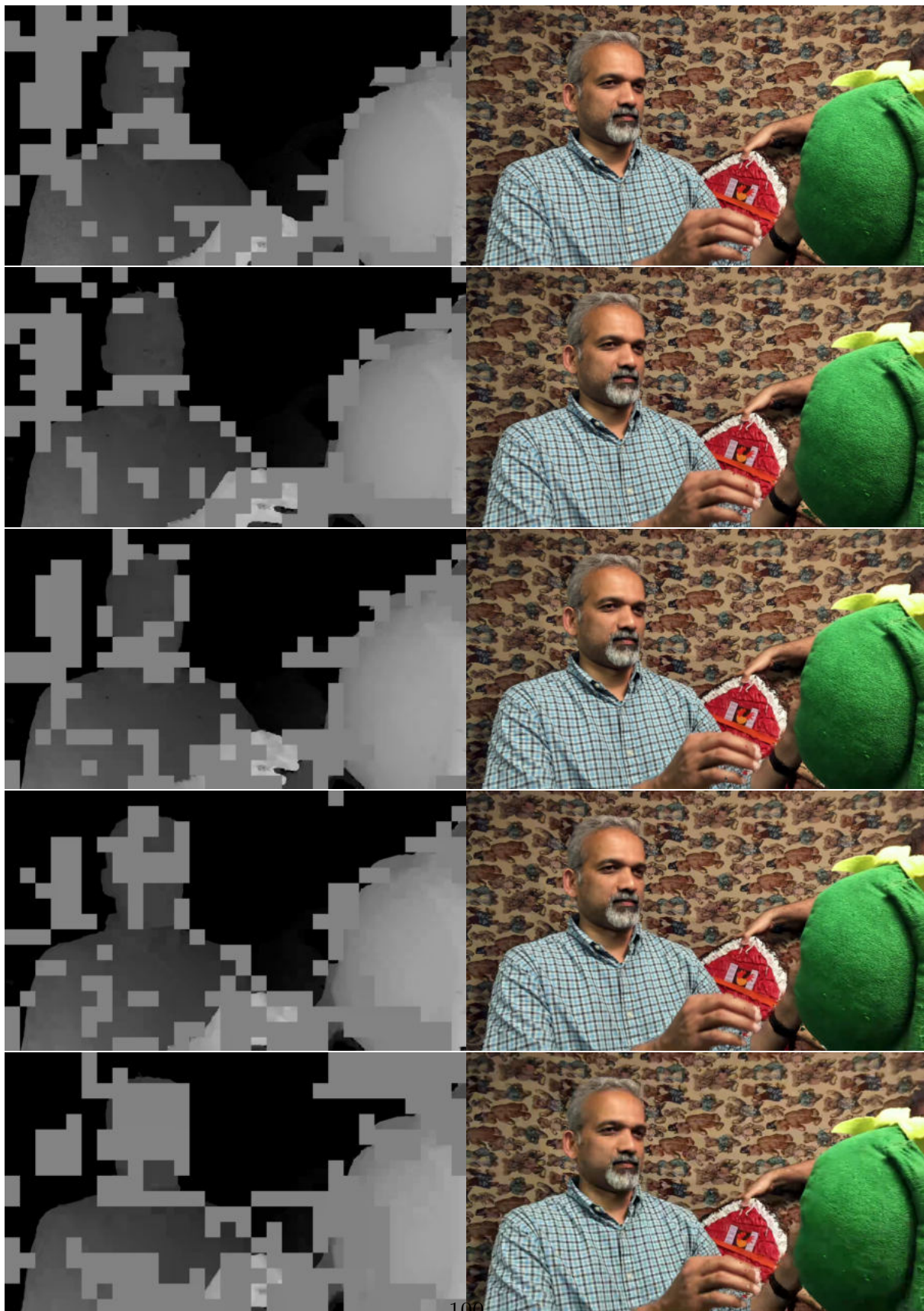
Figure 4.5 – Evolution of H-DSDE selection (left) and corresponding view synthesis quality (right) with falling bitrate for natural content (Frog sequence). The grey blocks indicate omitted depth CTUs, which have to be recovered at the decoder side.
