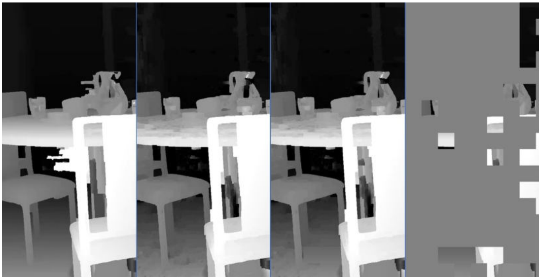
Figure 4.2 – Example for different depth signals in the H-DSDE system. From left to right: source depth ( D ), DSDE depth ( D^+ ), hybrid depth ( D_H ), decoded partial depth ( D_{part}^* ).
