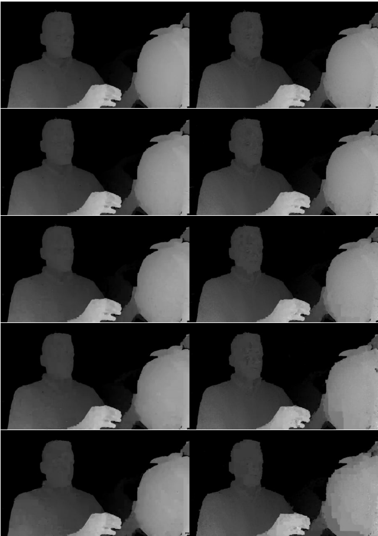
Figure 3.3 – Evolution of depth map quality for ESDE (left) and DSDE (right) from high bitrate (top) to low bitrate (bottom) for natural content (Frog sequence).
