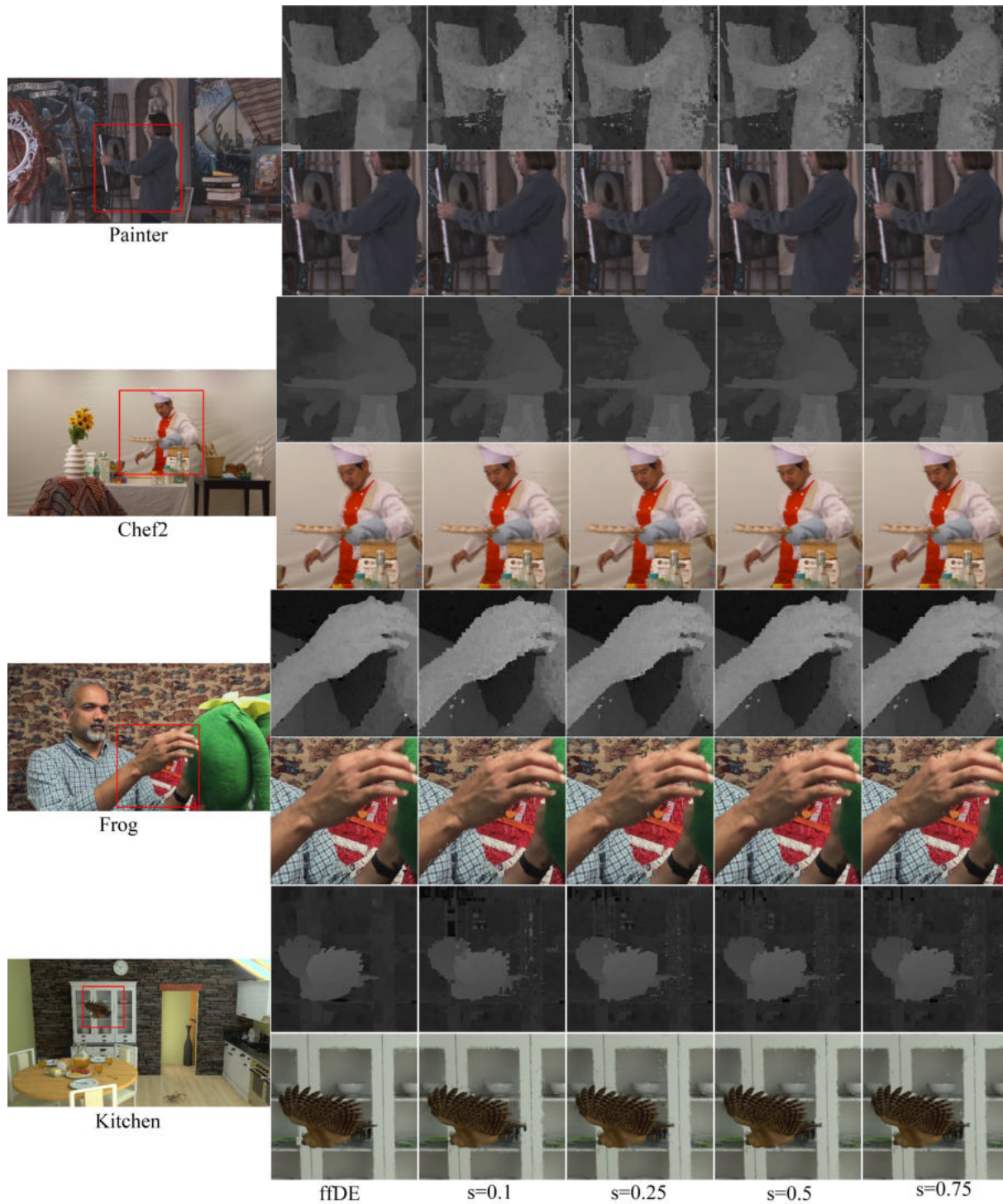
Figure 7.14 – Depth maps and synthesized view of two sequences. Frame 16 is shown for the unmodified reference in the B-DSDE system using ffDE as well as the MC-DSDE proposal for different thresholds.
