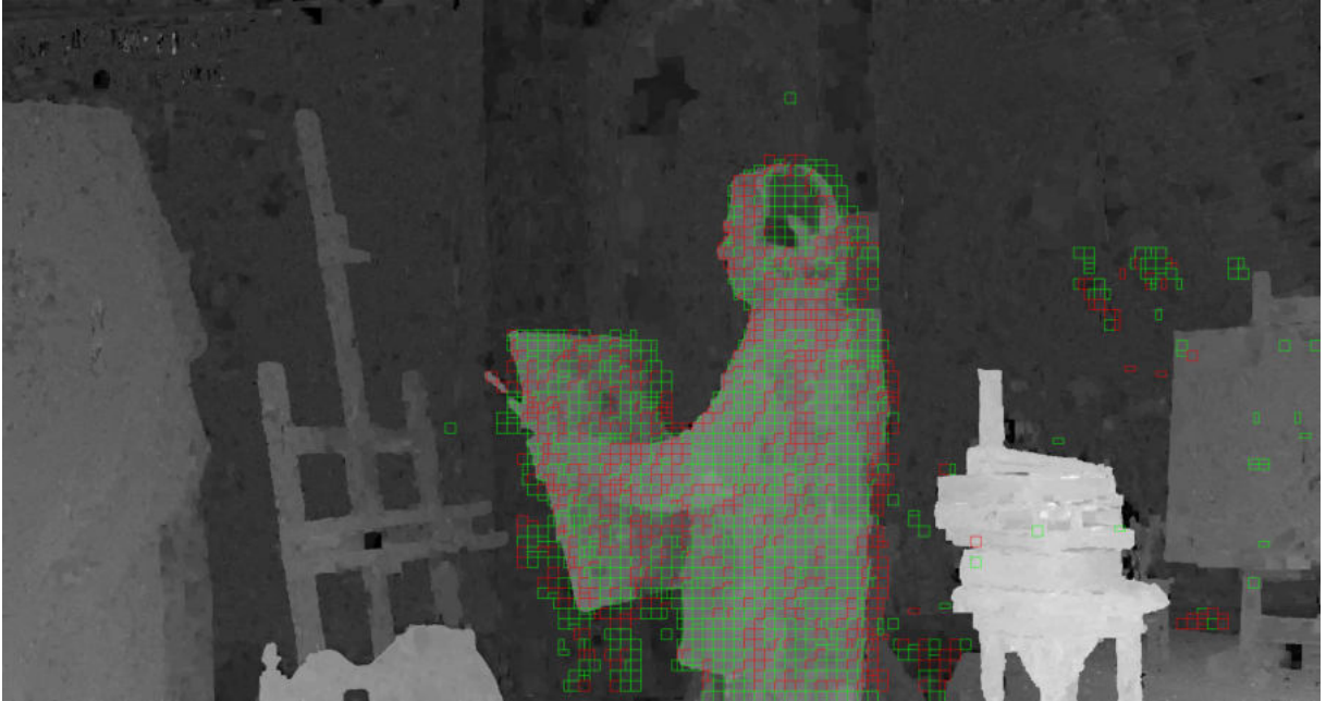
Figure 7.3 – Example for identified Prediction Units with non-zero motion information. Green blocks are motion compensated, while red blocks are estimated using the block-based DERS8 (case s = 0.25 , Painter sequence).
