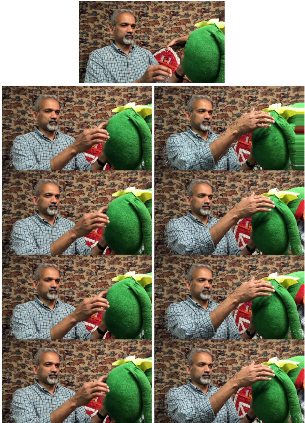
175 Figure 7.13 – Frog Sequence. Top: frame 0, synthesized using depth maps estimated by the unmodified DERS8. left: Frame 8. Right: Frame 16. From top to bottom: increasing threshold s , from 0.1 to 0.75
