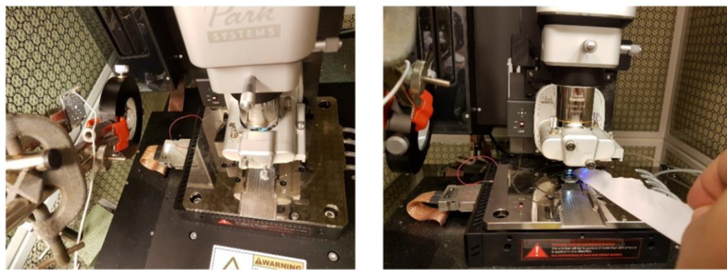
Figure 56 : KPFM measurement setup with the LED and an added lens between the LED and the sample.
