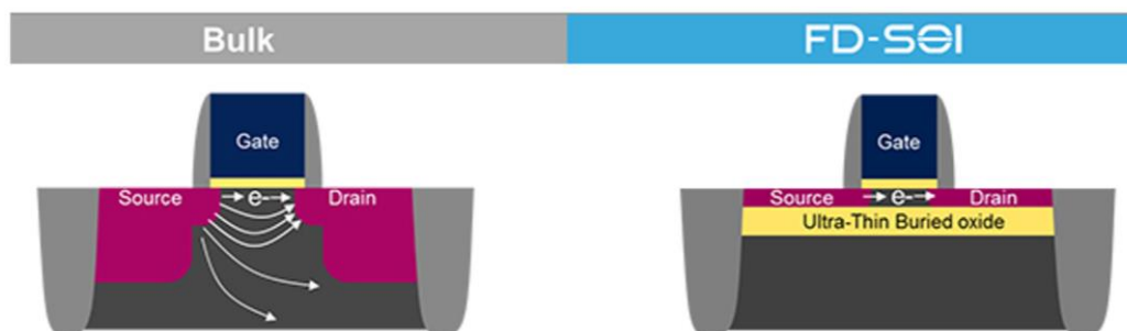
Figure 10 : Bulk MOS structure (left) versus fully depleted SOI (FD-SOI) structure (right). The electrons flowing from the source to the drain are confined in the channel region in the latter case thanks to the presence of the buried oxide layer (BOX). 48
