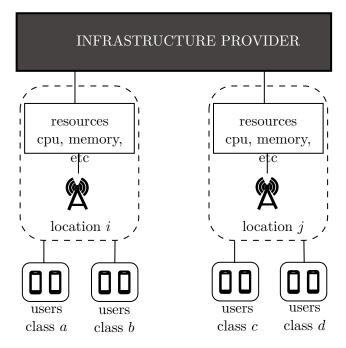
Figure 3.2 – System description: topological view.
