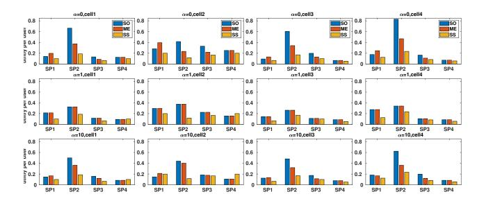
Figure 3.4 – Bar graphs describe the utilities (service rate) under Socially optimal allocation (SO), market equilibrium (ME) and Static proportional (SS) allocation scheme attained by the users associated with the service providers SP1, SP2, SP3 and SP4 in the cell 1-4, when  $\alpha$  fairness criteria with  $\alpha = 0$ ,  $\alpha = 1$  and  $\alpha = 10$  applied by the service providers.
