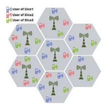
Fig. 1. Resource Slicing in 5G Networks: slices are assigned radio resources on a per-cell basis.
