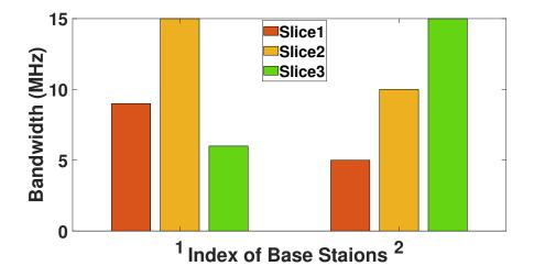
Figure 2.6 – Allocation of bandwidth among the slices at base station 1 and 2.
