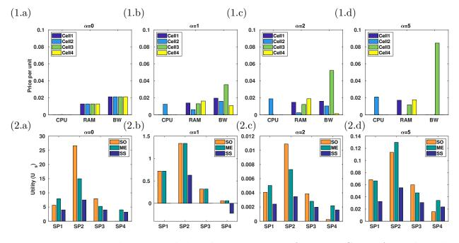
Figure 3.5 – Bar graphs 1. a to 1.d show the price per unit of resources CPU, RAM and Bandwidth (BW) at cells 1 to 4 when alpha fairness criteria with  $\alpha = 0, 1, 2$  and 5 applied by the service providers. Each bar graph from 2. a to 2.d describe the total utility achieved by the SPs under optimal social allocation (SO), market equilibrium (ME) allocation, and static proportional allocation (SS) when  $\alpha$  fairness with  $\alpha = 0, 1, 2$  and 5 applied by the SPs.
