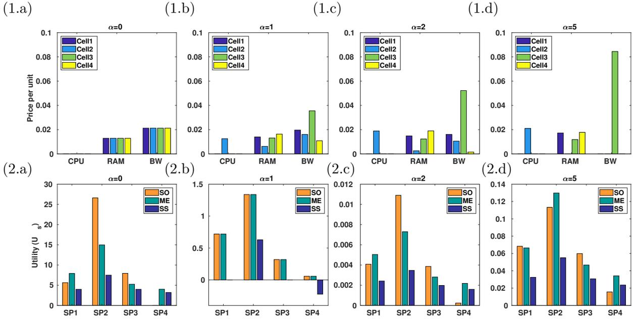
Figure 3.5 – Bar graphs 1. a to 1.d show the price per unit of resources CPU, RAM and Bandwidth (BW) at cells 1 to 4 when alpha fairness criteria with  $\alpha = 0, 1, 2$  and  $5$  applied by the service providers. Each bar graph from 2. a to 2.d describe the total utility achieved by the SPs under optimal social allocation (SO), market equilibrium (ME) allocation, and static proportional allocation (SS) when  $\alpha$  fairness with  $\alpha = 0, 1, 2$  and  $5$  applied by the SPs.
