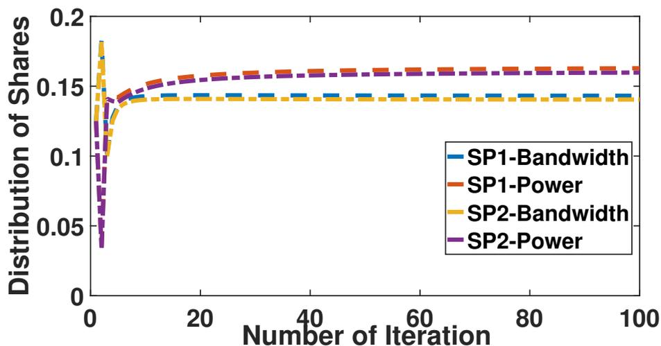
Figure 4.5 – Convergence of Algorithm 1 to the NE
