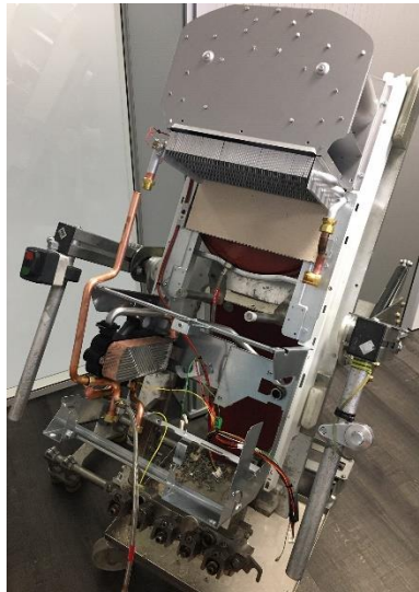
Figure 2-5. Field experiment: assembly of a boiler in progress.
