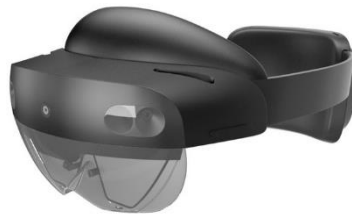
Figure 4-4. Microsoft HoloLens 2, a state-of-the-art AR see-through HMD.
