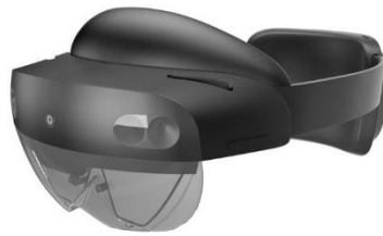
Figure 4-4. Microsoft HoloLens 2, a state-of-the-art AR see-through HMD.
