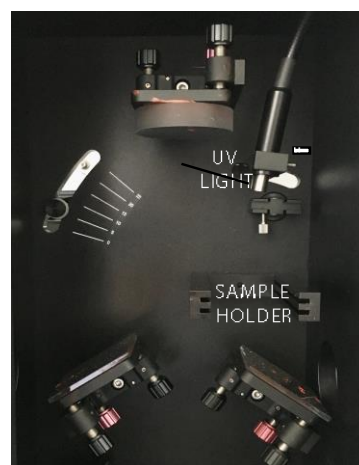
Figure-S II-2 Experimental set-up for real-time FTIR monitoring of photopolymerization
