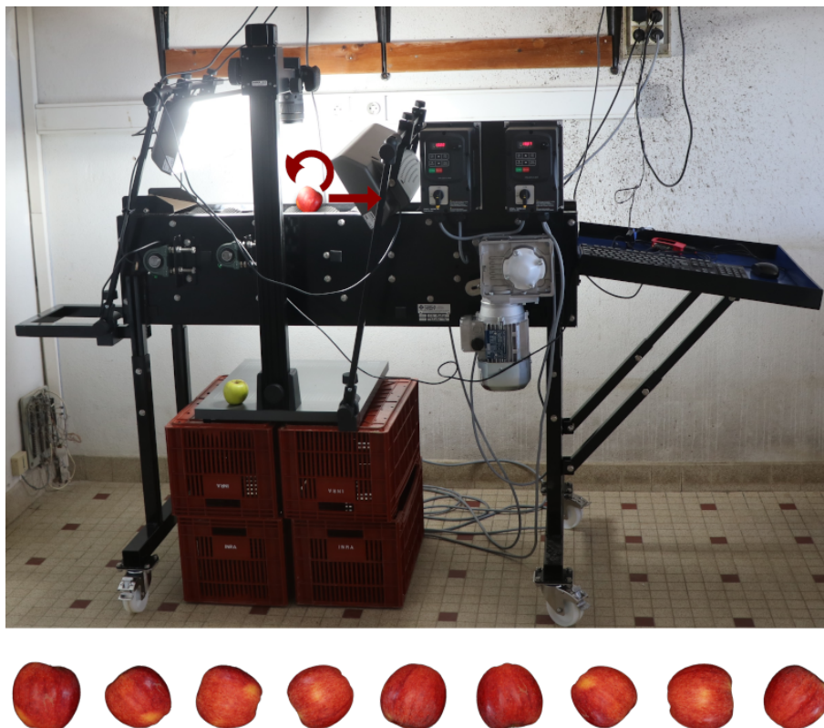
Figure 3.1 – Acquisition system. Upper panel: Machine equipped with a conveyor belt, used for the acquisition of images of apples with a high surface coverage. Lower panel: view of the acquired images of apples after segmentation from the background.
