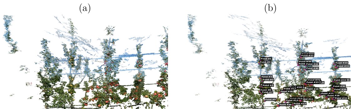
Figure 6.2 – (a): 3D point cloud of apple trees. (b): 3D point cloud of apple trees with ground truth apple locations.
