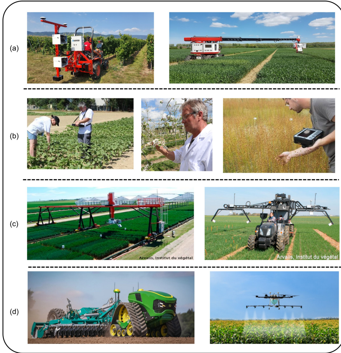
Figure 1.2 – (a): High-throughput phenotyping platform in plant breeding [1]. (b): Example of measurements conducted manually, in variety testing [2]. (c): Robots used by technical institutes. The illustrated one is called Phenoarch used in Arvalis technical institutes [3]. (d): Robots and drones used by farmers [4].
