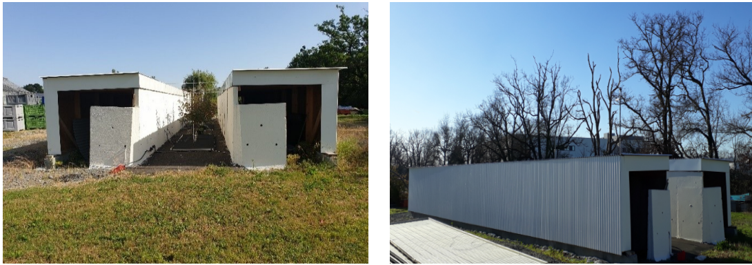
FIGURE 82 – Street canyon on 1/5 th scale built on Institut Agro site in Angers, France.
