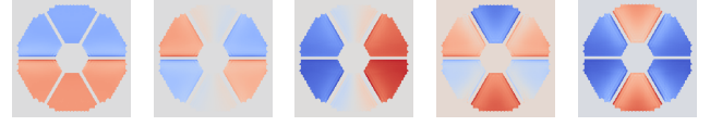
Fig. 2. Last eigenvectors of the interaction matrix: they are dominated by petal modes.
