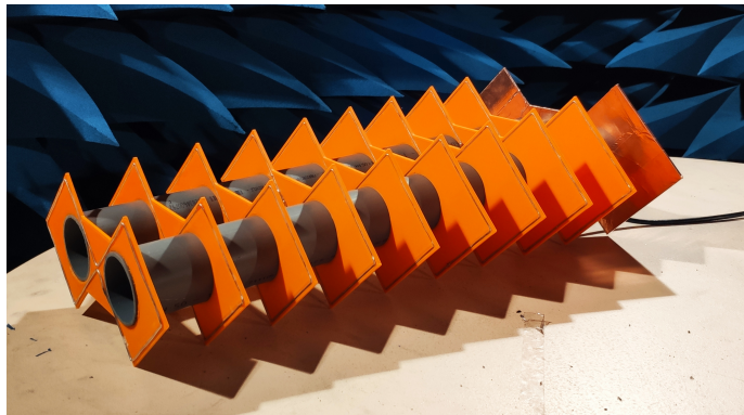
Figure 7-2 – 3D printed Yagi antenna at 770 MHz.
