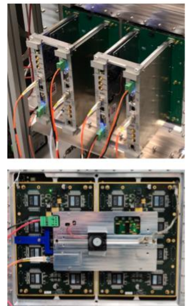
Figure 7.18: Photographs of the readout electronics used for T2K TPCs: the ARC cards, versatile card with AFTER chips (top), and the new design for the HA-TPCs using FEC cards synchronized by a FEM (bottom).
