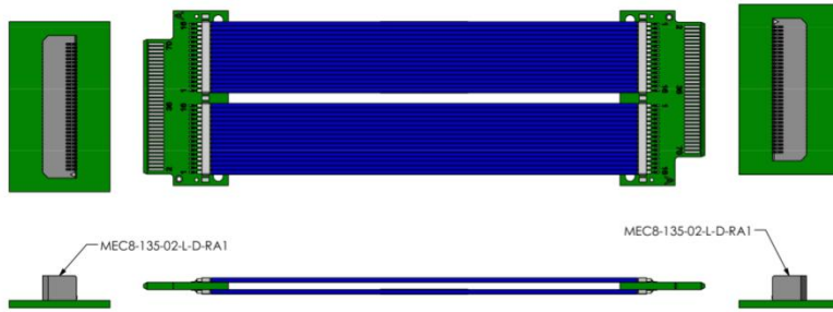
Figure 3.20: Specifically designed Samtec cable for detector to electronics connection. The MEC8 connectors can either be horizontal as illustrated or vertical.
