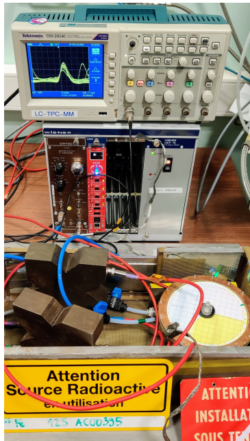
Figure 4.3: Experimental setup for the Micromegas readout plane characterization reading the micro-mesh signal.
