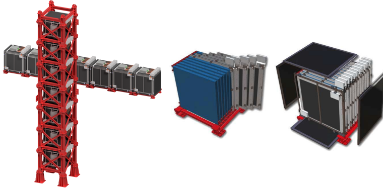
Figure 6.9: Left: Overview of the INGRID on-axis detector with its 14 modules arranged in a cross shape (2 additional off-axis modules are not represented here). Right: Exploded view of a single INGRID module: tracking planes are represented in blue and interleaved with iron plates, veto planes are the external planes shown in black.
