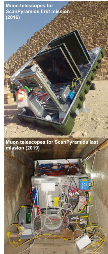
Figure 2.12: Comparison of CEA muon telescopes design between the first and last ScanPyramids mission.
