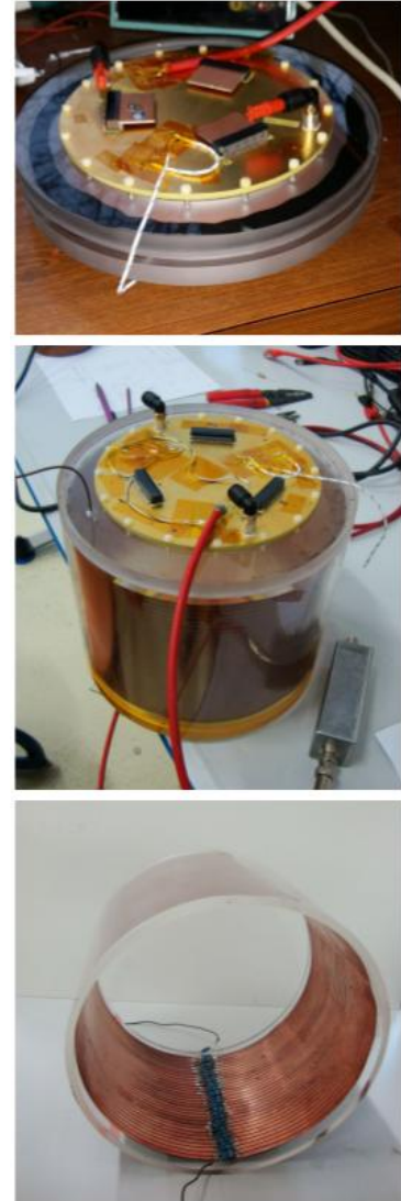
Figure 3.29: Photographs of the preliminary prototypes developed during my first year of PhD: 3 cm drift space P1 (top), 22 cm drift space P2 (middle) with copper strips field cage (bottom).
