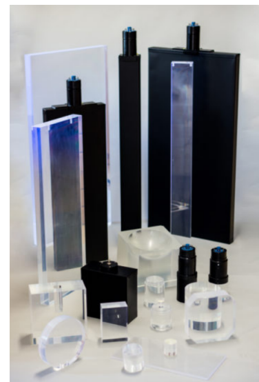
Figure 3.22: Examples of possible plastic scintillator shapes available from the supplier.
