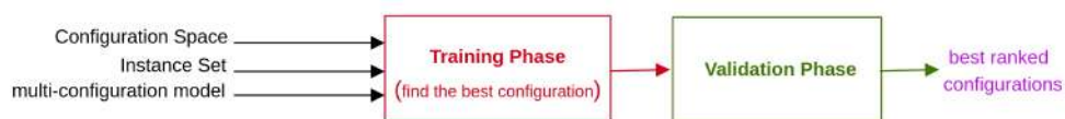
Figure 2.18: The automated design system component and the arrows define the information flow
