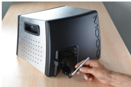
(e) Desktop Haptic Interface from MOOG, Inc., U.S.A.[31]
