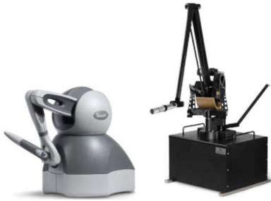
(a) Touch and Phantom Premium 3.0 from 3D Systems, U.S.A.[1]
