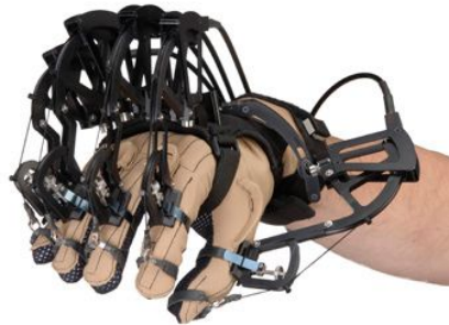
Figure 1.11 – Force feedback interface by Cyber glove [30].
