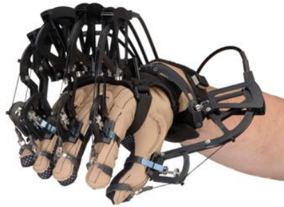
Figure 1.11 – Force feedback interface by Cyber glove [30].
