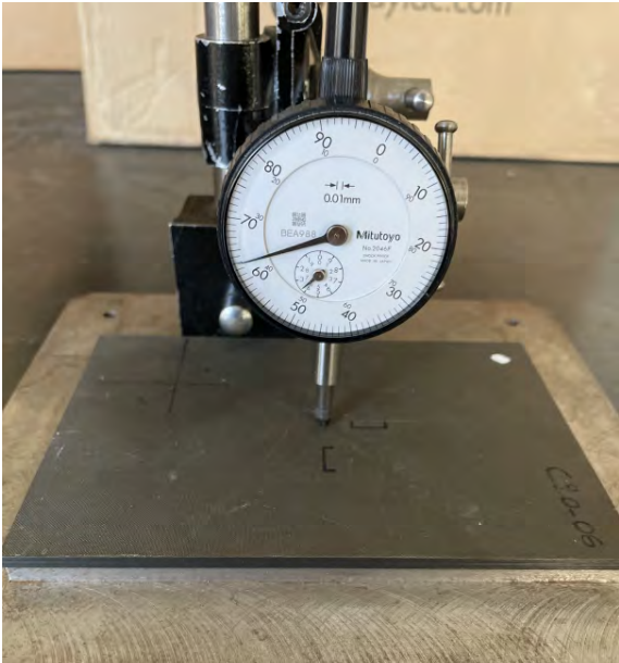
Figure 2.9: Mechanical comparator used for the measurement of the residual dent
