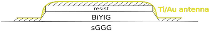
Figure 3.12: Profile view of a disk B under the antenna showing the contact between the edges of the disk and the Ti/Au antenna at the lateral boundaries.
