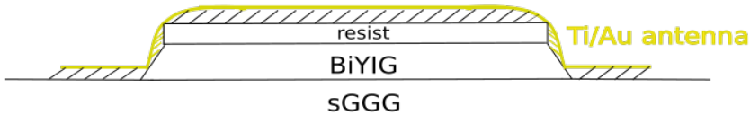
Figure 3.12: Profile view of a disk B under the antenna showing the contact between the edges of the disk and the Ti/Au antenna at the lateral boundaries.
