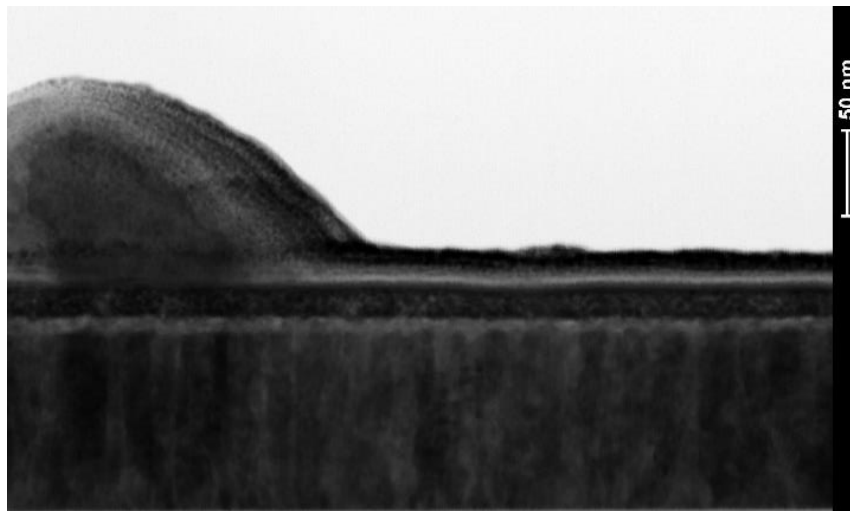
Figure 129 Cross sectional TEM image of TiN/HZO/TiN stack with 100/15/100 nm
