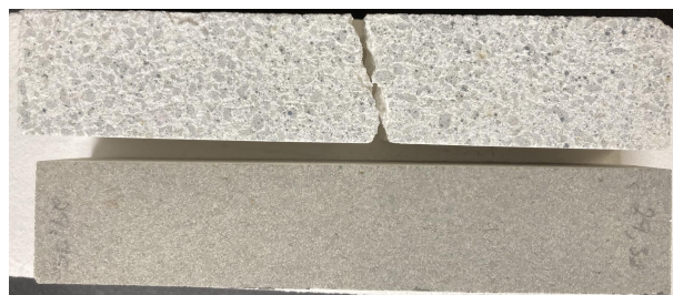
Figure IV.19: Four-point bending: Sample before (below) and after (above) a test that took three days.
