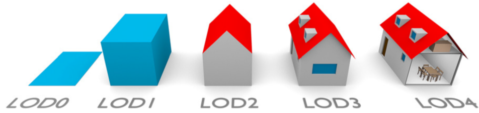
Figure 1.4: The five LODs of CityGML 2.0. From LOD0 to LOD4, the virtual models are more and more precise. They are employed in various application contexts. Image taken from [BLS16]
