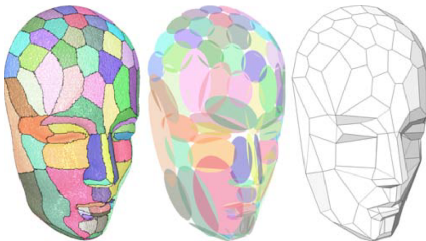
Figure 2.5: Dense mesh partitioning and approximation. The input dense mesh is divided by error-driven partitioning (left). And a planar proxy is extracted for each cluster (middle). The proxies are then used to generate an approximated compact mesh (right). Image sourced from [CSAD04].
