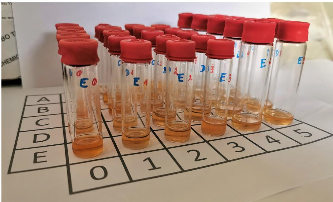
Figure 4.1: A photograph of 30 samples assembled and measured under the controlled, dry atmosphere of argon. The number from 0 to 5 represent the percentage (vol.) of water added to the DMF solution. The letters from A to E represent the amount of dissolved bismuth (III) disalicylate per 2.5 ml of DMF, starting from 10, 20... up to 50 mg.
