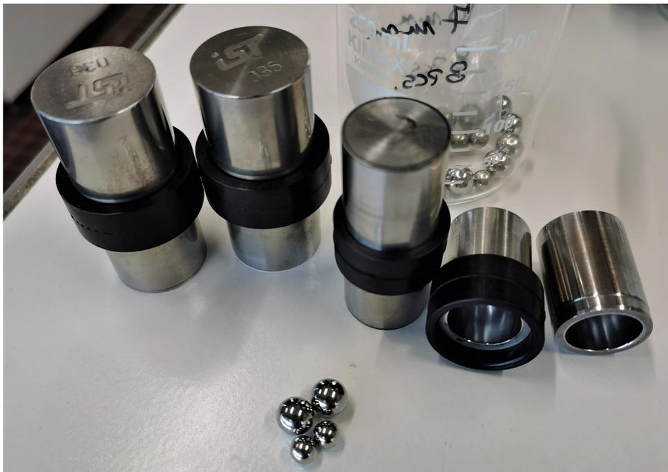
Figure 2.2: A photograph of the milling jars and the stainless steel balls used in the project. During the synthesis, the reaction mixture is placed inside one half of the jar, and followed by the milling balls. Then, the jar is sealed with the other half and the rubber seal. The assembled jars are placed vertically in between the clamps of the mill, before the milling starts.
