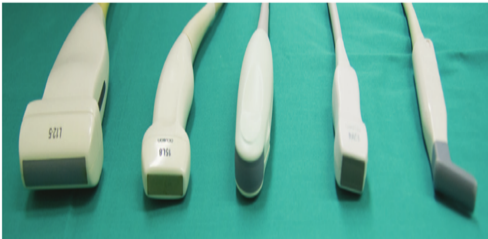
Figure 1.4: US transducers for regional anesthesia. The photograph includes (left to right) broad linear, small footprint linear, curved, sector, and hockey-stick transducers [25].
